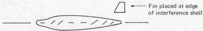
Fuselage is a body of revolution plus camber slopes defined along straight aerodynamic mean centerline.
