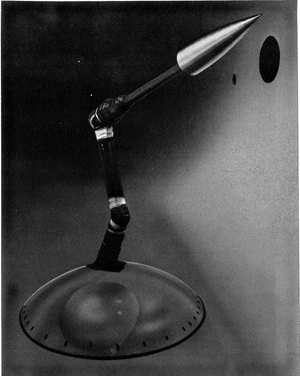
(c) Installation of tangent ogive on floor support system, \alpha = 0^\circ to 45^\circ .
