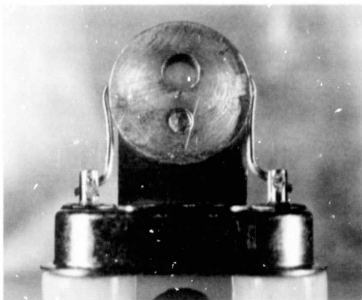
x4 Fig. 4. View looking in the primary beam direction of a specimen holder used to mount lunar fines for AES/SEM.
