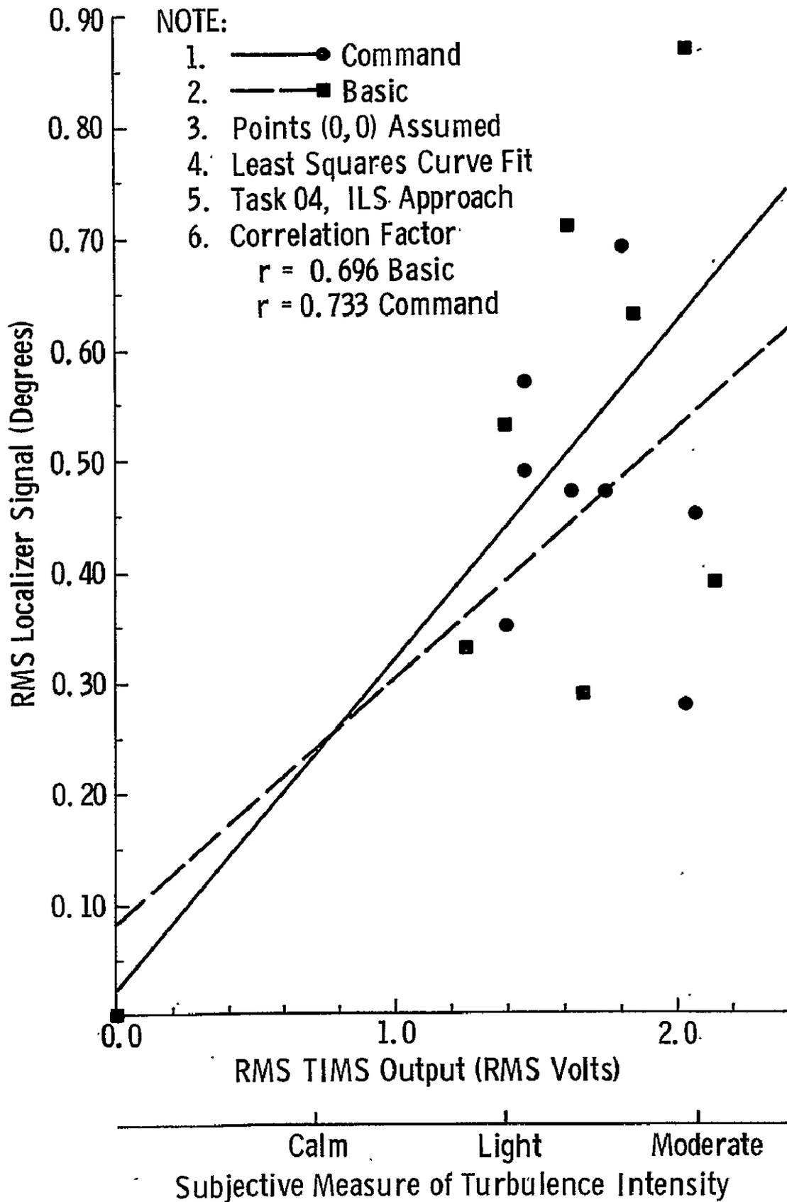
FIGURE 9.12 Least Squares Curve Fit to the RMS Localizer Signal as a Function of RMS TIMS Output
