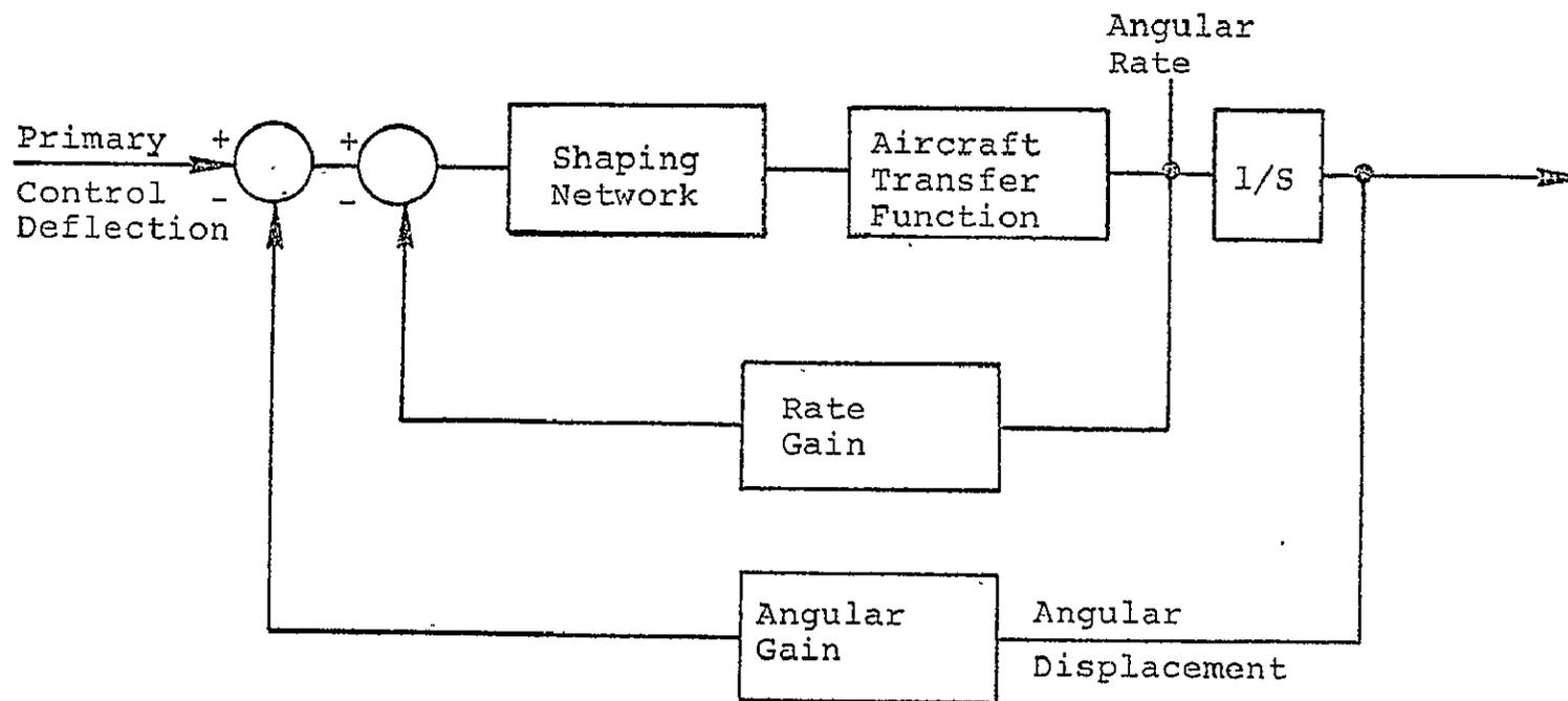
FIGURE 3.5 Simplified Block Diagram of Attitude Command Control System
