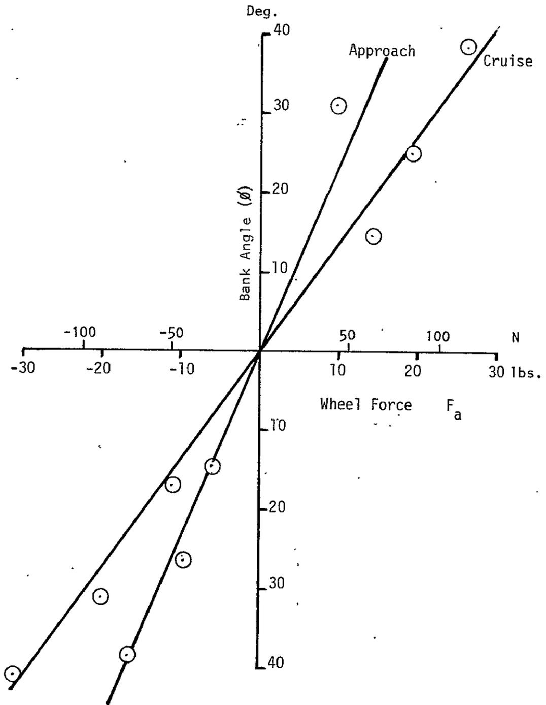
FIGURE 7.2 SSSA Model 99 Aileron Control Forces
