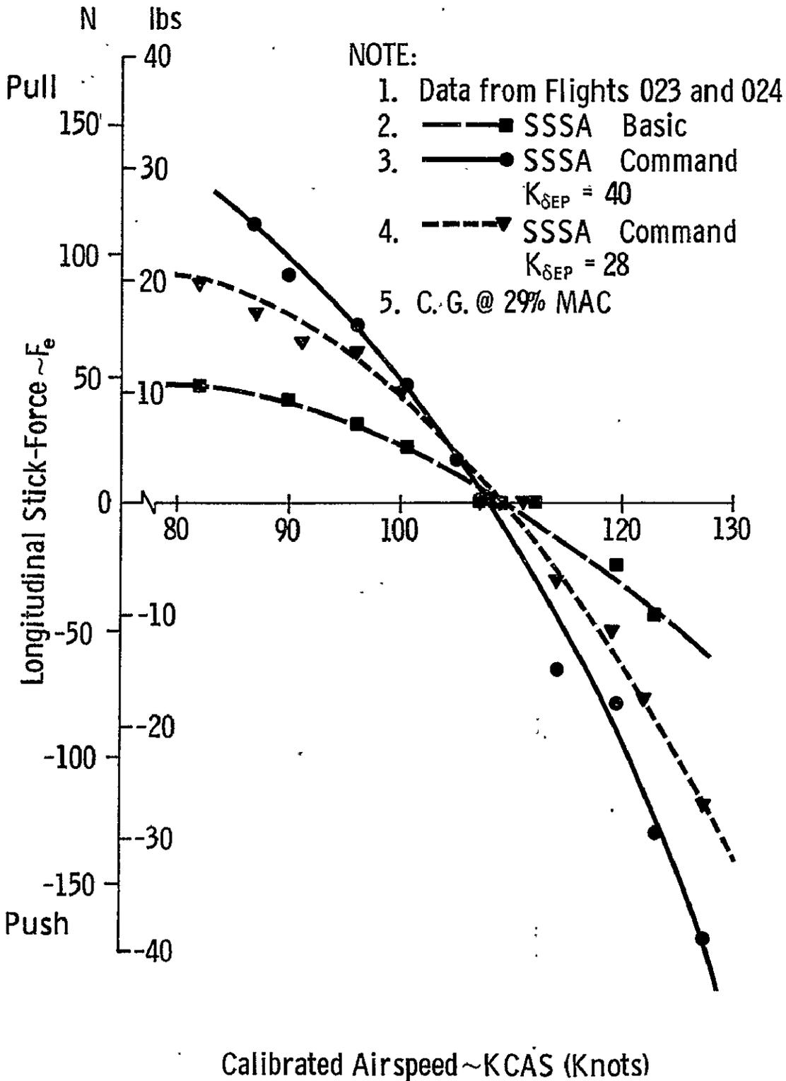
FIGURE 8.7 SSSA Model 99 Static Longitudinal Stability, as a Function of  $K_{\delta EP}$  in the Approach Configuration
