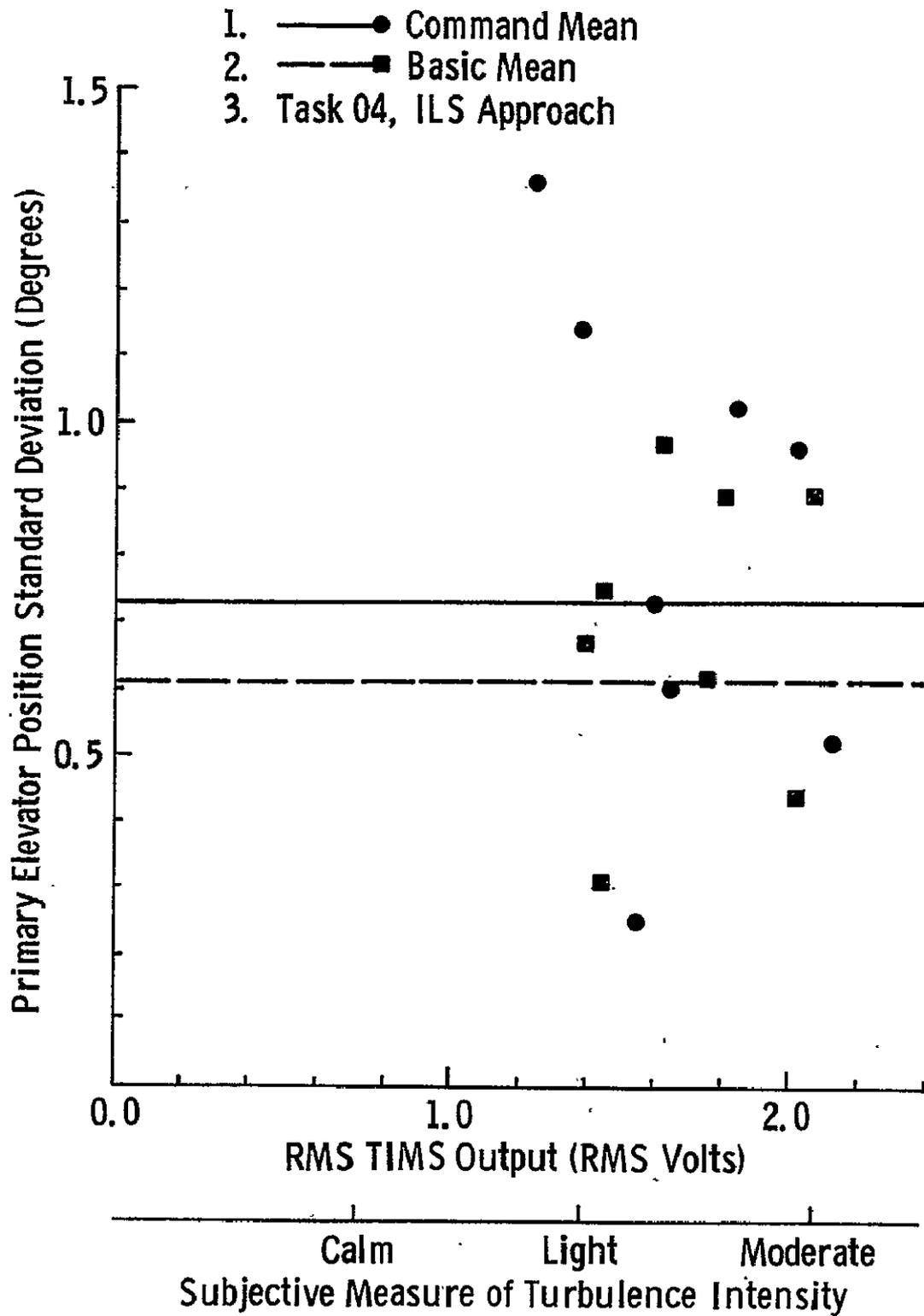
FIGURE 9.21 Average Standard Deviation of Primary Elevator Position as a Function of RMS TMS Output for the ILS Approach
