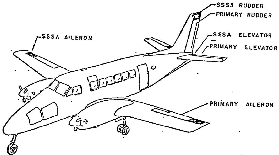
FIGURE 3.1. General Arrangement of the SSSA Surface
