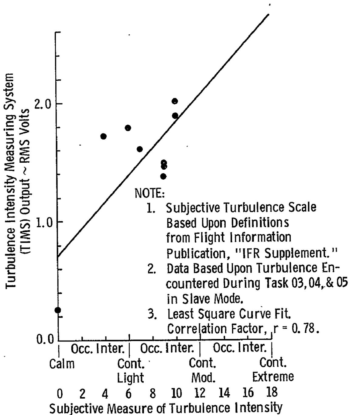
FIGURE 9.1 Relationship of the Pilots' Subjective Measure of Turbulence to the TIMS Output
