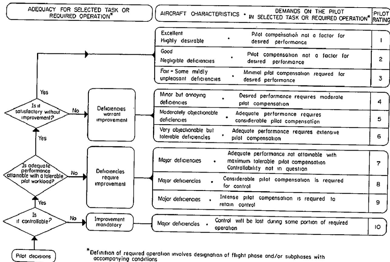
FIGURE 5.3 Cooper-Harper Handling Qualities Rating Scale
