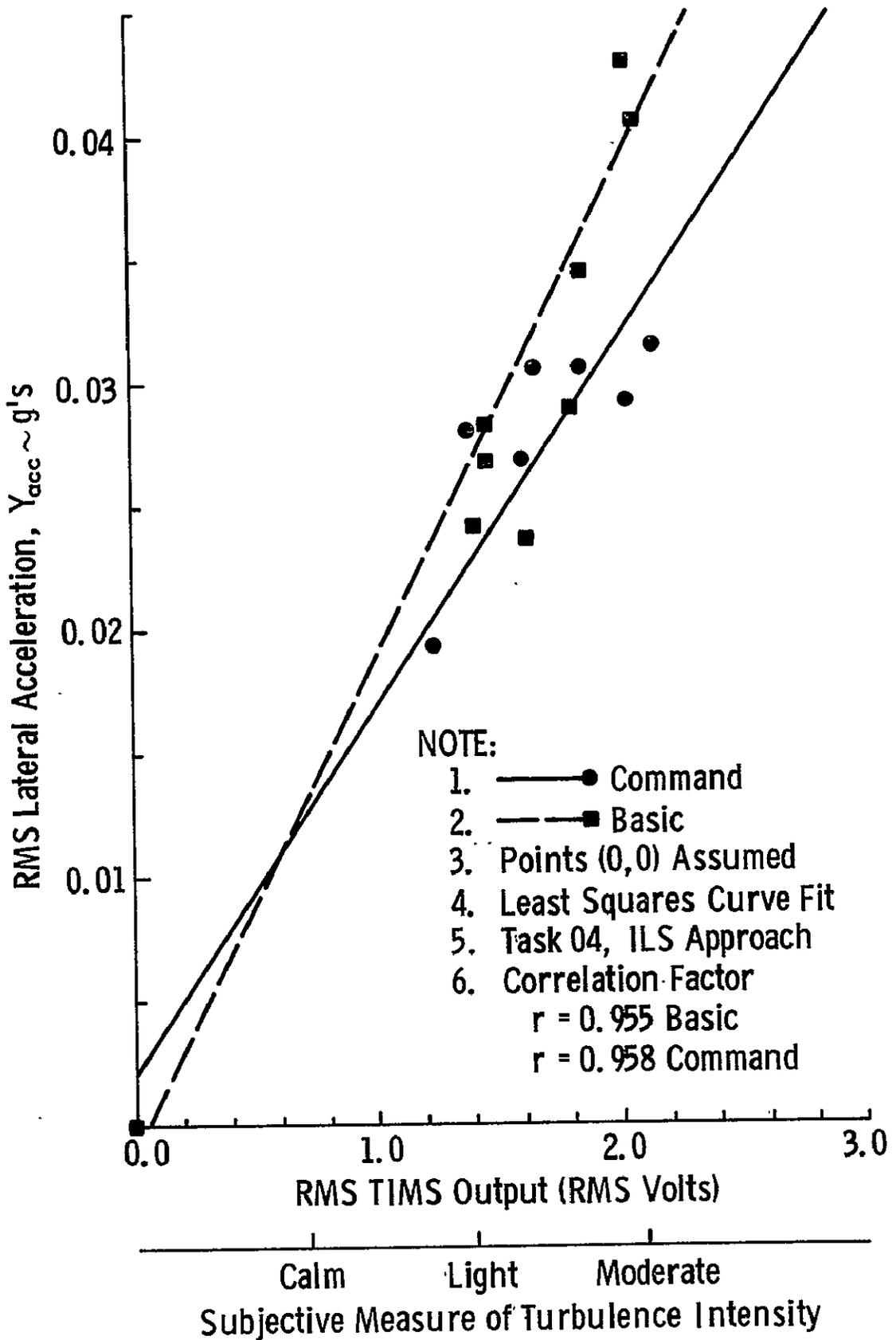
FIGURE 9.31 Least Squares Curve Fit to the RMS Lateral Acceleration as a Function of RMS TMS Output for the ILS Approach
