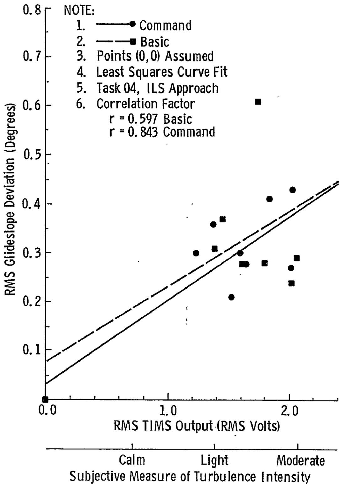
FIGURE 9.13 Least Squares Curves Fit to the RMS Glideslope Signal as a Function of RMS TIMS Output
