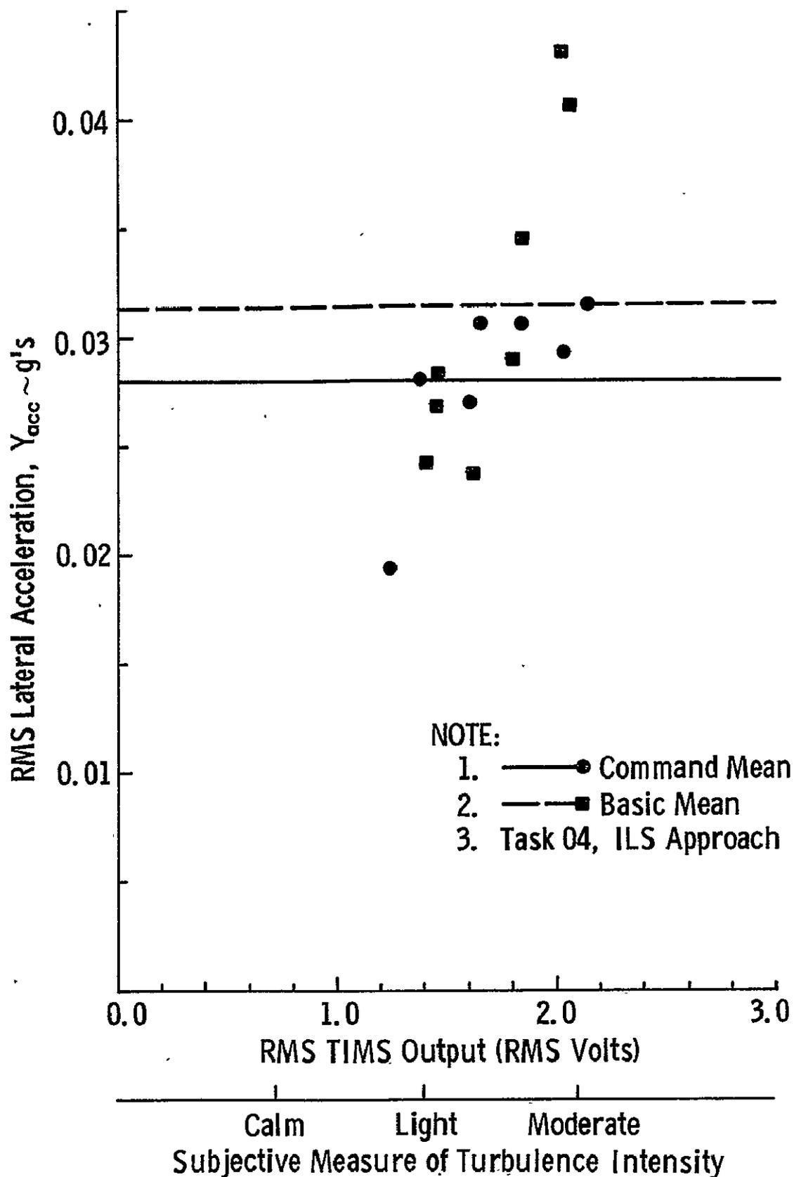
FIGURE 9.30 Average RMS Lateral Acceleration as a Function of RMS TMS Output for the ILS Approach
