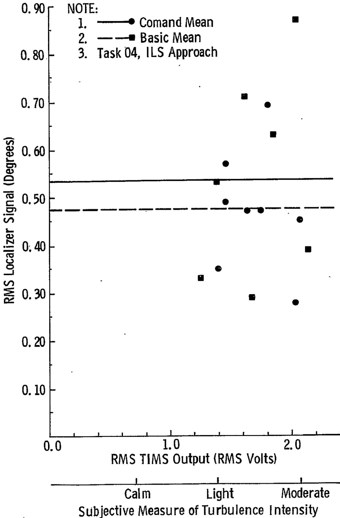
FIGURE 9.10 Average RMS Localizer Signal as a Function of RMS TIMS Output
