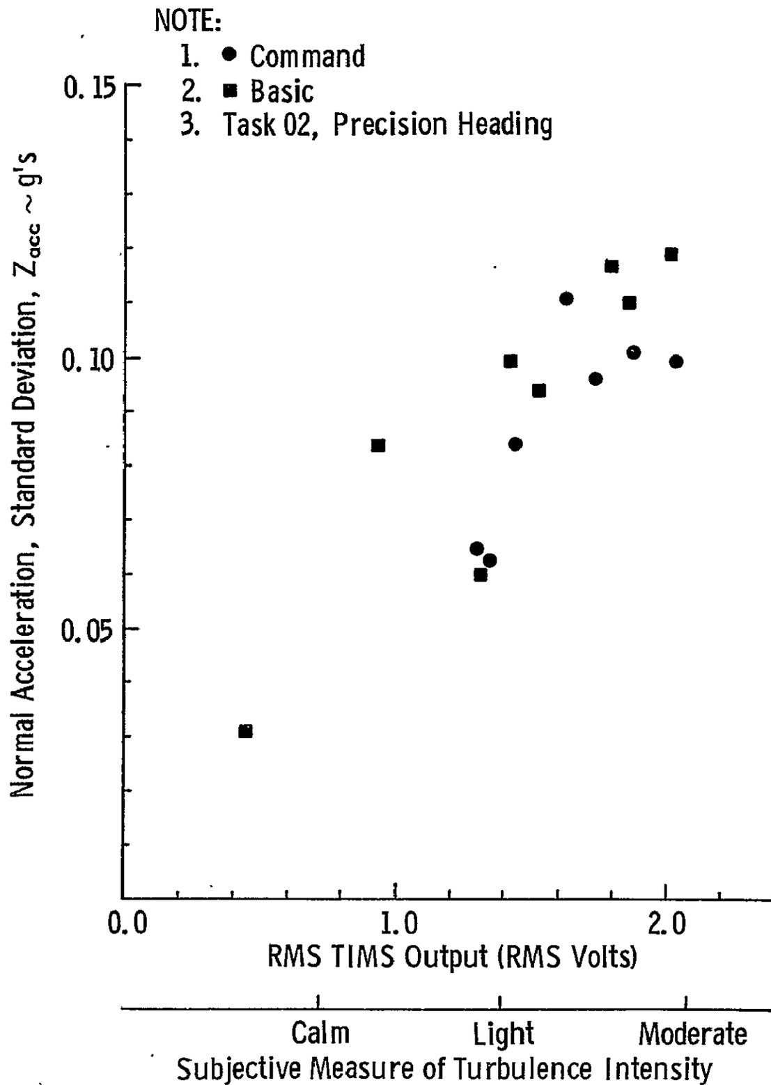
FIGURE 9.23 Standard Deviation of Normal Acceleration as a Function of RMS TIMS Output for the Precision Heading Task
