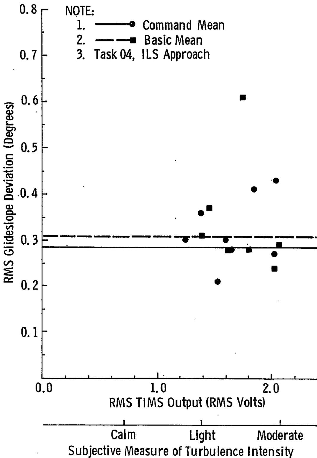
FIGURE 9.11 Average RMS Glideslope Signal as a Function of RMS TMS Output
