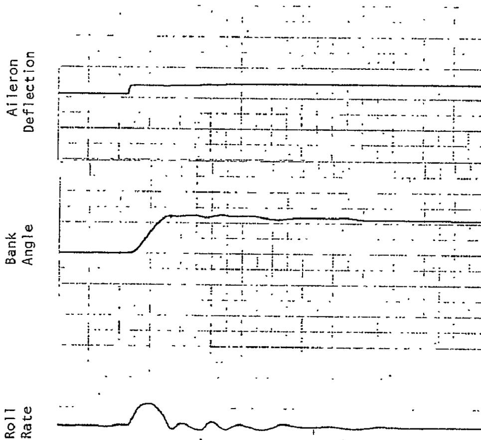
FIGURE 2.2 Attitude Command Roll Response Due to Step Aileron Input
