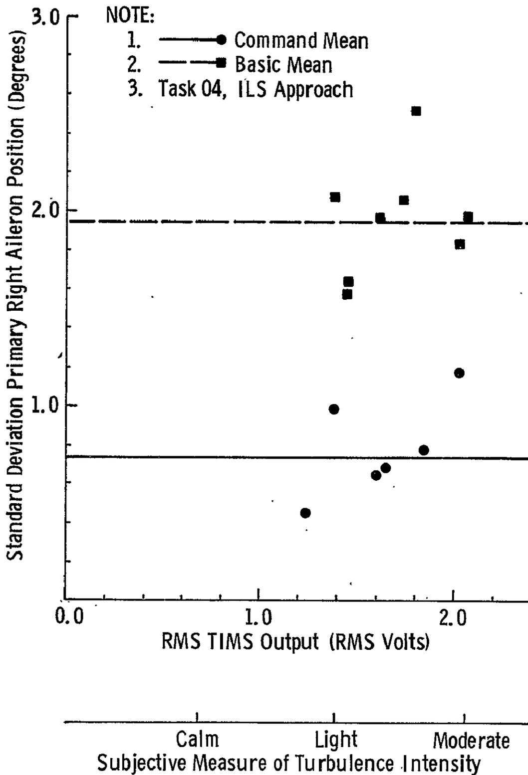
FIGURE 9.18 Average Standard Deviation of Primary Right Aileron Position as a Function of RMS TIMS Output for the ILS Approach
