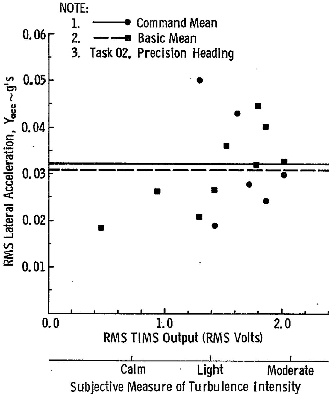
FIGURE 9.27 Average RMS Lateral Acceleration as a Function of RMS TMS Output for the Precision Heading Task
