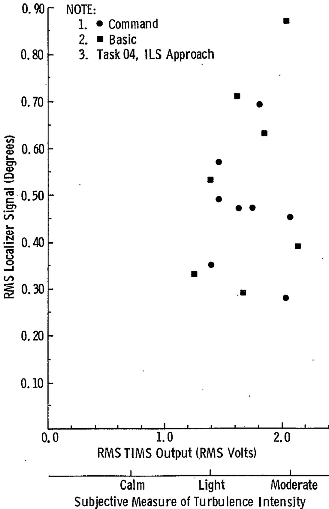
FIGURE 9.8 RMS Localizer Signal as a Function of RMS TIMS Output
