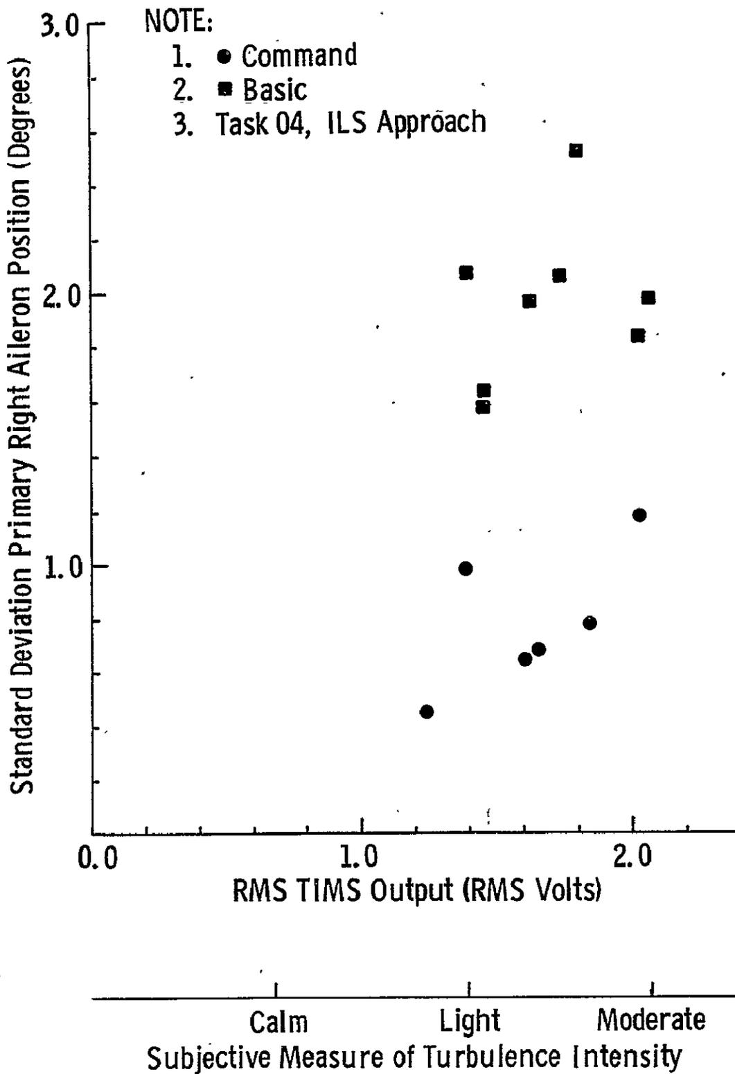
FIGURE 9.17 Standard Deviation of Primary Right Aileron Position as a Function of RMS TMS Output for the ILS Approach
