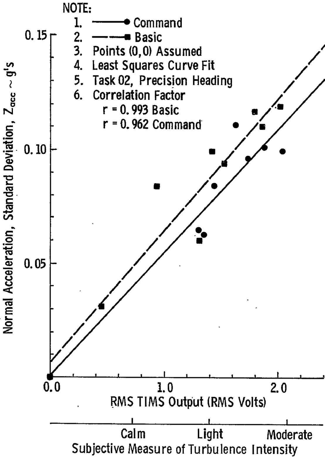
FIGURE 9.25 Least Squares Curve Fit to the Standard Deviation of Normal Acceleration as a Function of RMS TIMS Output for the Precision Heading Task
