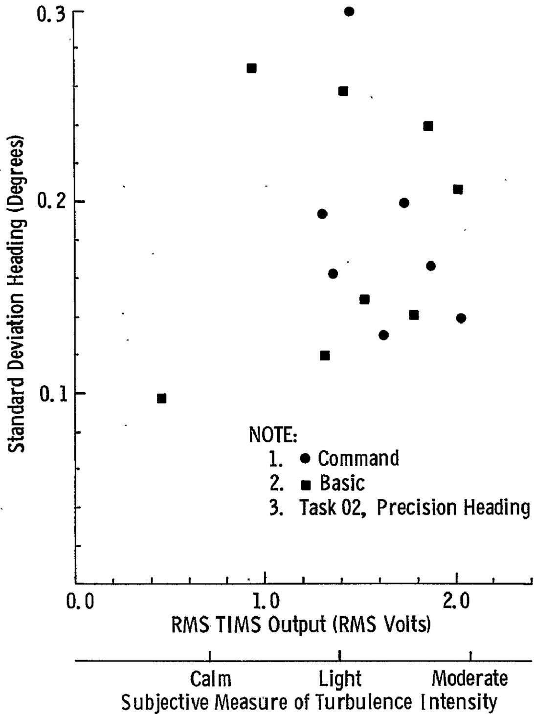
FIGURE 9.5 Standard Deviation of SSSA Model 99 Heading as a Function of RMS TIMS Output for the Precision Heading Task
