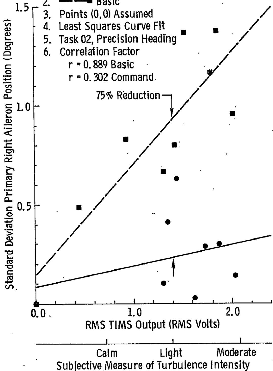
FIGURE 9.16 Least Squares Curve Fit to the Standard Deviation of Primary Right Aileron Position as a Function of RMS TIMS Output for the Precision Heading Task
