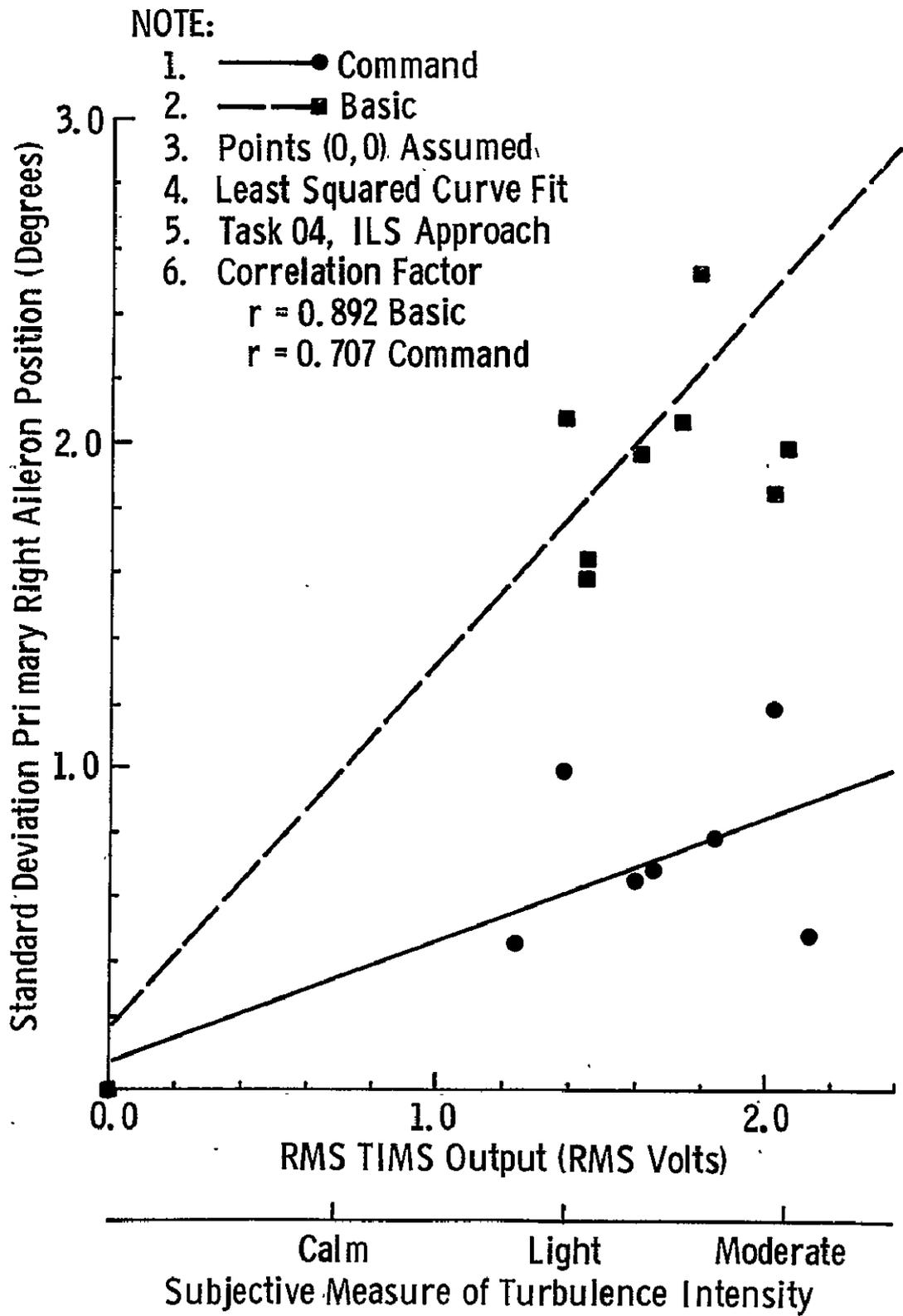
FIGURE 9.19 Least Squares Curve Fit to the Standard Deviation of Primary Right Aileron Position as a Function of RMS TMS Output for the ILS Approach
