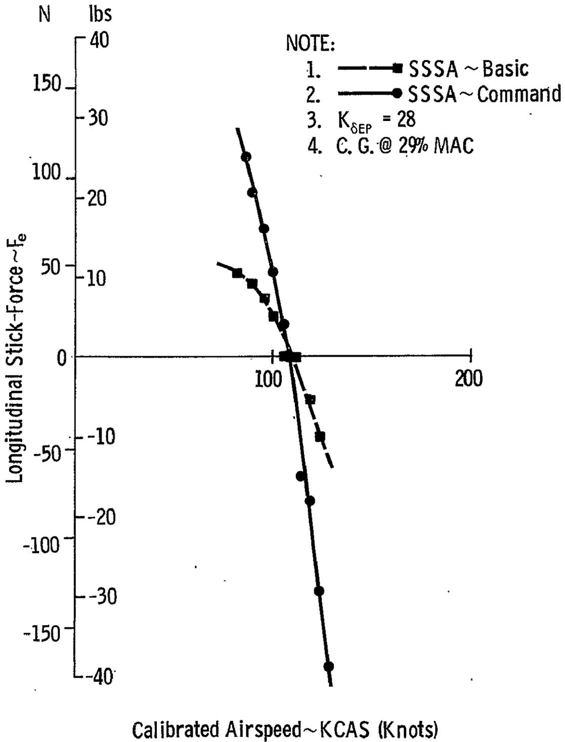
FIGURE 8.5 SSSA Model 99 Static Longitudinal Stability in the Approach Configuration
