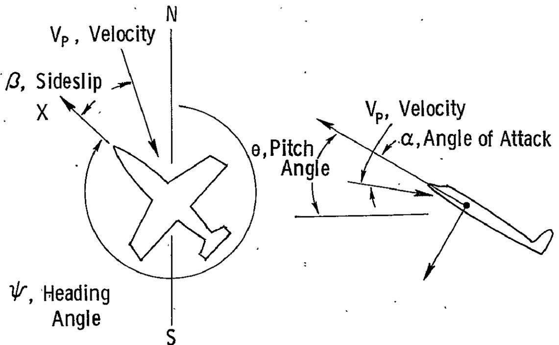
FIGURE 2.5 Angle of Sideslip and Attack Description
