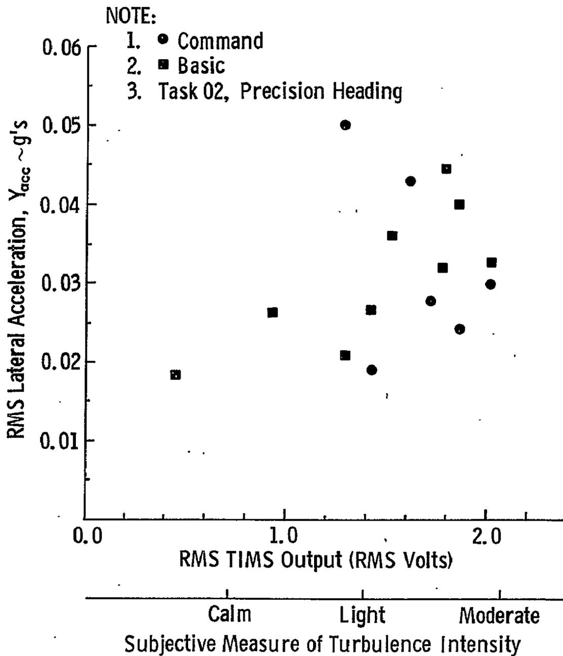
FIGURE 9.26 RMS Lateral Acceleration as a Function of RMS TIMS Output for the Precision Heading Task
