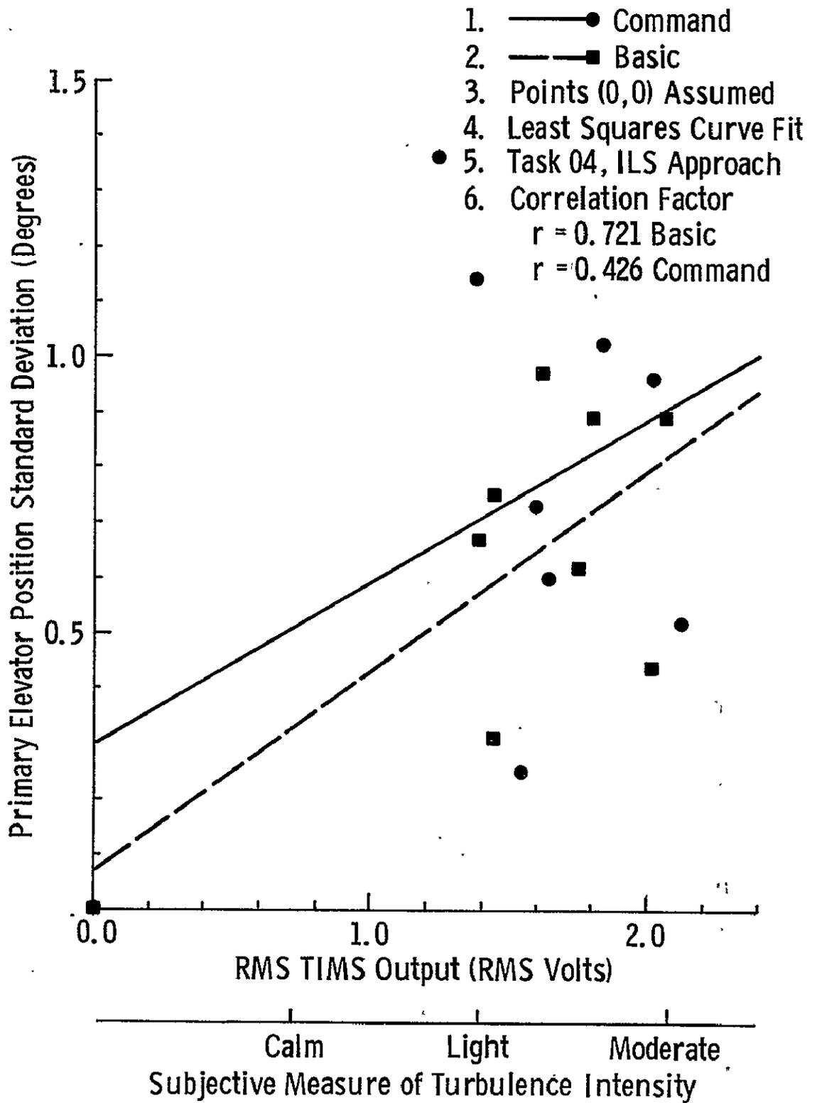
FIGURE 9.22 Least Squares Curve Fit to the Standard Deviation of Primary Elevator Position as a Function of RMS TIMS Output for the ILS Approach
