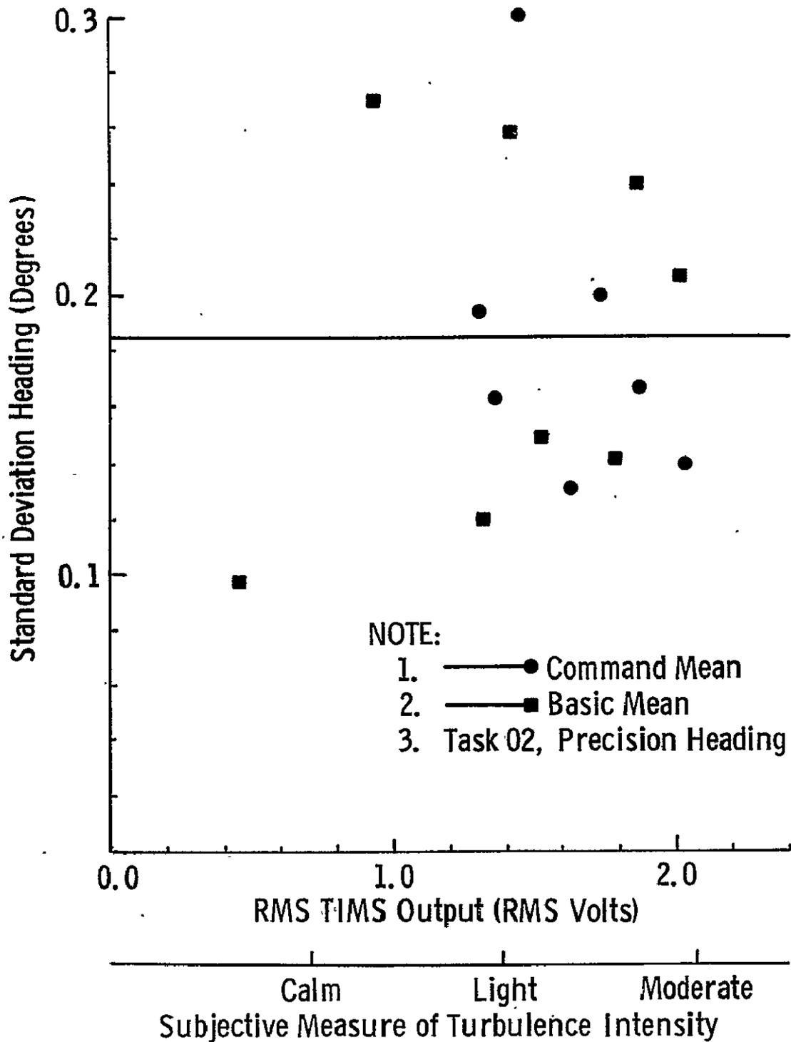
FIGURE 9.6 Average Standard Deviation of SSSA Model 99 Heading as a Function of RMS TMS Output for the Precision Heading Task
