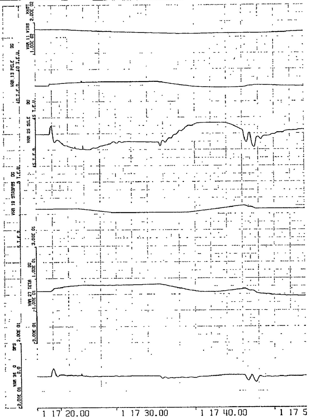
FIGURE 8.4 SSSA Model 99 (Command Mode) Pitch Response Due to a Step Elevator Input
