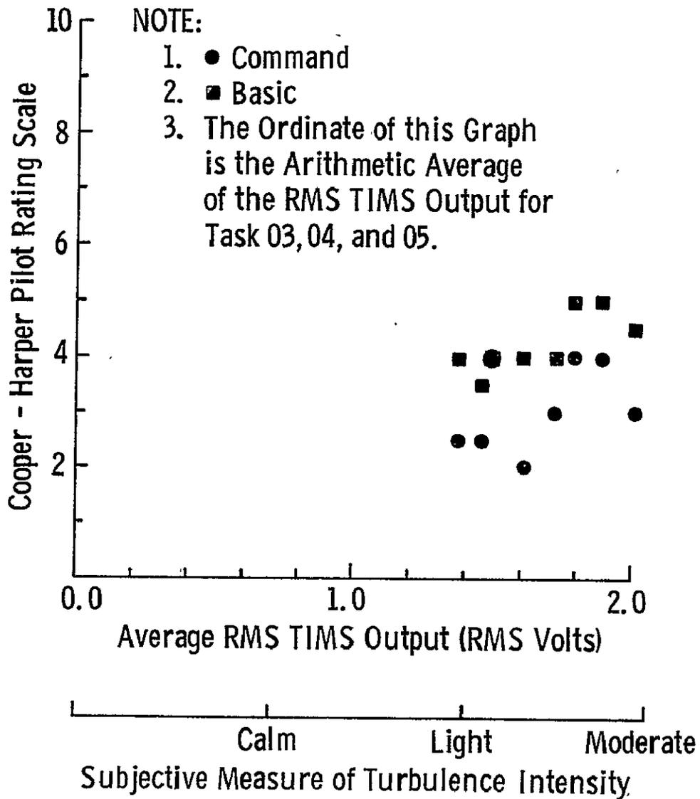
FIGURE 9.2 Cooper-Harper Pilot Rating as a Function of Average RMS TIMS Output
