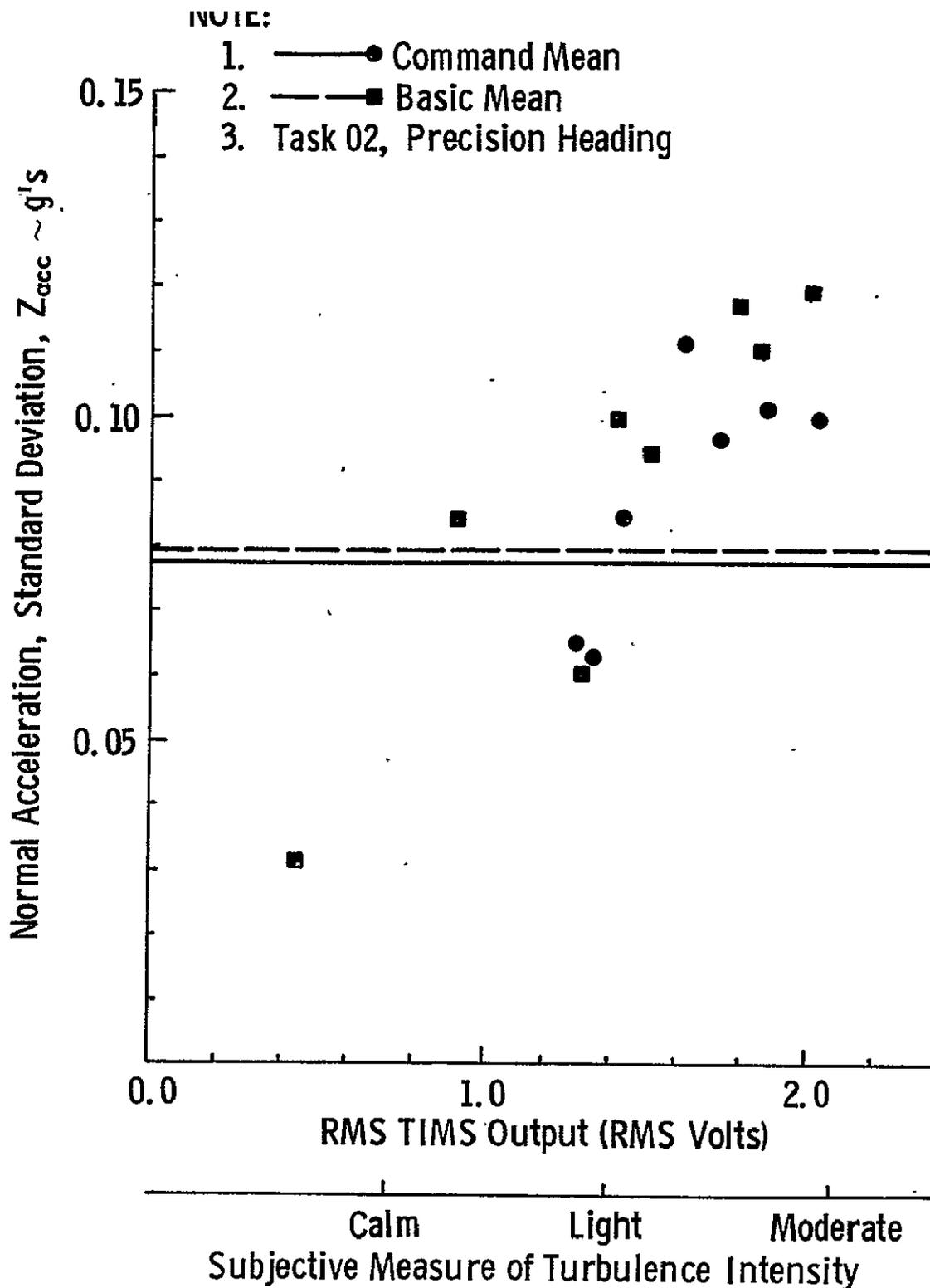
FIGURE 9.24 Average Standard Deviation of Normal Acceleration as a Function of RMS TIMS Output for the Precision Heading Task
