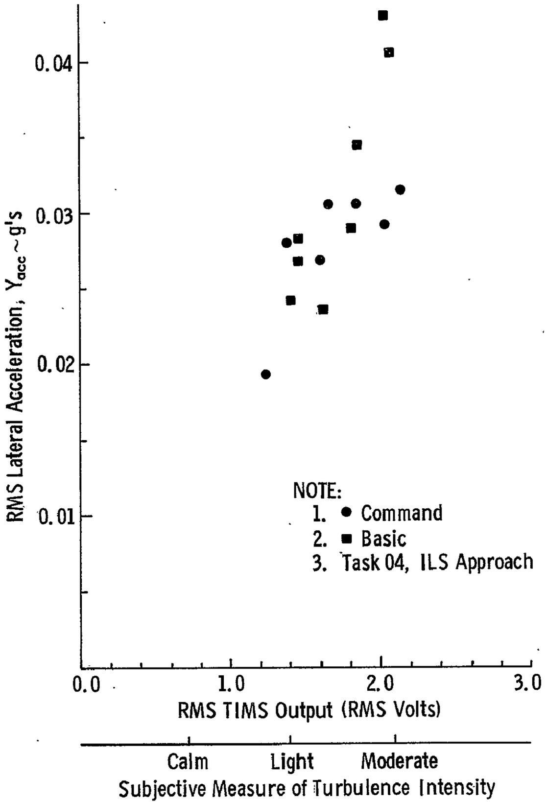
FIGURE 9.29 RMS Lateral Acceleration as a Function of RMS TIMS Output for the ILS Approach
