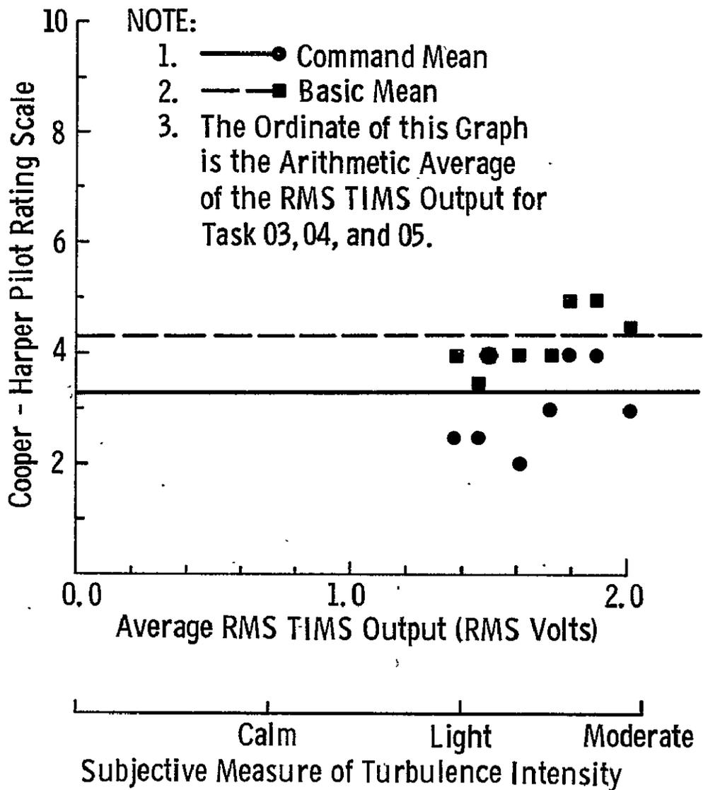
FIGURE 9.3 Average Cooper-Harper Pilot Rating as a Function of Average RMS TIMS Output
