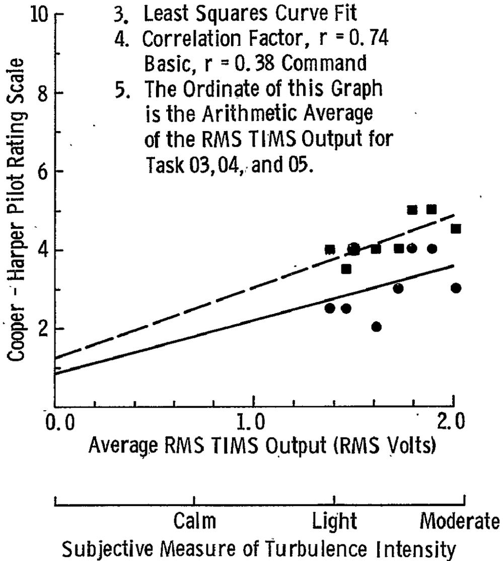
FIGURE 9.4 Least Squares Curve Fit to the Cooper-Harper Pilot Rating Scale as a Function of RMS TIMS Output
