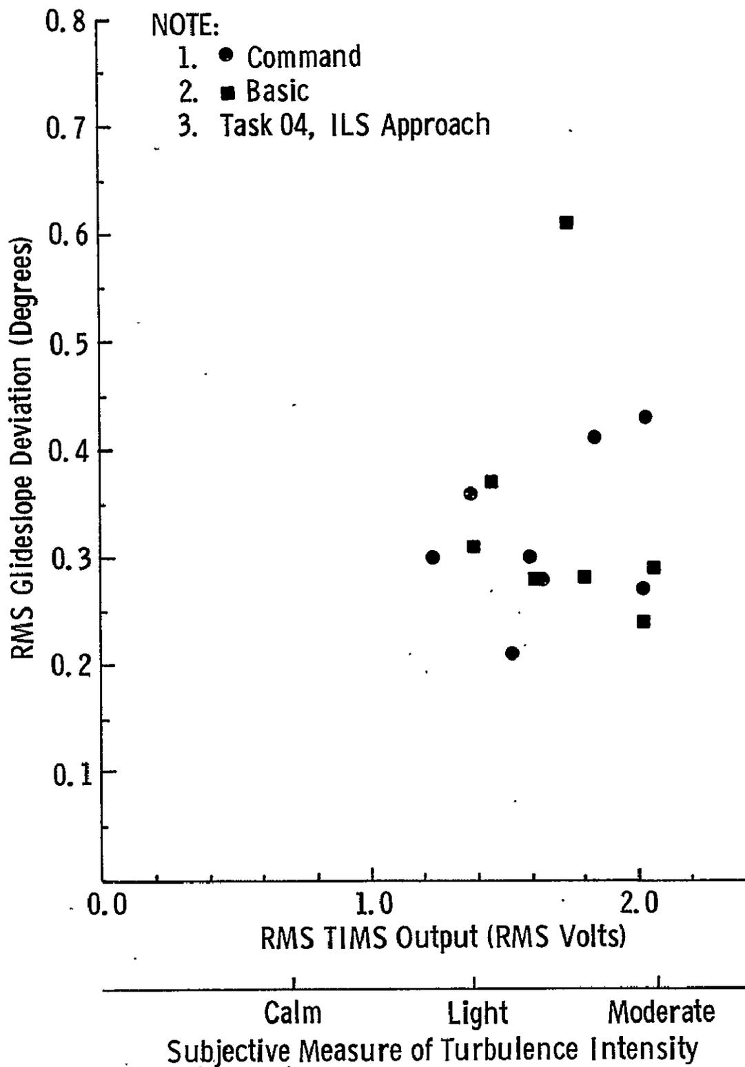
FIGURE 9.9 RMS Glideslope Signal as a Function of RMS TIMS Output
