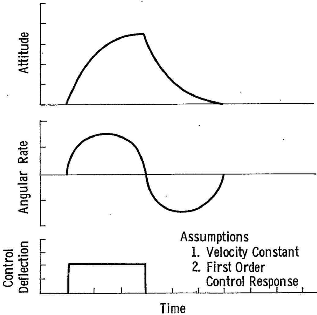
FIGURE 2.3 Conventional Aircraft Control Response About Pitch and Yaw Axes
