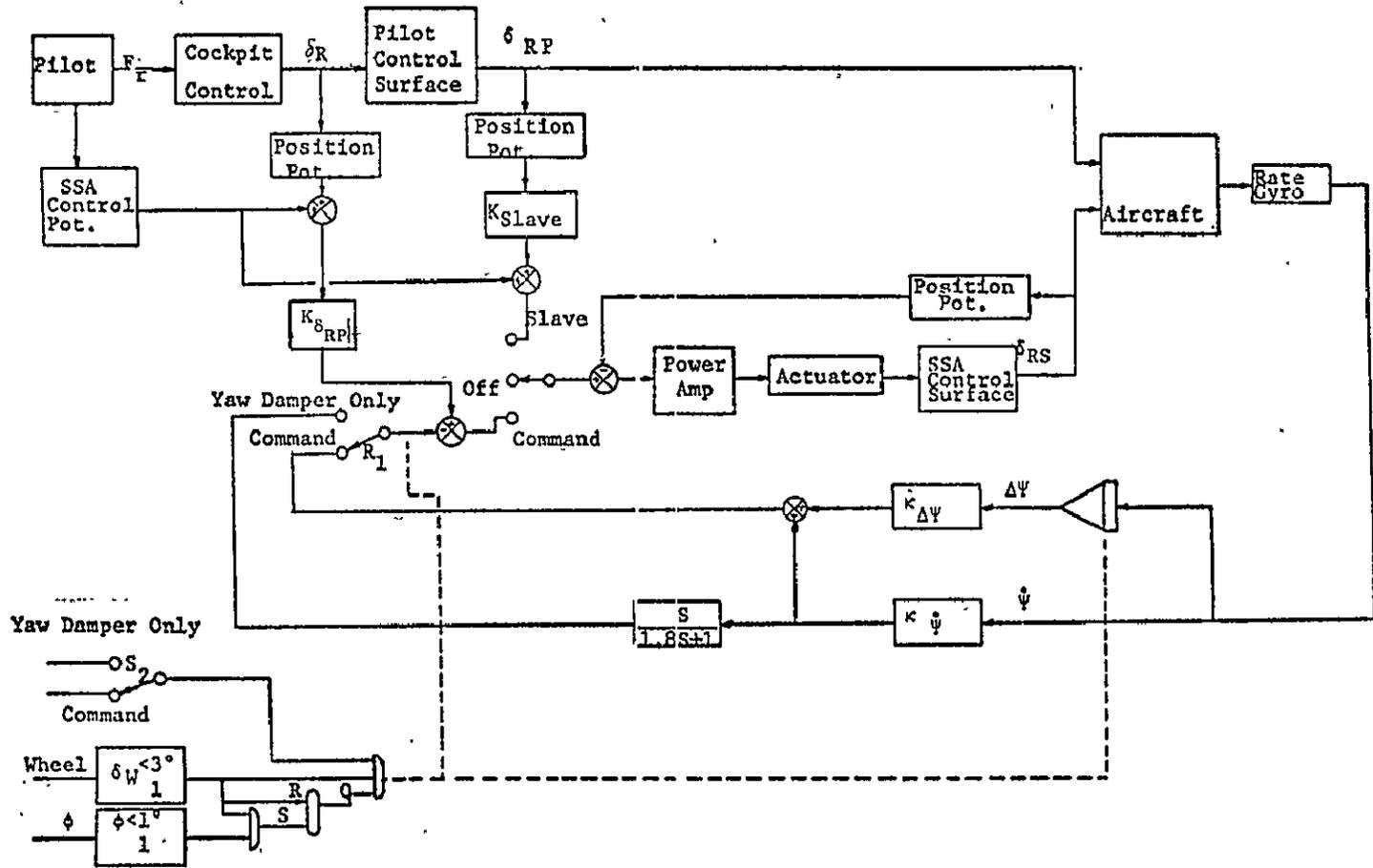
FIGURE 3.4 Block Diagram - Yaw Axis
