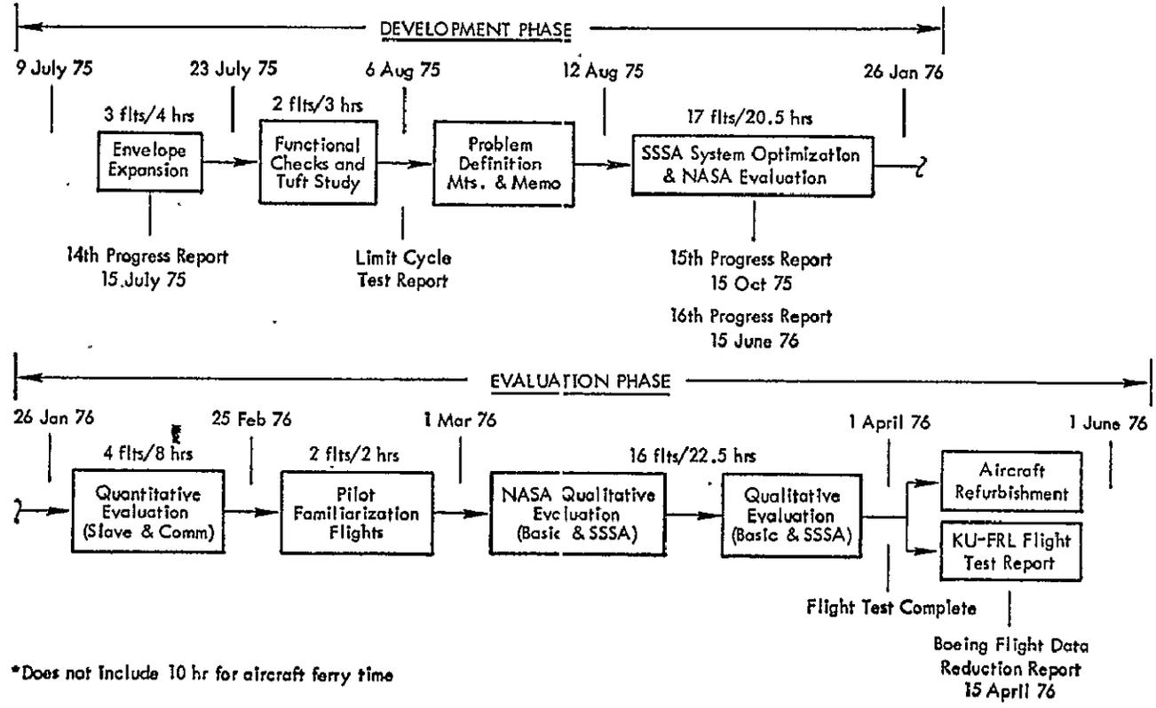
FIGURE 5.1 Proposed SSSA Model 99 Flight Test Schedule
