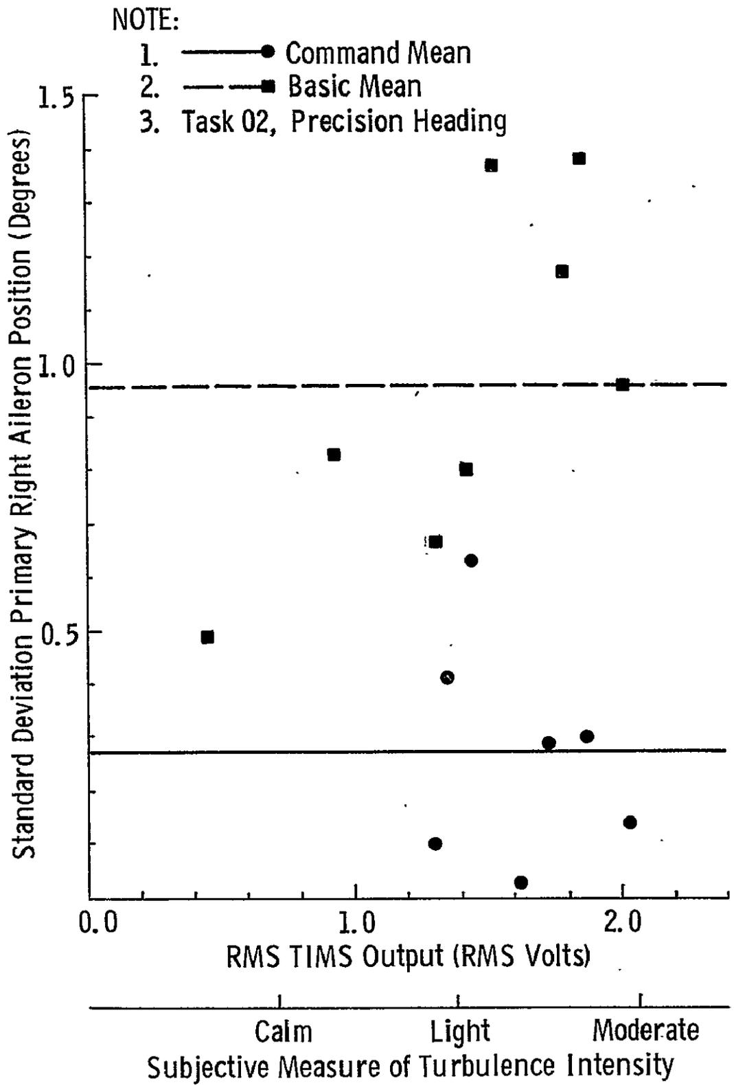
FIGURE 9.15 Average Standard Deviation of Primary Right Aileron Position as a Function of RMS TIMS Output for the Precision Heading Task
