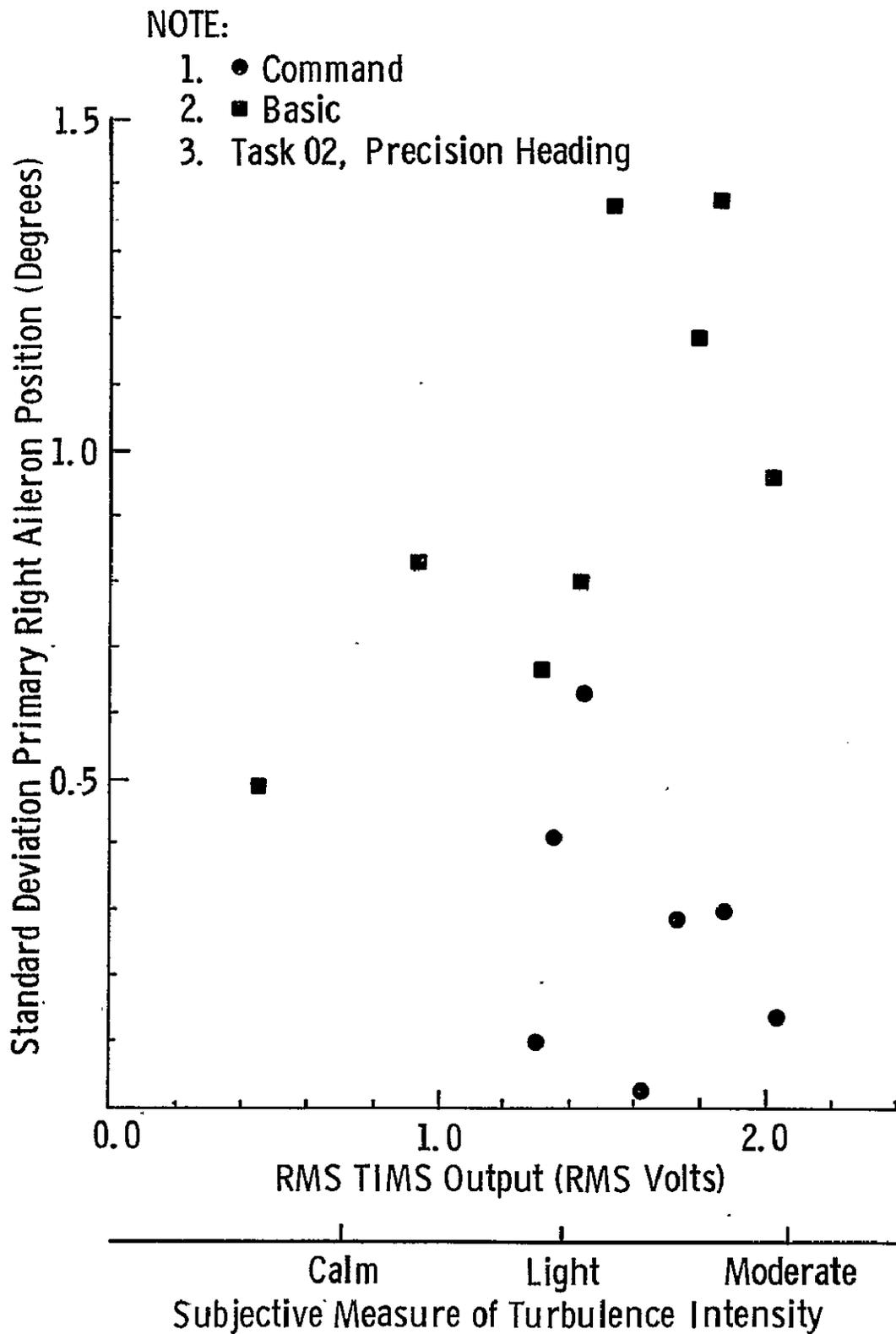
FIGURE 9.14 Standard Deviation of Primary Right Aileron Position as a Function of RMS TMS Output for the Precision Heading Task
