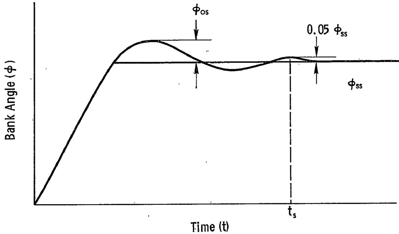
FIGURE 7.1 Definition of Bank Angle Overshoot and Settling Time
