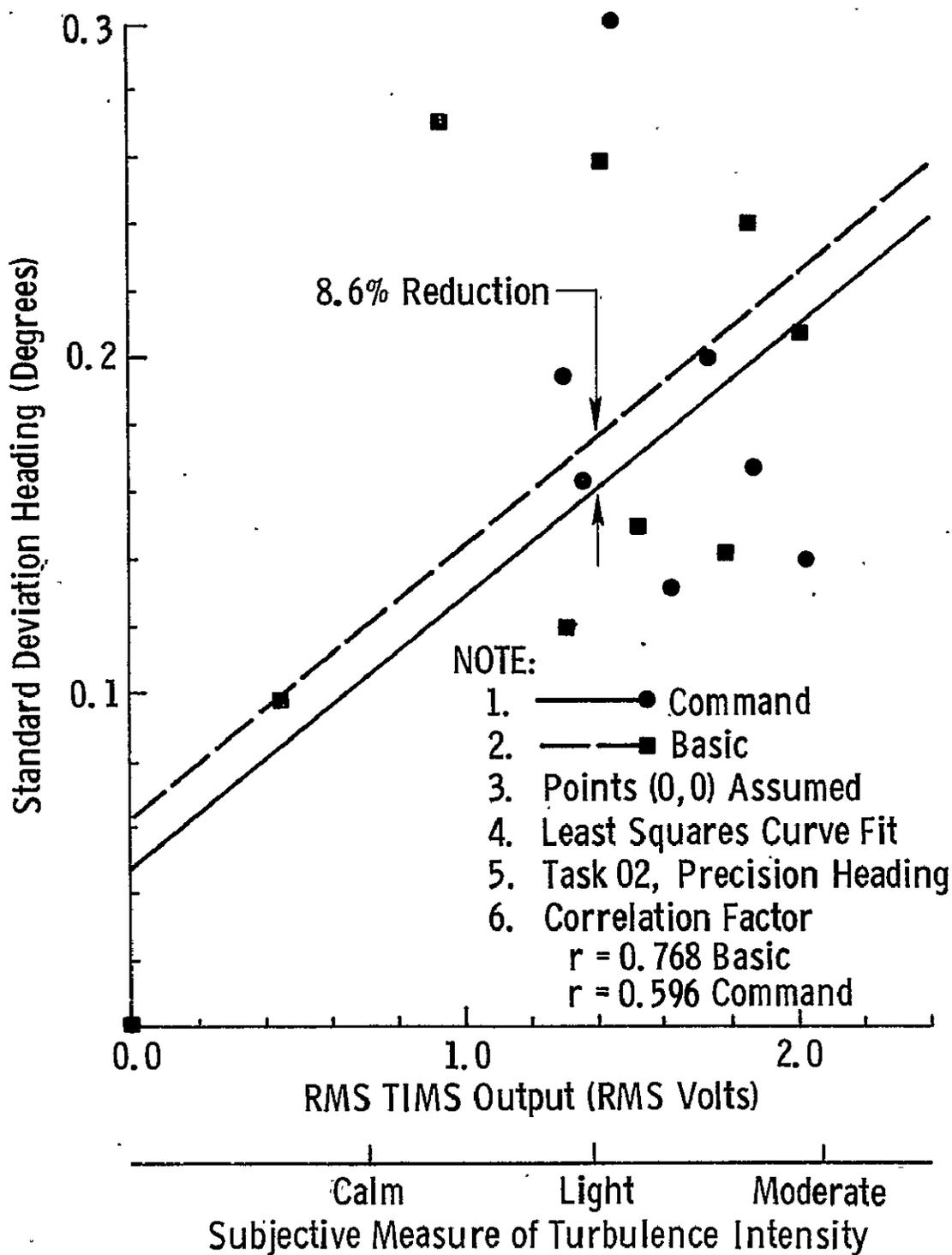
FIGURE 9.7 Least Squares Curve Fit to the Standard Deviation of SSSA Model 99 Heading as a Function of RMS TIMS Output for the Precision Heading Task
