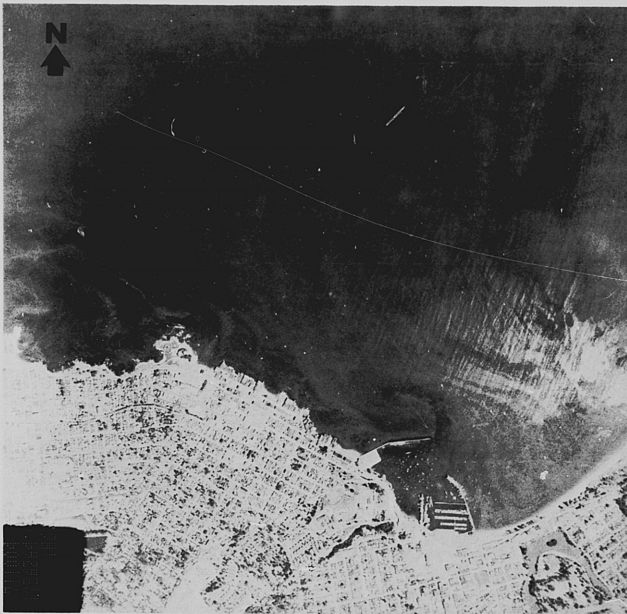
Figure 4-5 Southern Monterey Bay and Monterey Harbor Area Imaged on 4 Oct 1971, from NASA Mission 186, Altitude of 10,000 Feet. Original Photography was in Yellow Filtered Color and Defined Currents, Sediments and Red Tide Bloom.
