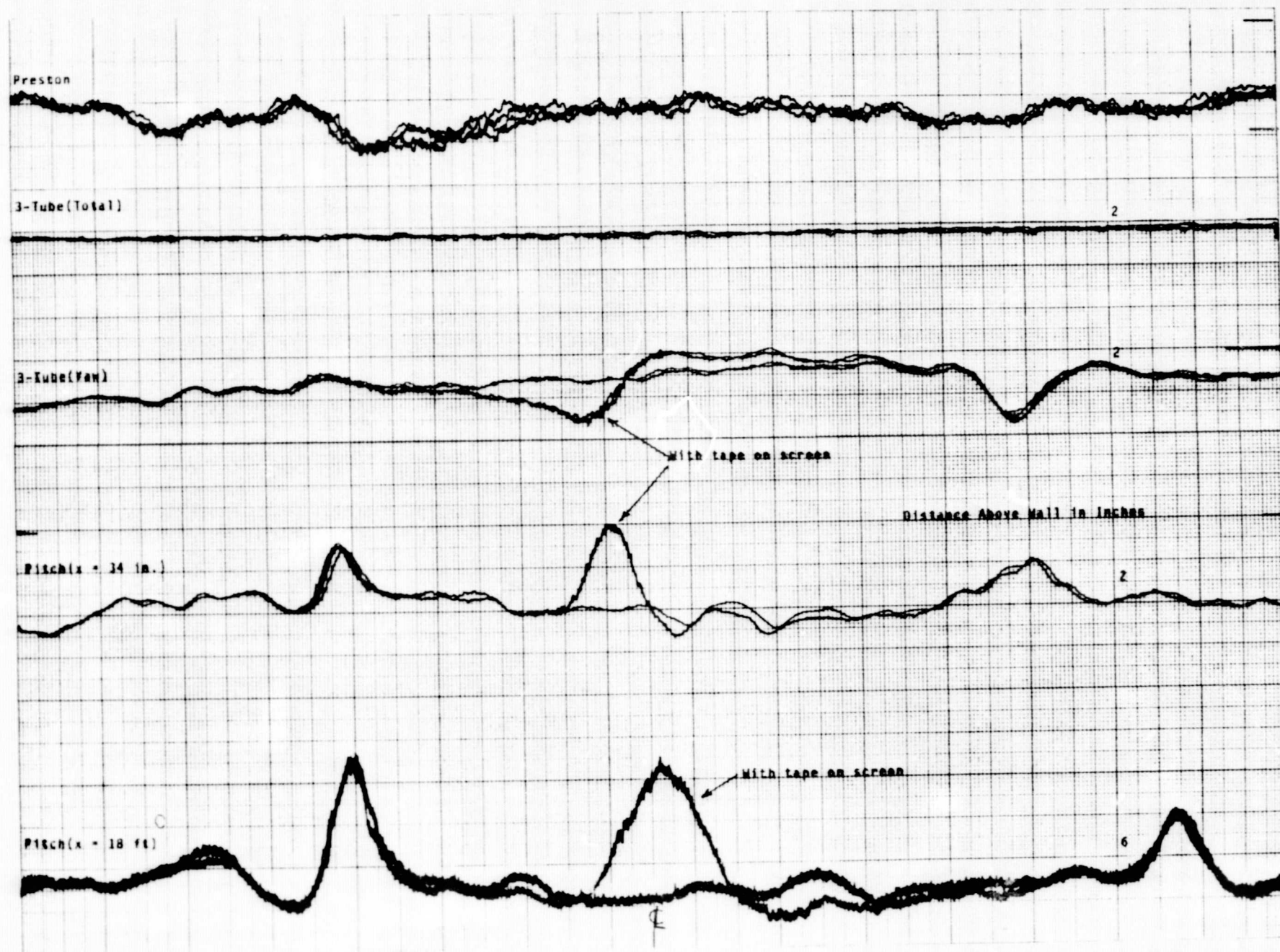
Fig.36 Effects of a 0.05 in. Wide Tape Placed on C of Last Inlet Damping Screen
