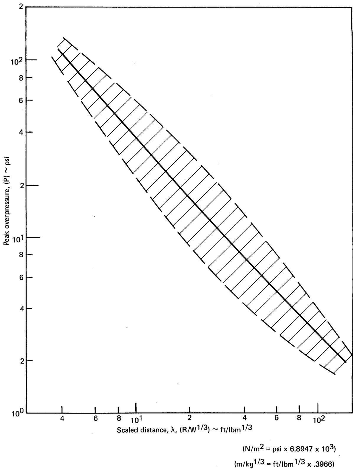
**FIGURE 5-28. — PRESSURE VS. SCALED DISTANCE. HYPERGOLIC PROPELLANT; CMB AND CBGS FAILURE MODES. (REF. 54)**
