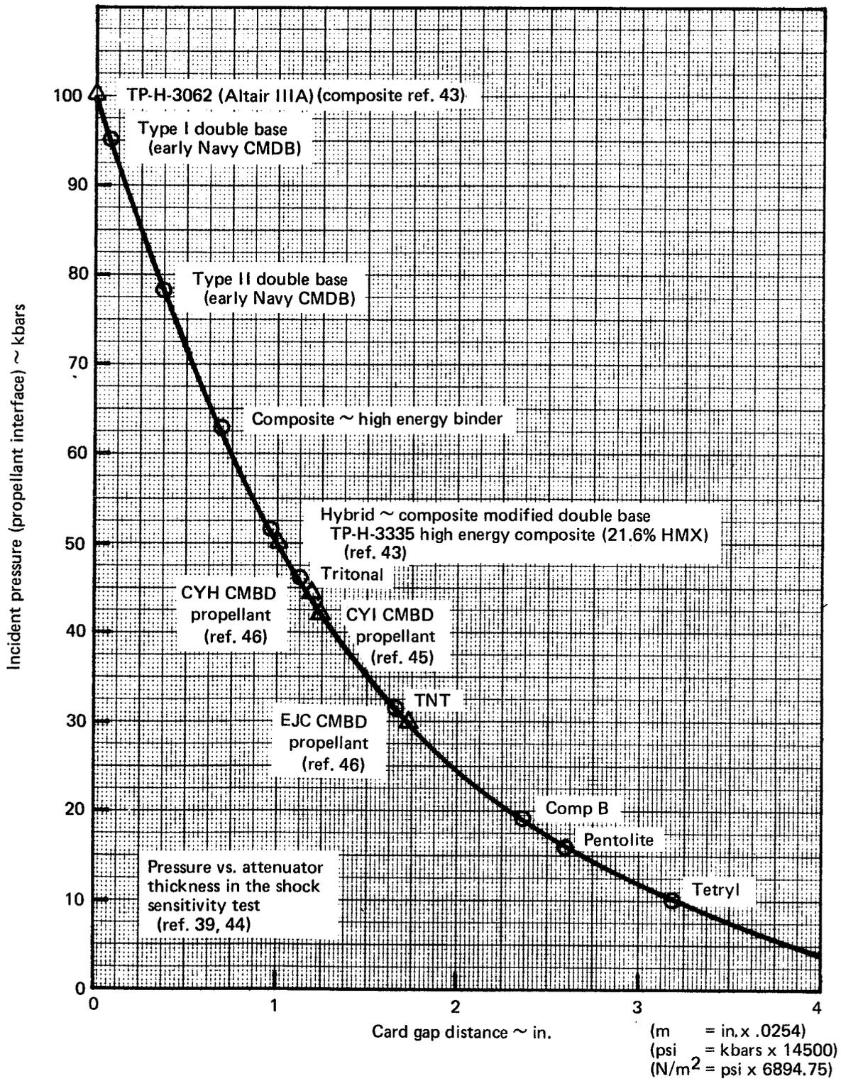
FIGURE 5-10. — INCIDENT PRESSURE IN CARD GAP TEST
