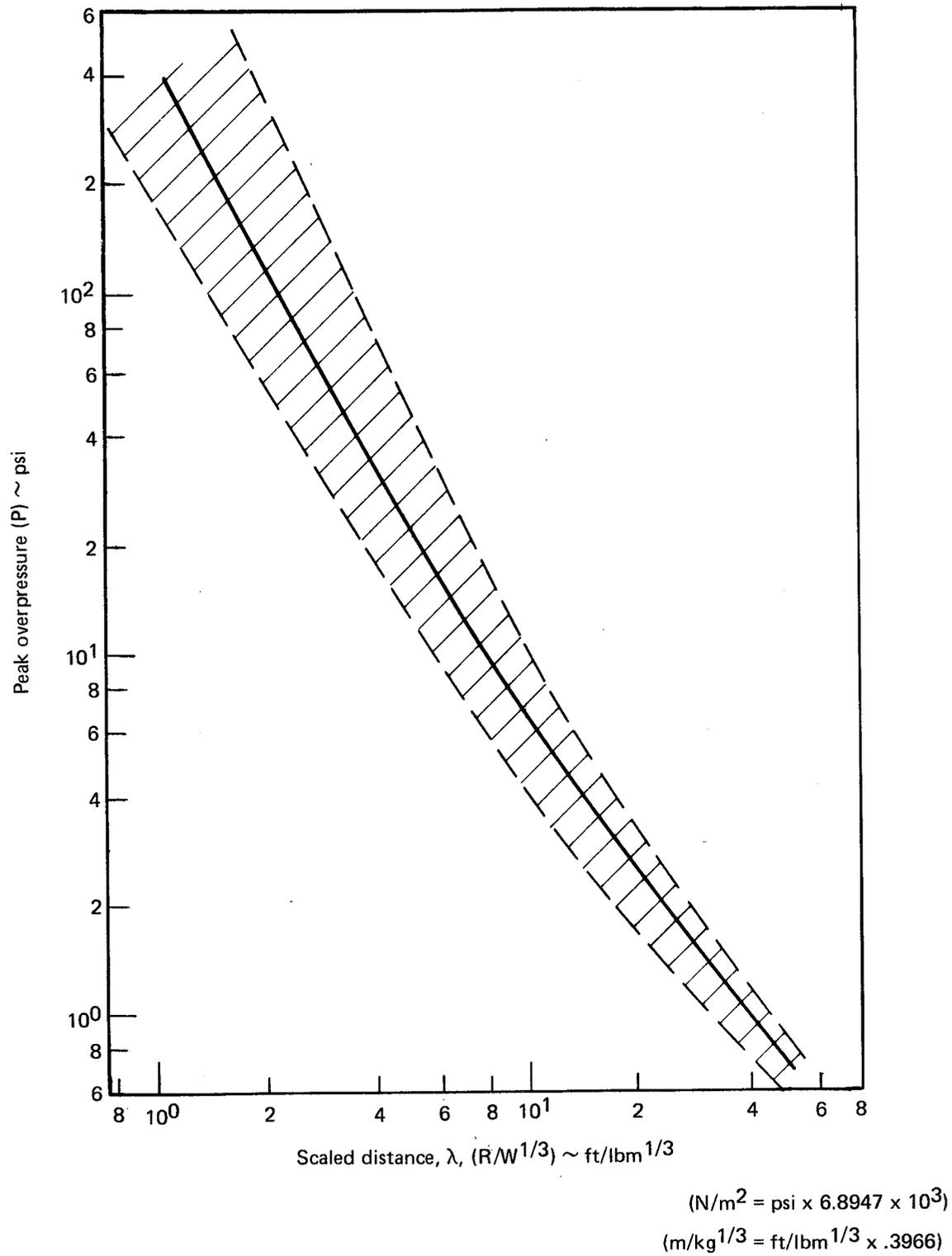
**FIGURE 5-36. — PRESSURE VS SCALED DISTANCE. LO<sub>2</sub>/LH<sub>2</sub> PROPELLANT; CBGS AND HVI FAILURE MODES. (REF. 54)**
