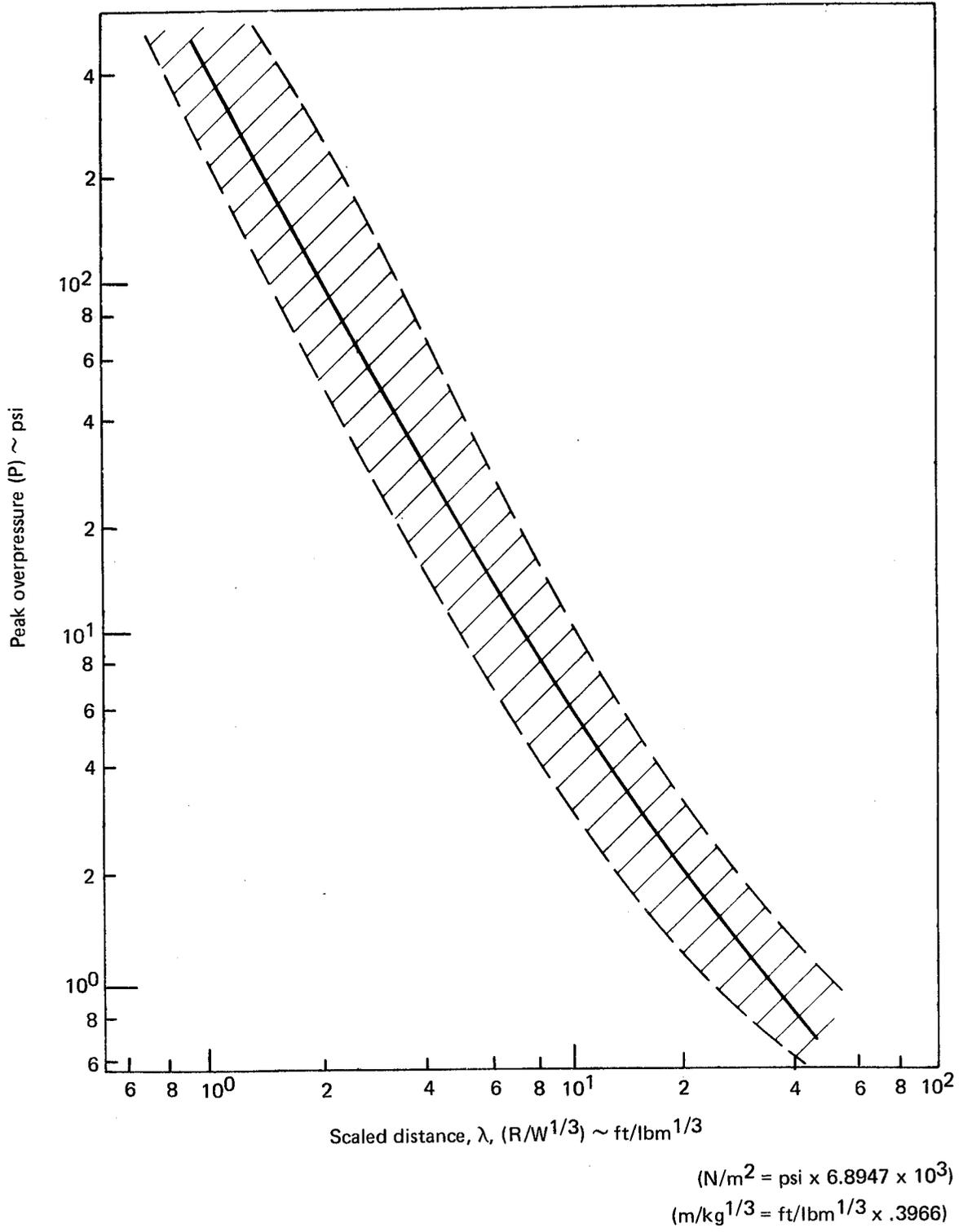
**FIGURE 5-35. — PRESSURE VS SCALED DISTANCE. LO<sub>2</sub>/LH<sub>2</sub> PROPELLANT; CBM FAILURE MODE (REF. 54)**
