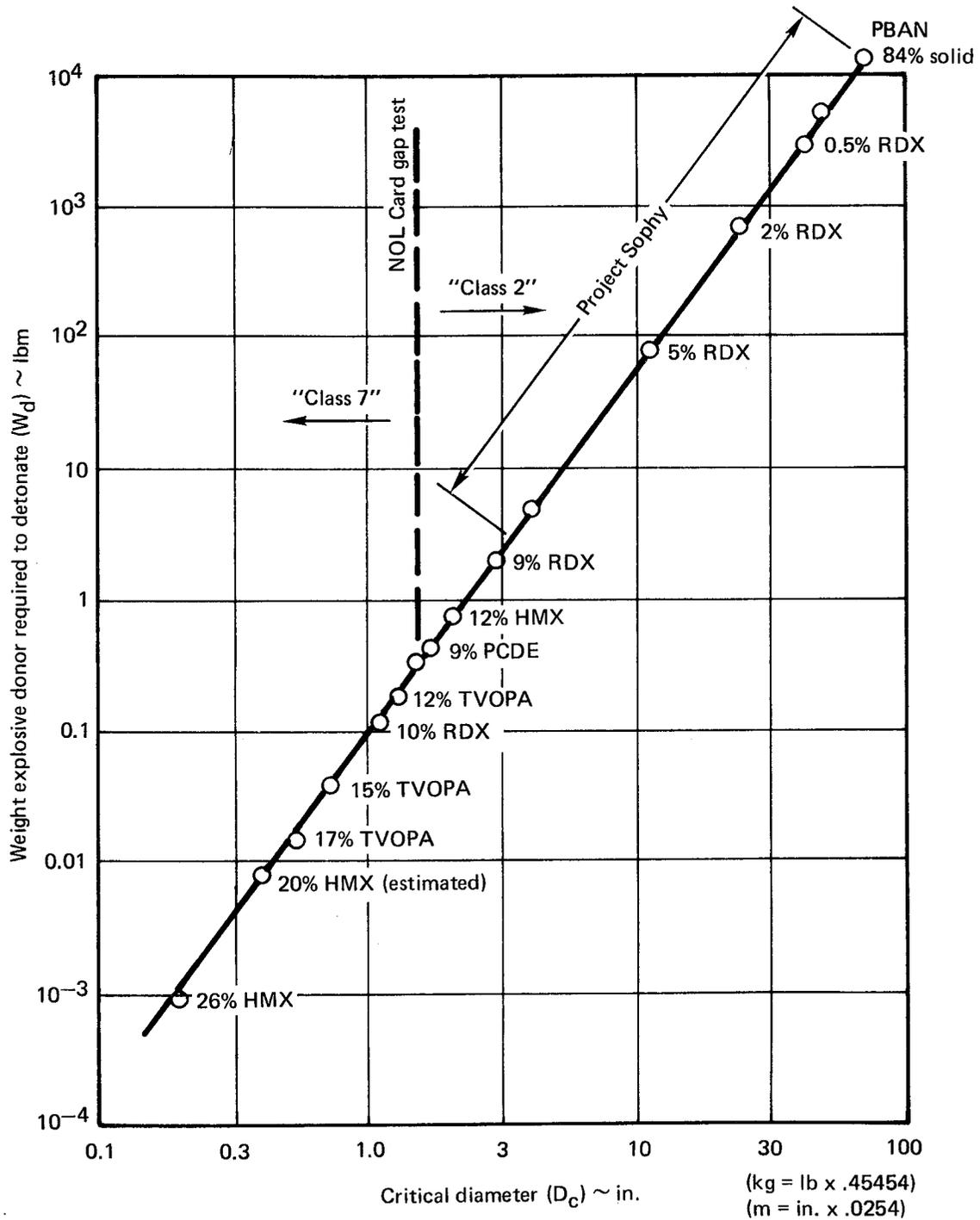
FIGURE 5-6. — EFFECT OF HIGH ENERGY INGREDIENTS ON CRITICAL DIAMETER AND EXPLOSIVE BOOSTER SIZE REQUIRED TO DETONATE SOLID PROPELLANTS (REF. 7)
