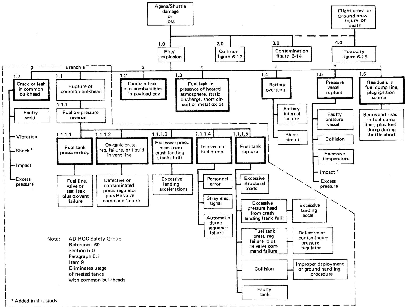
FIGURE 6-12. — FIRE/EXPLOSION HAZARD DIAGRAM
