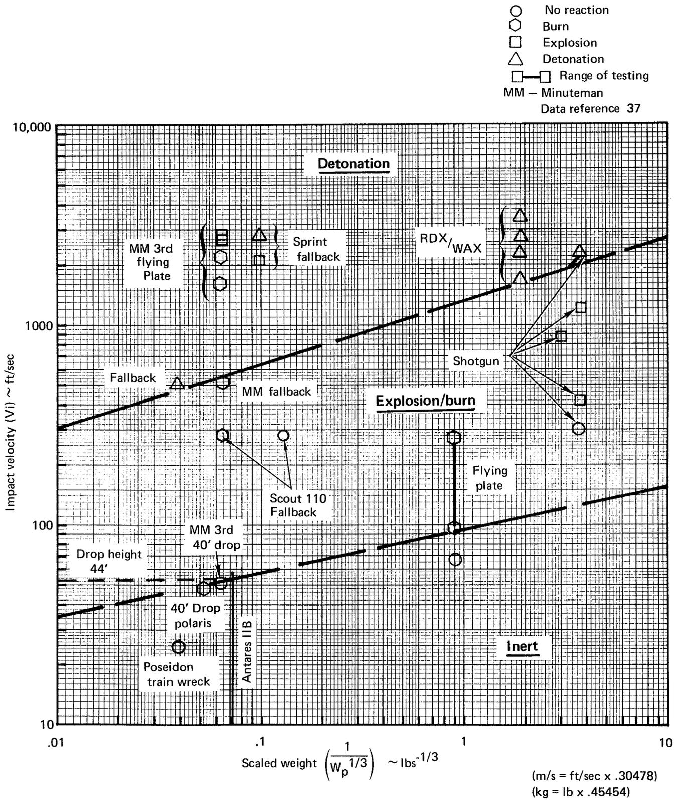
FIGURE 5-2. — DOUBLE BASE (CMDDB): IMPACT VELOCITY VS. PROPELLANT WEIGHT
