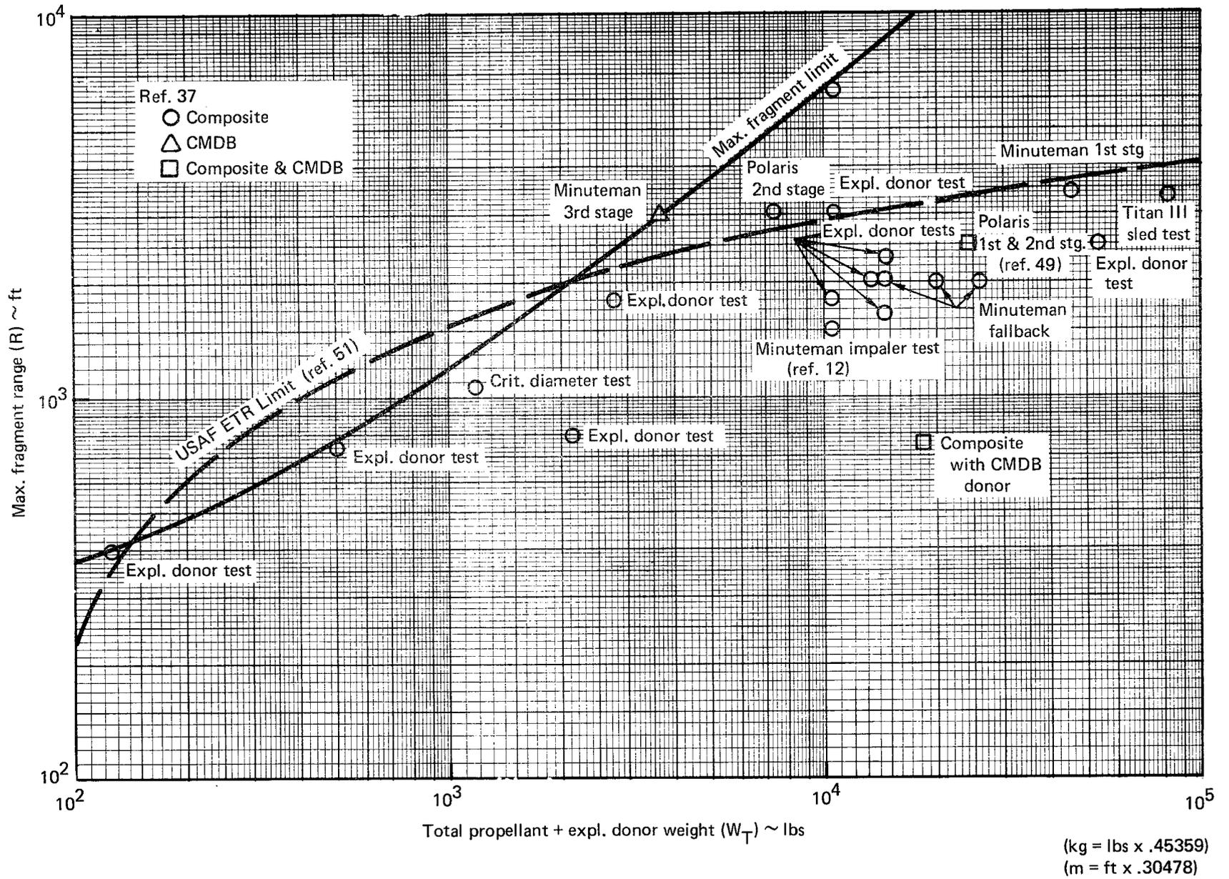
FIGURE 5-18. — MAXIMUM FRAGMENT RANGE — SOLID PROPELLANT SYSTEMS
