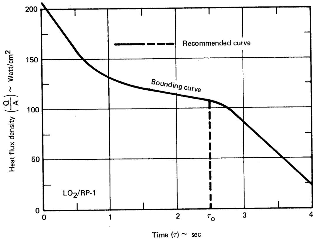
FIGURE 5-41. — BOUNDING AND RECOMMENDED HEAT FLUX DENSITY CURVES (REF. 35)
