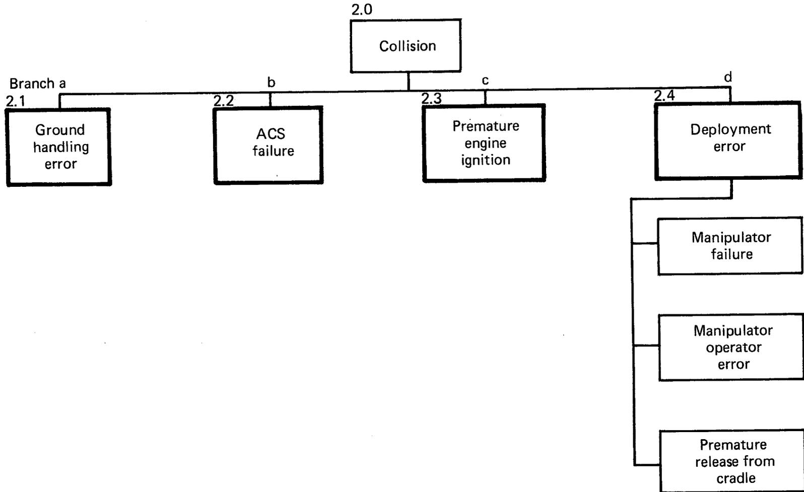
FIGURE 6-13. — COLLISION HAZARD DIAGRAM
