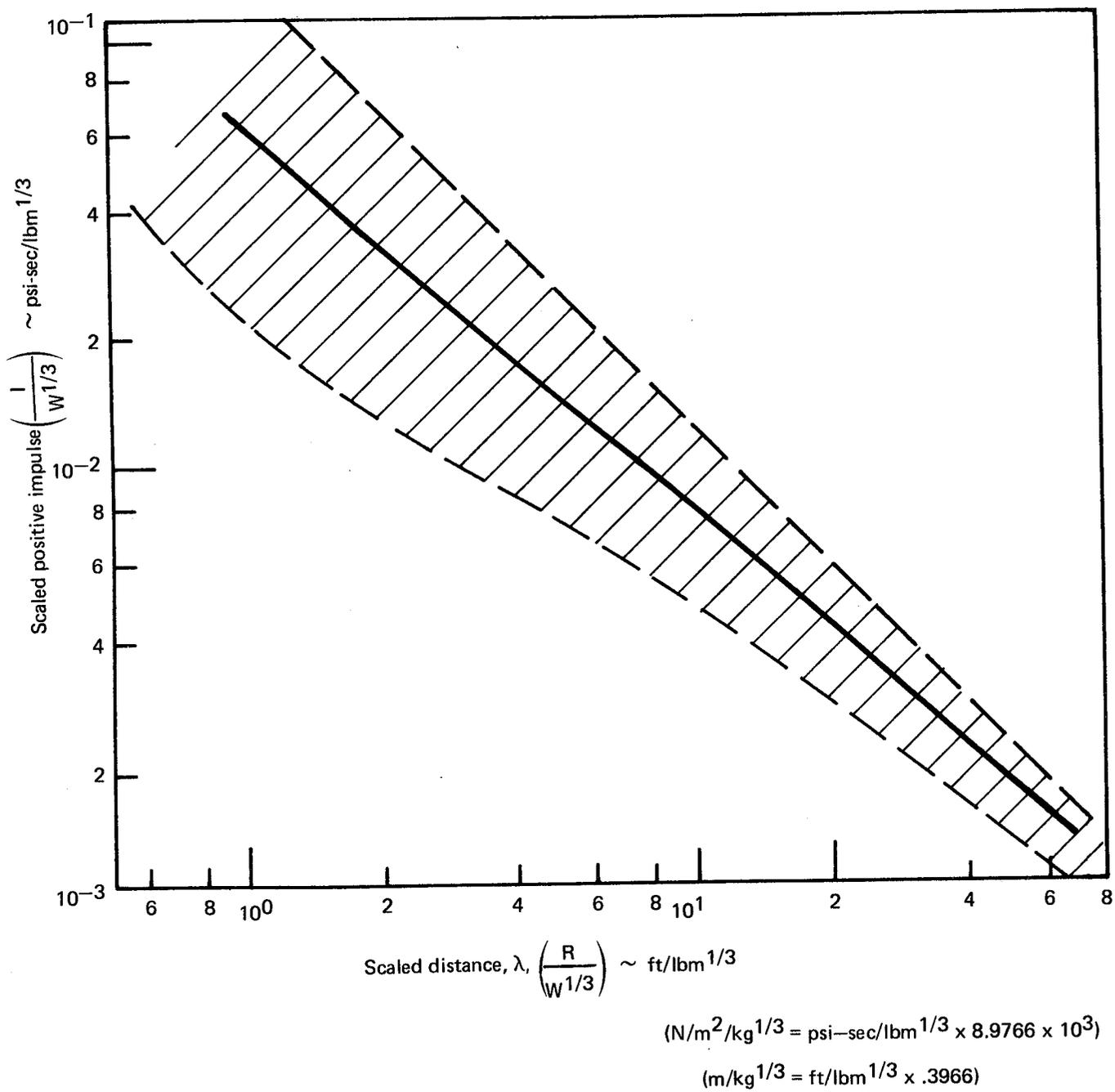
**FIGURE 5-38. — SCALED POSITIVE IMPULSE VS SCALED DISTANCE. LO<sub>2</sub>/LH<sub>2</sub> PROPELLANT; CBGS AND HVI FAILURE MODES (REF. 54)**
