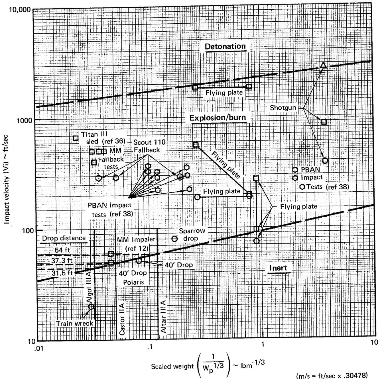
FIGURE 5-1. — COMPOSITES: IMPACT VELOCITY VS. PROPELLANT WEIGHT
