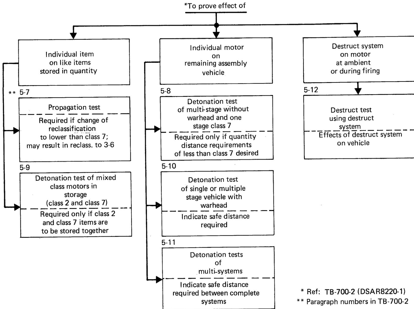
FIGURE 3-2. — MINIMUM TEST CRITERIA FOR DOD ROCKET MOTORS OR DEVICES CONTAINING SOLID PROPELLANT
