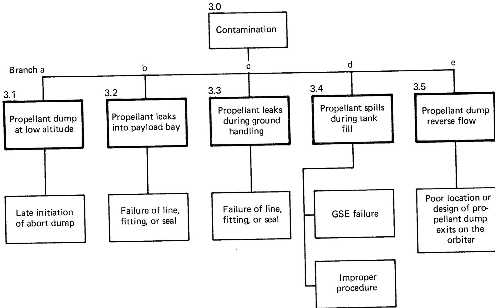
FIGURE 6-14. – CONTAMINATION HAZARD DIAGRAM
