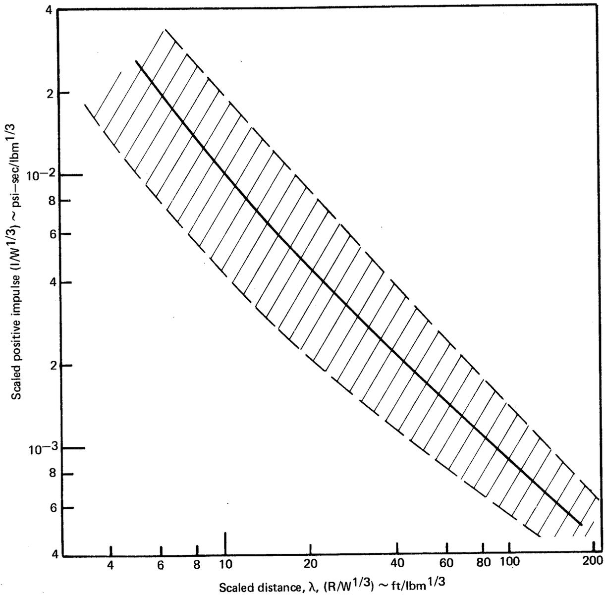
**FIGURE 5-30. — SCALED POSITIVE IMPULSE VS. SCALED DISTANCE.
