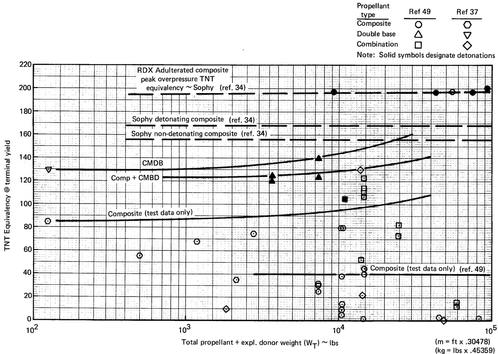
FIGURE 5-15. — TNT EQUIVALENCY AT TERMINAL YIELD — SOLID PROPELLANT SYSTEMS
