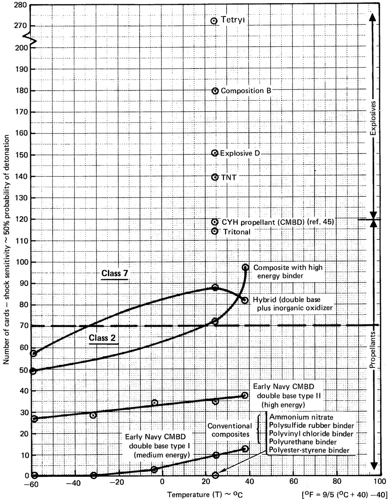
FIGURE 5-9. - CARD GAP TEST: NUMBER OF CARDS VS. TEMPERATURE (REF. 39, 44)
