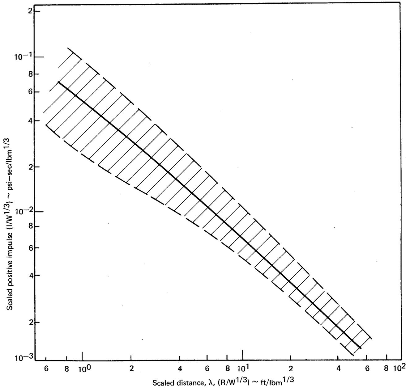
**FIGURE 5-34. — SCALED POSITIVE IMPULSE VS SCALED DISTANCE.
