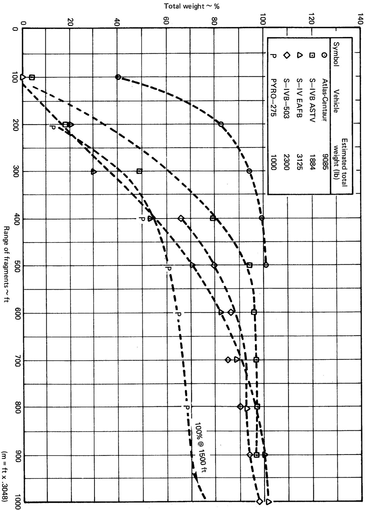
FIGURE 5-44. — PERCENTAGE OF TOTAL WEIGHT OF VEHICLE FRAGMENTS WITHIN RANGE INDICATED (REF. 61)
