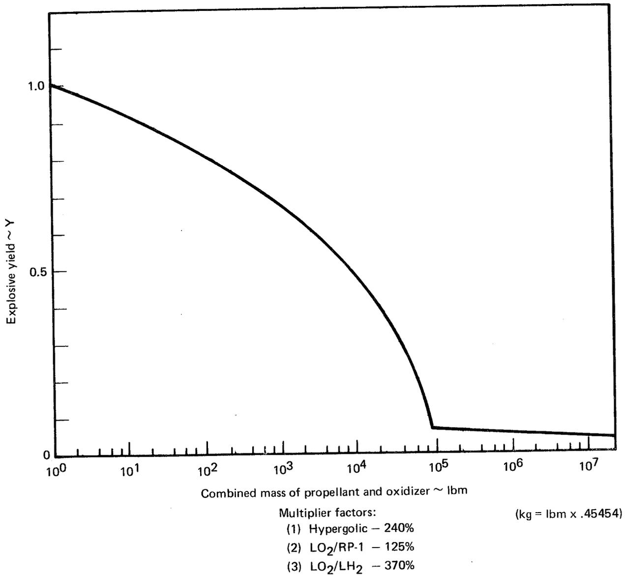
**FIGURE 5-20. — ESTIMATED TERMINAL YIELD AS A FUNCTION OF COMBINED PROPELLANT AND OXIDIZER MASS (REF. 54)**
