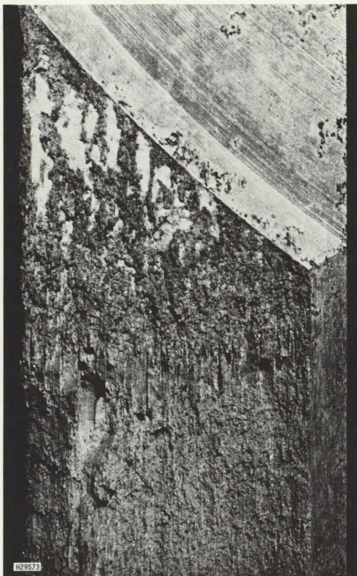
Figure E1. (f) Fracture surface of TL DCB from 1.25-in. 7049-T7351(T) plate exposed 6.5 mo. at Daytona Beach
