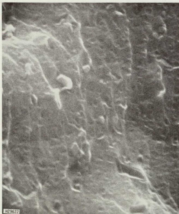
Figure F5. Stress corrosion fracture surface on SL-DCB specimen from 1.25-in. 7075-T7351 plate: salt-chromate environment (45°)
