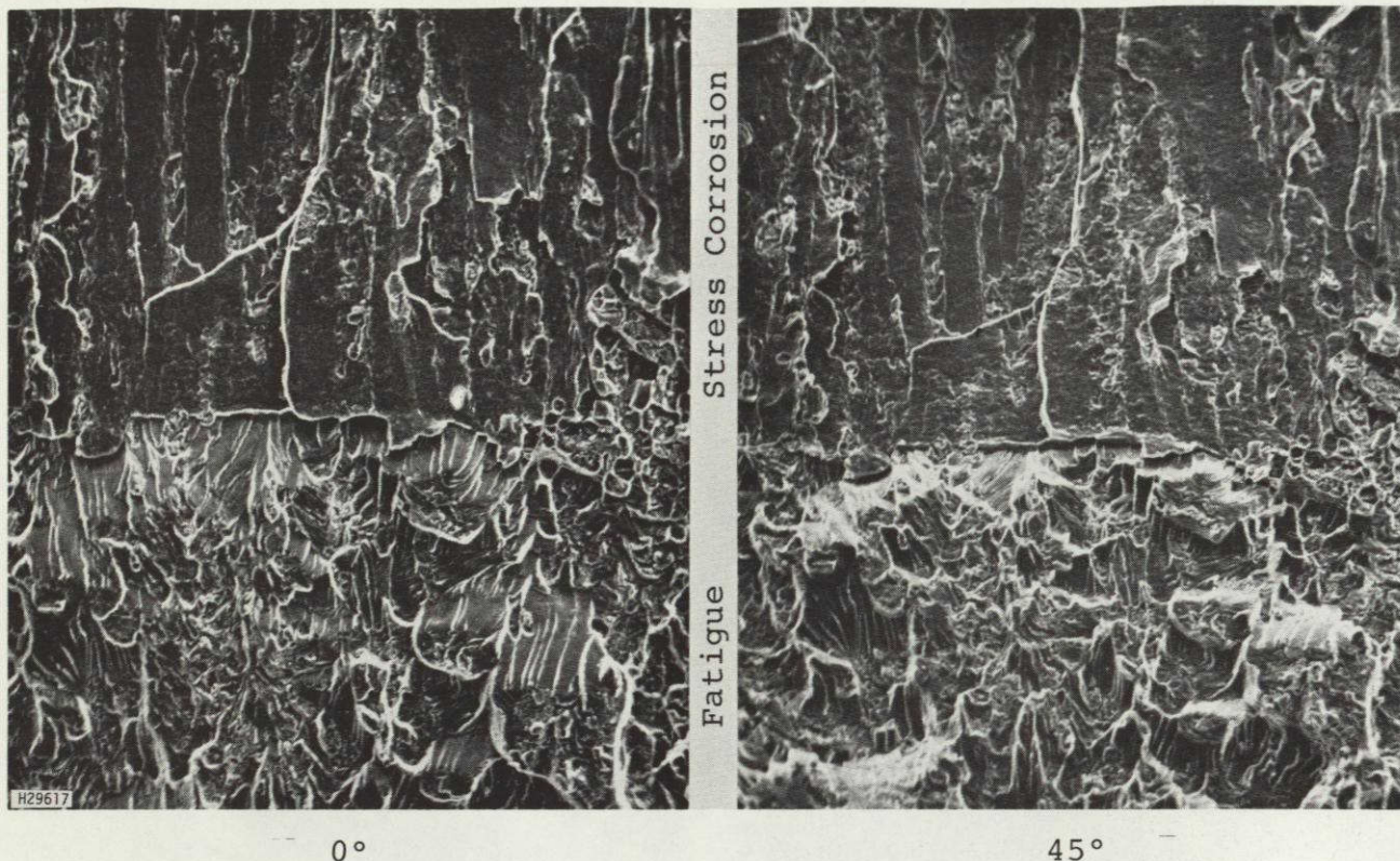
Figure F2. Fatigue precrack/stress corrosion interface on SL DCB from 1.25-in. 7075-T7351 plate: salt-chromate environment (100X)
