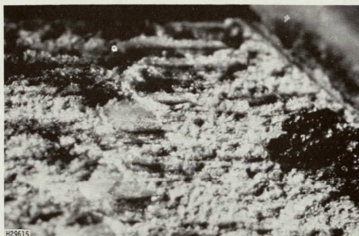
Figure E3. Cracks growing normal to precrack plane in TL specimen
