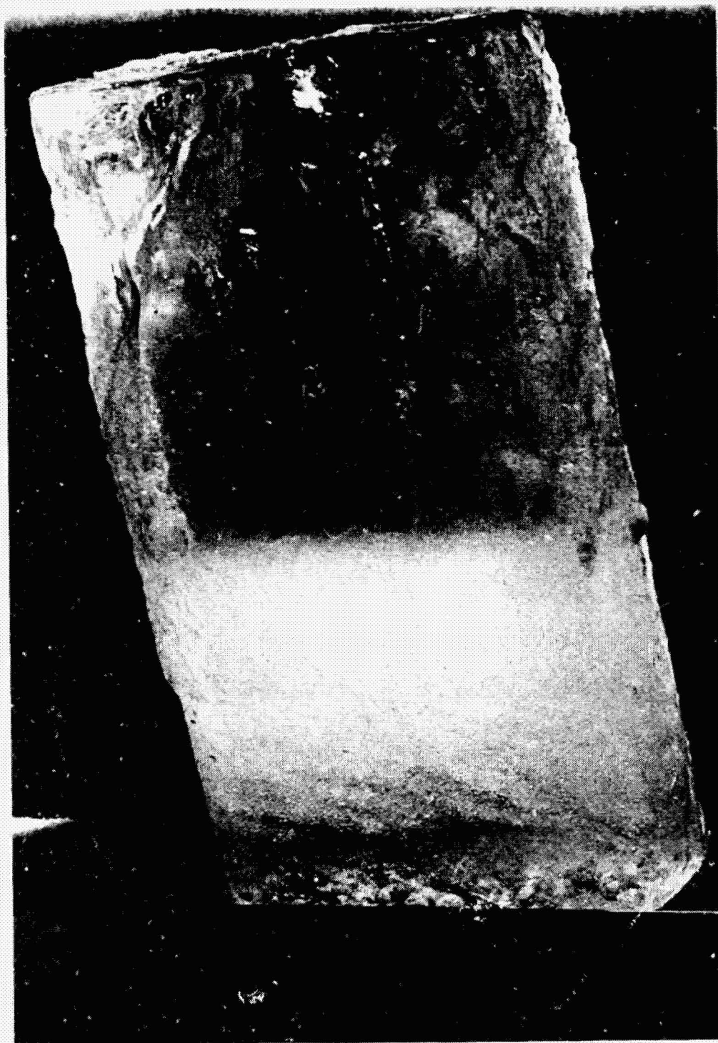
FIGURE 4 ICE SAMPLE 3 SHOWING LAYERS OF INCLUSIONS
