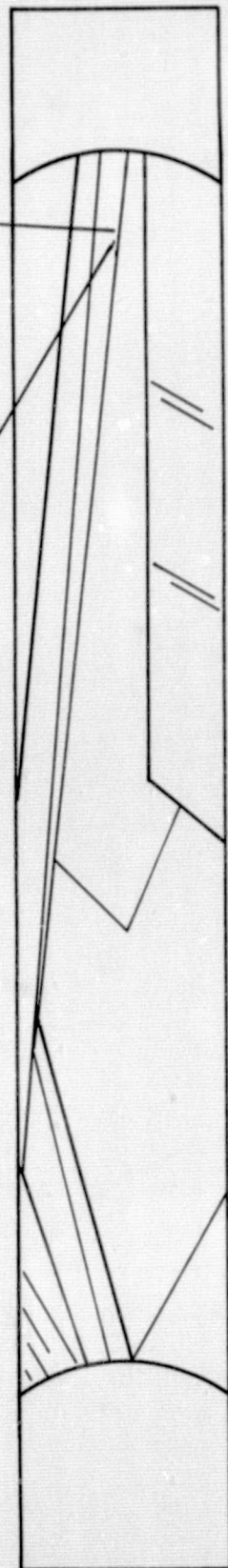
FIGURE 8 Sample grown from single crystal feedstock using a curved molten zone.
