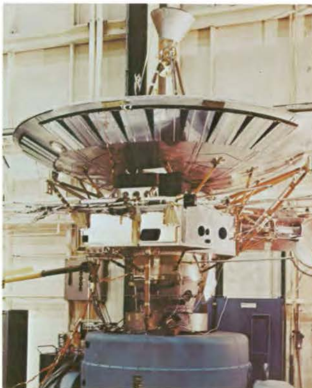
Figure 2-2. The Pioneer spacecraft itself was designed for high reliability using space-proven components. TRW Systems designed and fabricated the two Jupiter spacecraft, Pioneers F and G, at their Redondo Beach, California, facility.
