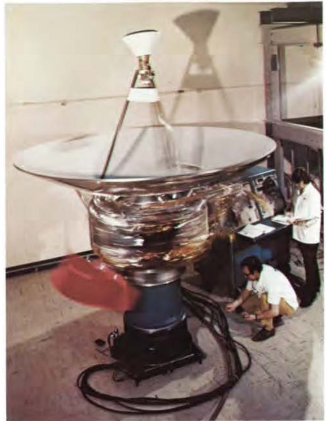
Figure 3-2. Each Pioneer spacecraft is stabilized by rotation as shown under test here.
