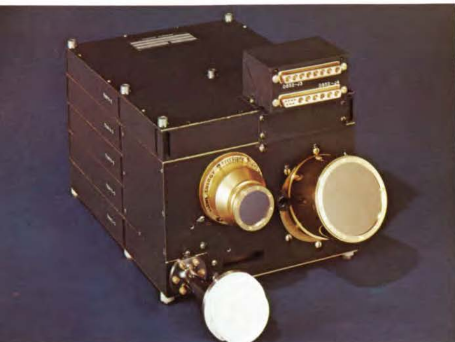
Figure 4-4. Charged particle detectors are used to study the life history of cosmic rays in the Solar System.
