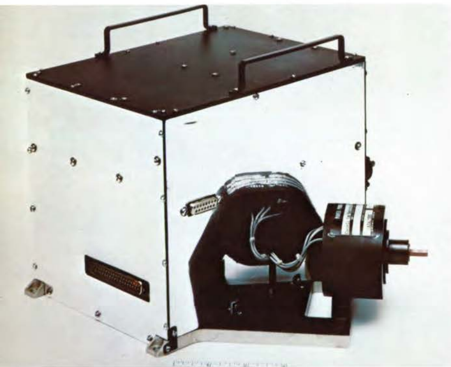
Figure 4-5. A combination of cosmic ray telescopes seeks further information on the composition of the cosmic ray particles and their energy ranges.
