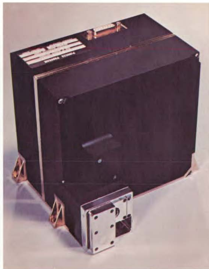
Figure 4-6. Other telescopes are used to explore the radiation belts of Jupiter, measuring electrons and protons in these belts.
