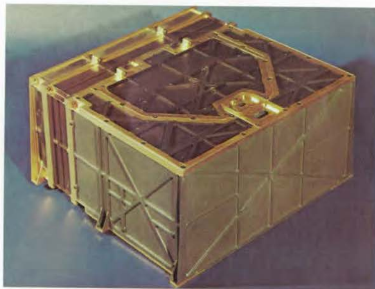
Figure 4-3. A plasma analyzer peers through a hole in the large dish-shaped antenna to detect particles of the solar wind originating from the Sun. (a) Shows the instrument in diagrammatic form. (b) Shows it ready for installation in the spacecraft.
