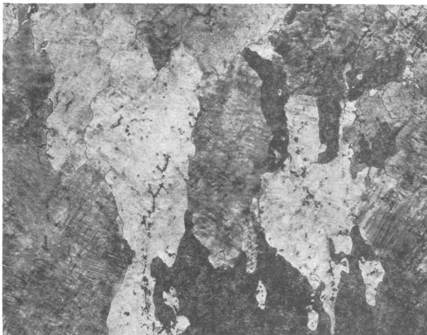
Figure 15.- Microstructure of 2124-T851 plate (perpendicular to short transverse direction)
