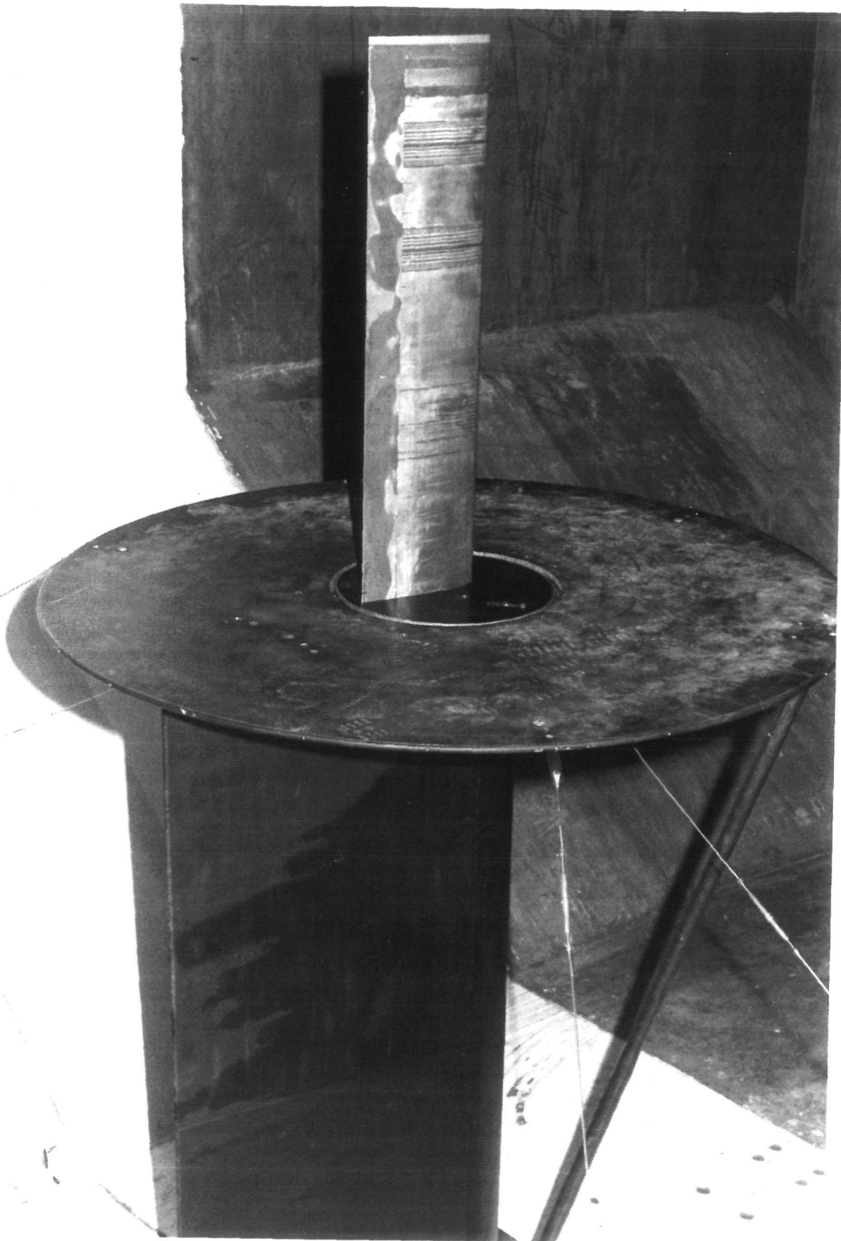
Figure 4. Wing Installed in wind tunnel.
