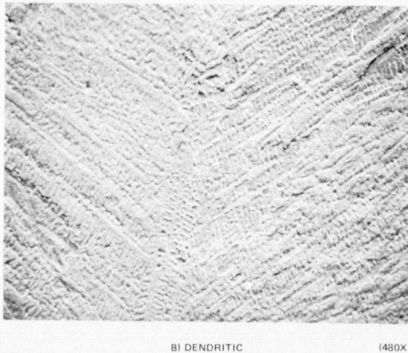
Fig. 12 Solidification Modes Found in Stainless Steel Alloy Welds A) Initial Transient and Cellular B) Cellular Dendrites
