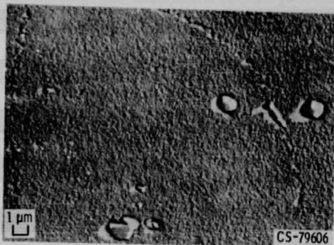
(a) 2 HOURS AT 1190°C PLUS 6 HOURS AT 1171°C.
