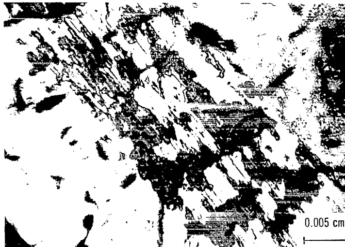
Figure 6. - Wear track on 3.02 percent carbon in gray cast iron after having been in sliding contact with a 52100 steel ball for 1 hour. Sliding velocity, 5 centimeters per minute; load, 50 grams; argon atmosphere; temperature, 23° C.
