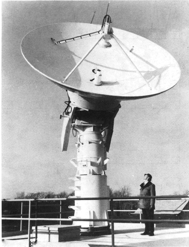
Figure 11. - Five-meter-diameter (16-ft) super-high-frequency Cassegrain antenna.
