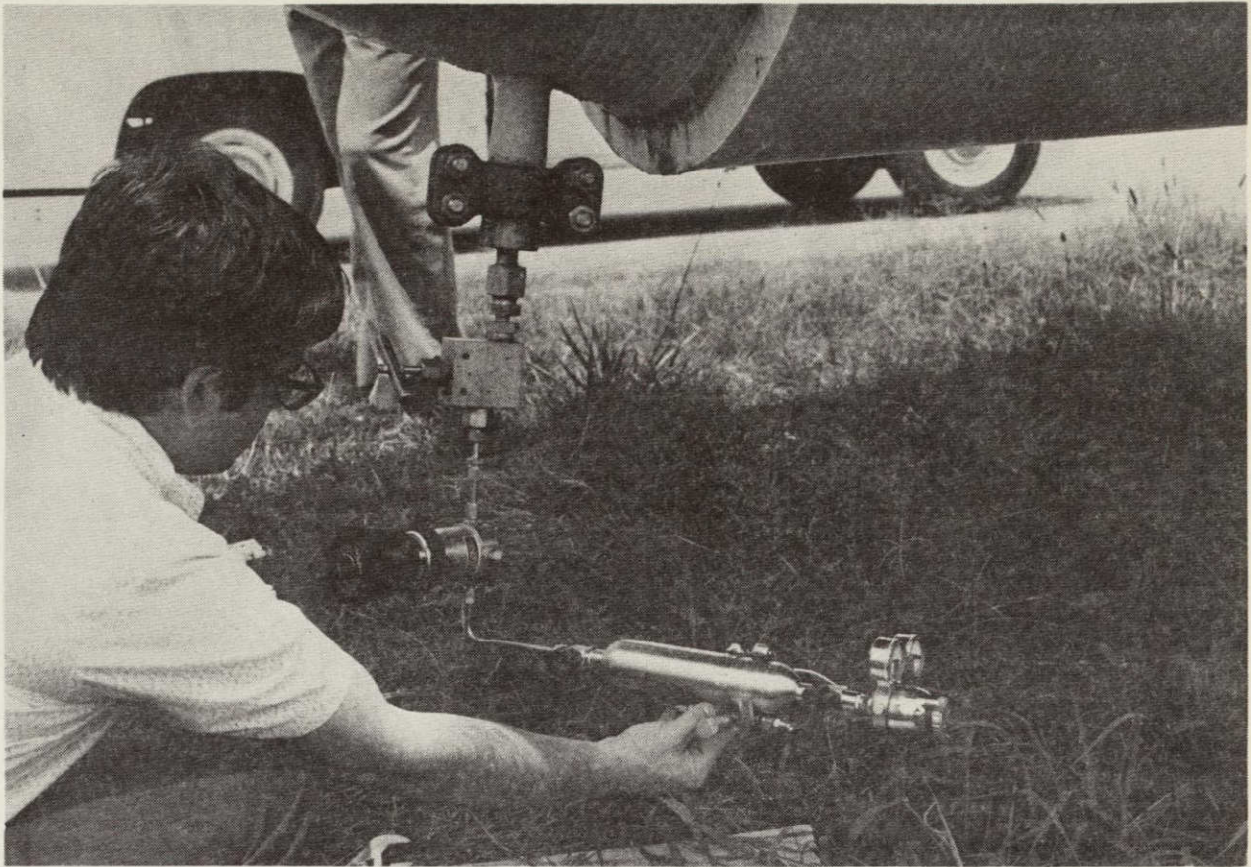
FIGURE 5. Sampling at the High Pressure Nitrogen Tank
