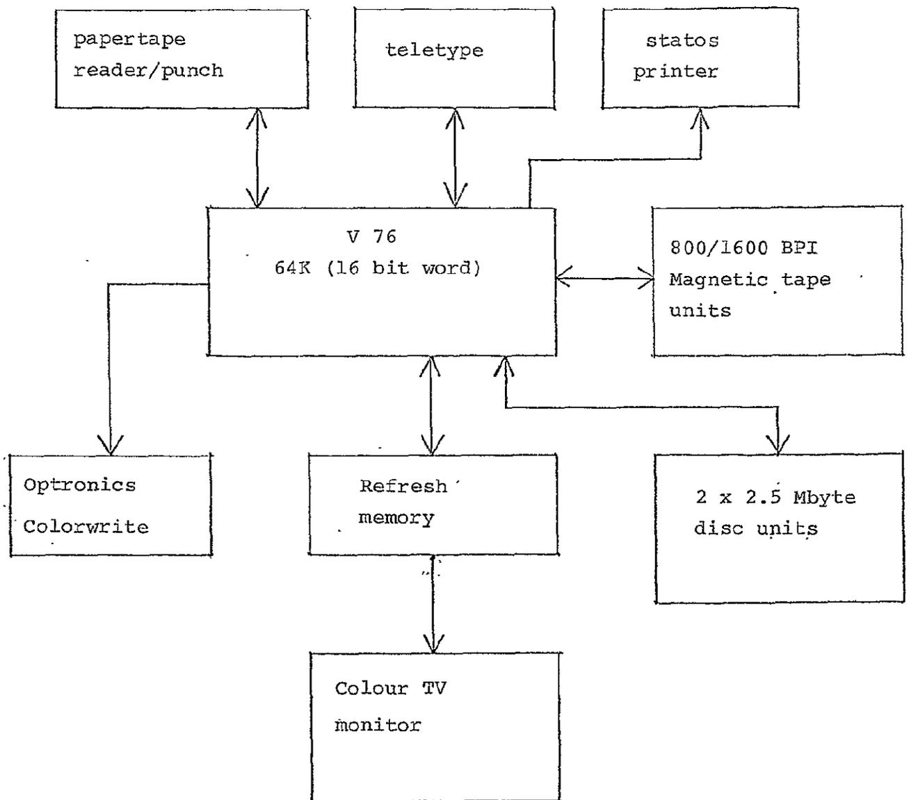
Figure 7.4 System configuration for image processing on the V 76 computer.
