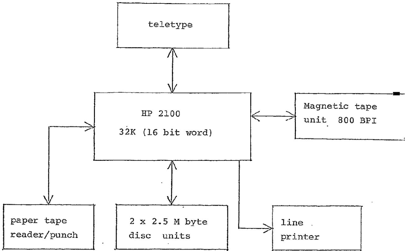
Figure 7.1 System configuration for image processing on the HP 2100 computer.
