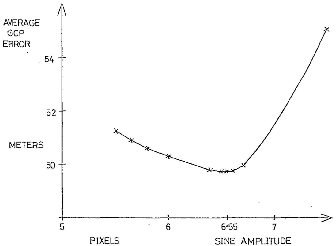
Figure 8.2 Average GCP error in meters versus amplitude of the sine error function in pixels in the along scan direction.
