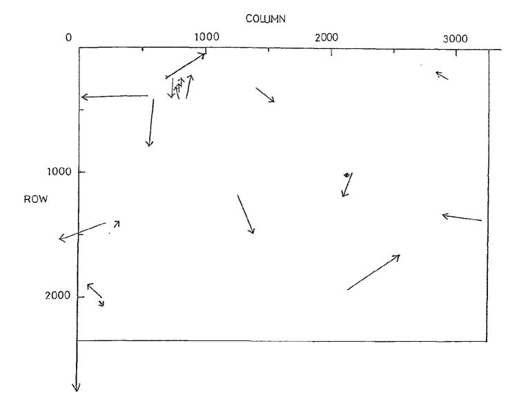
Figure 8.3 The positions of the 19 GCP's used in the geometric correction of LANDSAT scene 2334-21123 are shown by the start of the arrows. The length and direction of the arrows depict the mapping errors for each GCP.
