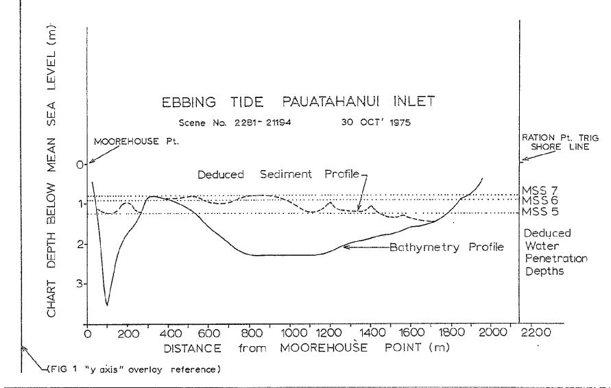
Fig. 12.3 Sediment profile deduced from Fig. 12.1 (bathymetry profile from Irwin, 1976) (Water penetration depth scale is identical to "Chart depth" scale.)
