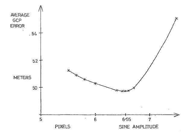
Figure 8.2 Average GCP error in meters versus amplitude of the sine error function in pixels in the along scan direction.
