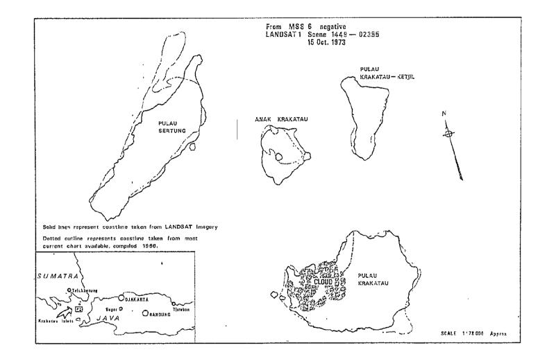
Fig. 13.2 1:78 000 outline map of the Krakatau group prepared from the MSS 6 negative of LANDSAT scene 1449-02355 recorded on 15 October 1973, with a 1966 compilation map contour overlaid in dots.
