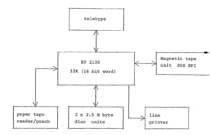
Figure 7.1 System configuration for image processing on the HP 2100 computer.
