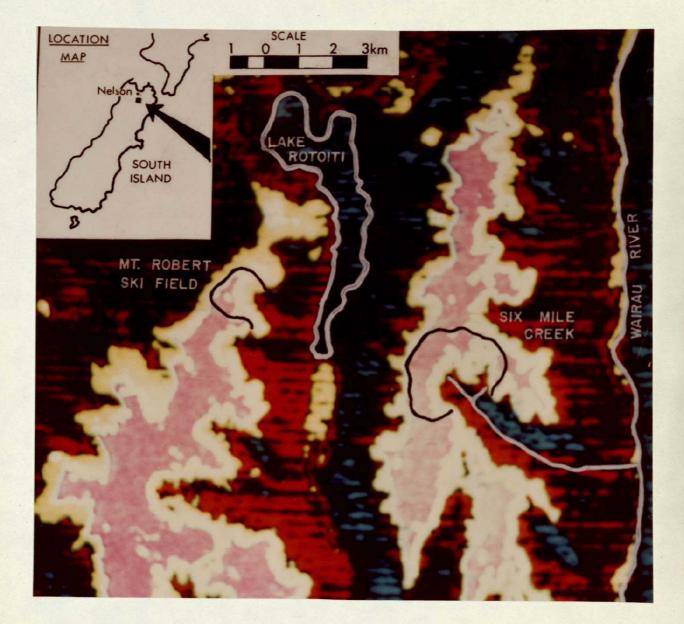
Fig. 11.1 Colour-coded isodemsitometer image of the MSS 4 positive transparency of part of scene 2282-21252 that was used in assessing the area of snow in the two basins and selecting the location of the transect. Inset: location map for the study.
