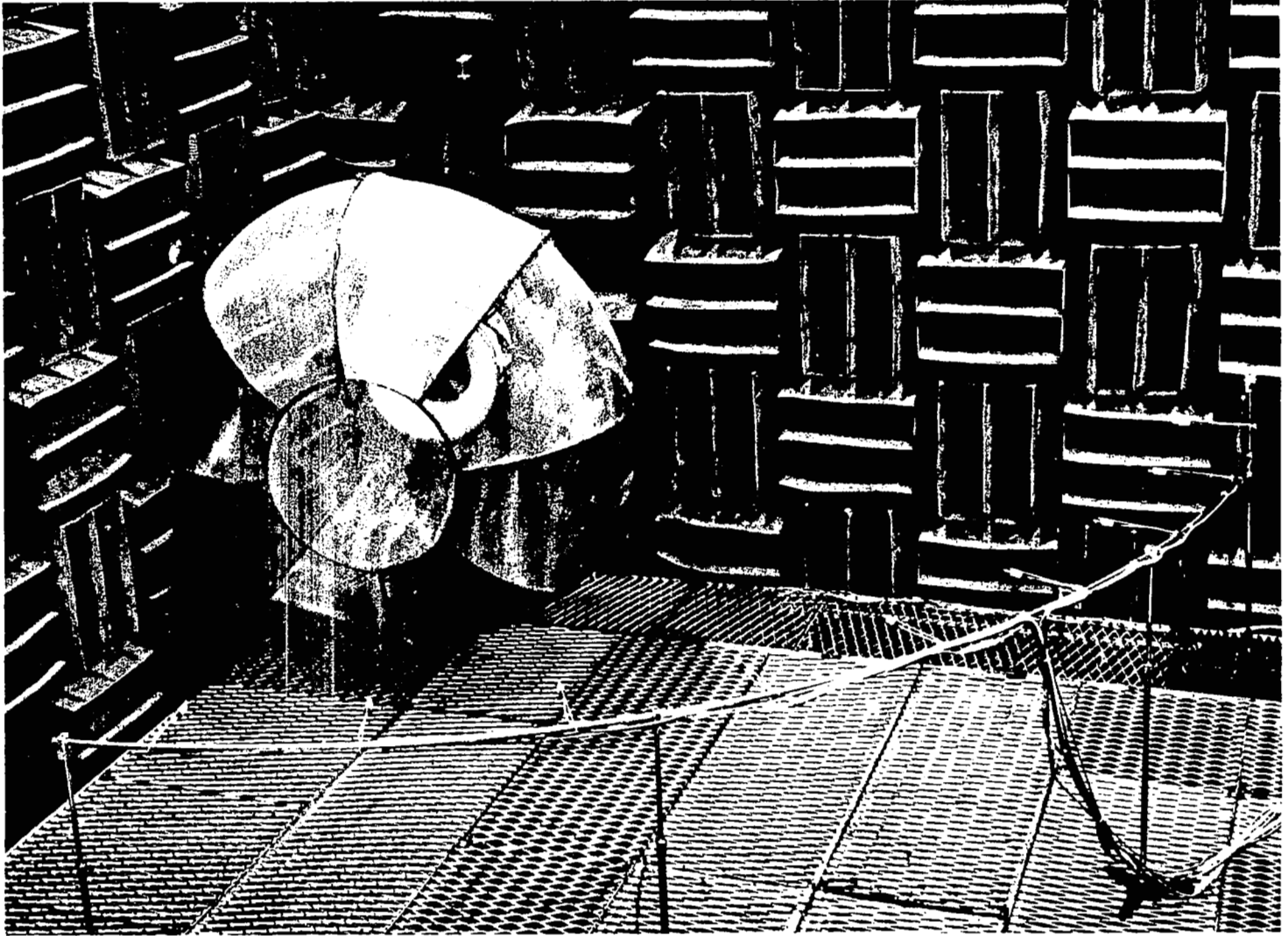
Figure 8. Inlet Turbulence Screen Installed on Test Vehicle.
