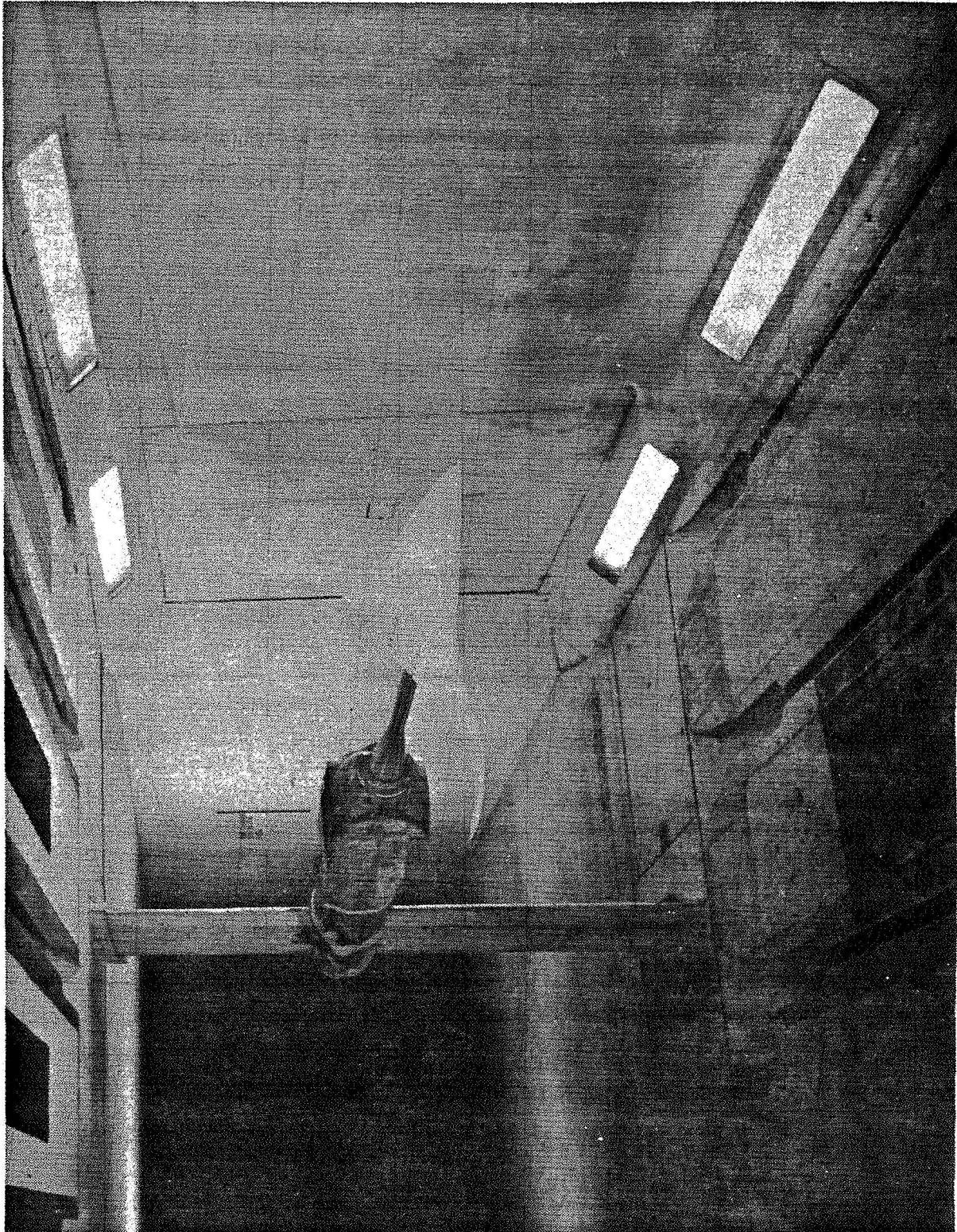
Figure 19. A force model mounted on the high angle stability sting.
