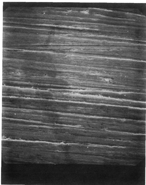
(a) As-machined copper surface. X1000.
