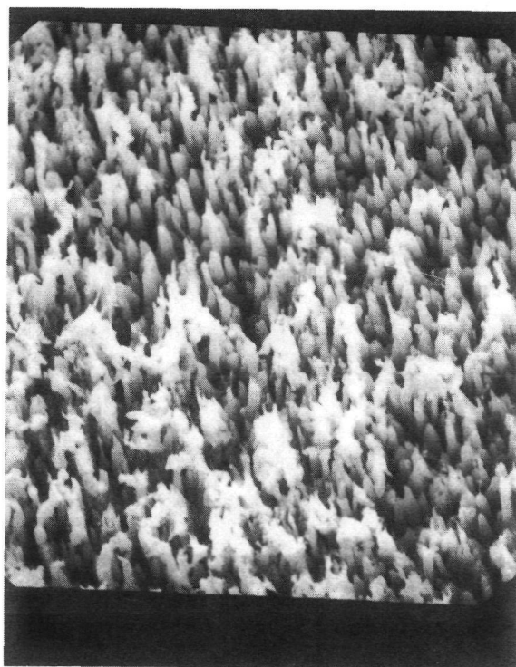
(c) Sputtered copper surface having needle-like protuberances.
