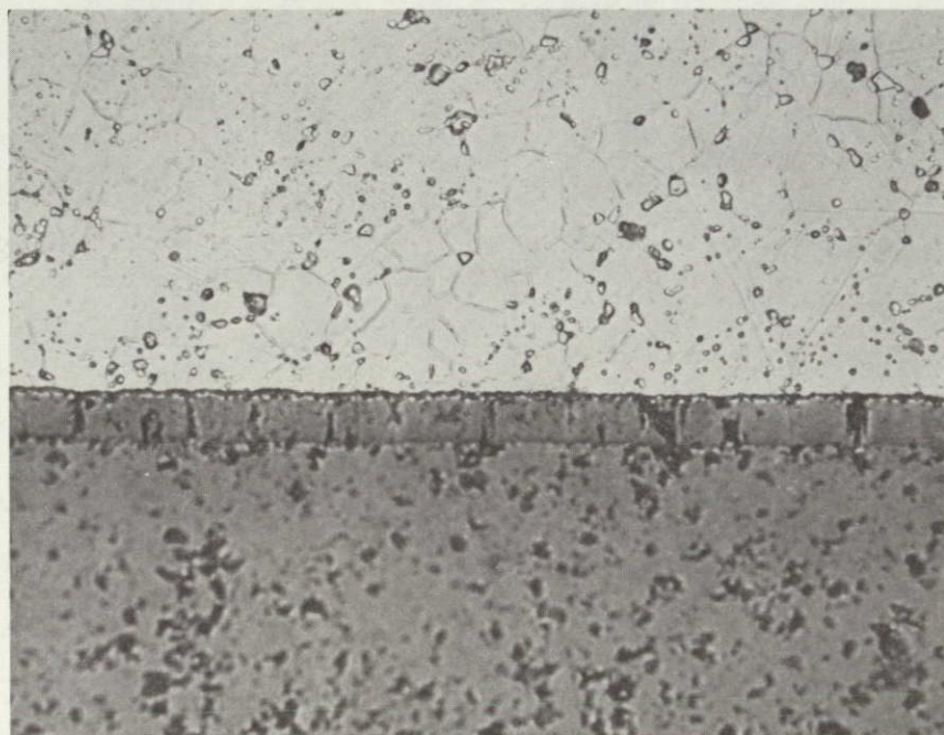
Fig. 8. Diffusion Couples Between Waspaloy and RF Sputtered HfC on a SiC Substrate, as HIP (a) and After 200 Hours at 982°C (1800°F) (b).
