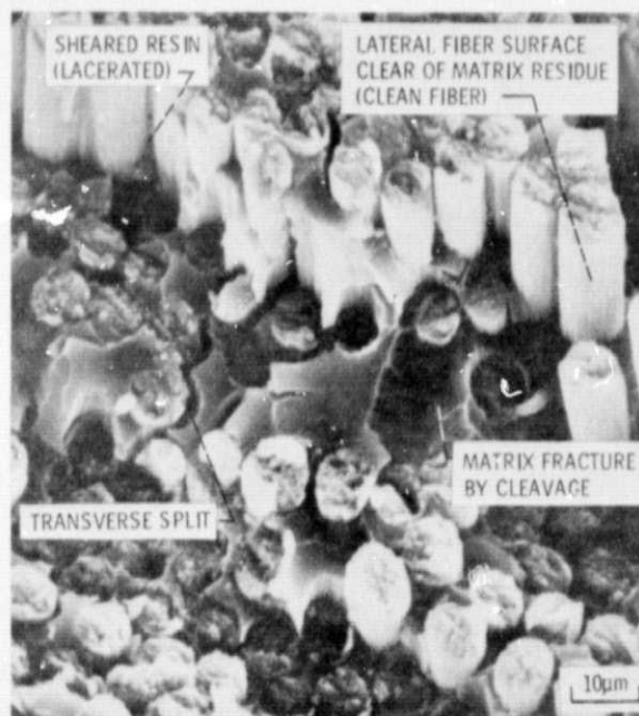
(c) ENLARGEMENT OF DETAIL IN (b) TO SHOW FRACTURE MODE.
