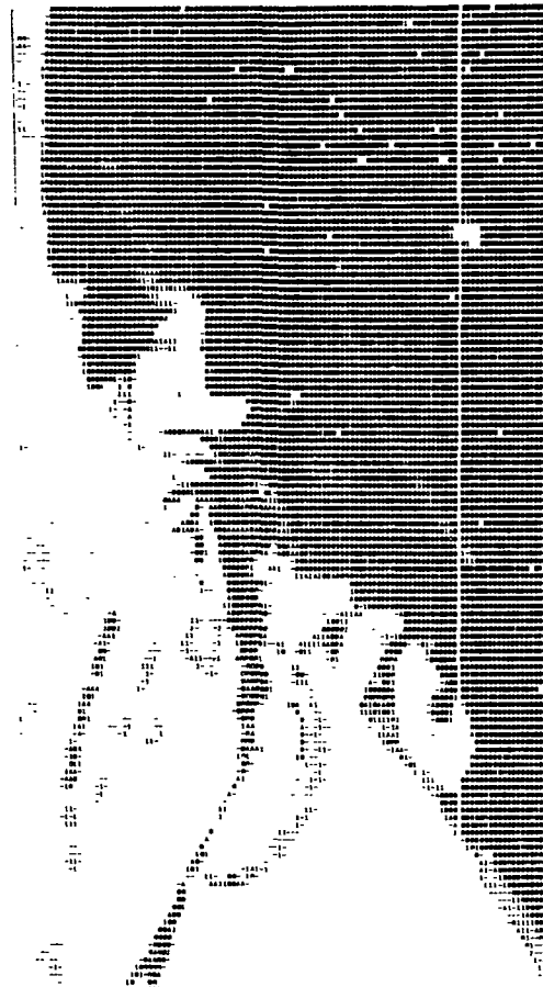
FIG.2. COPENHAGEN WASTE PLUMES. Grey-tone plot (line printer) covering the Copenhagen area (MSS 5, 27/8-73).
