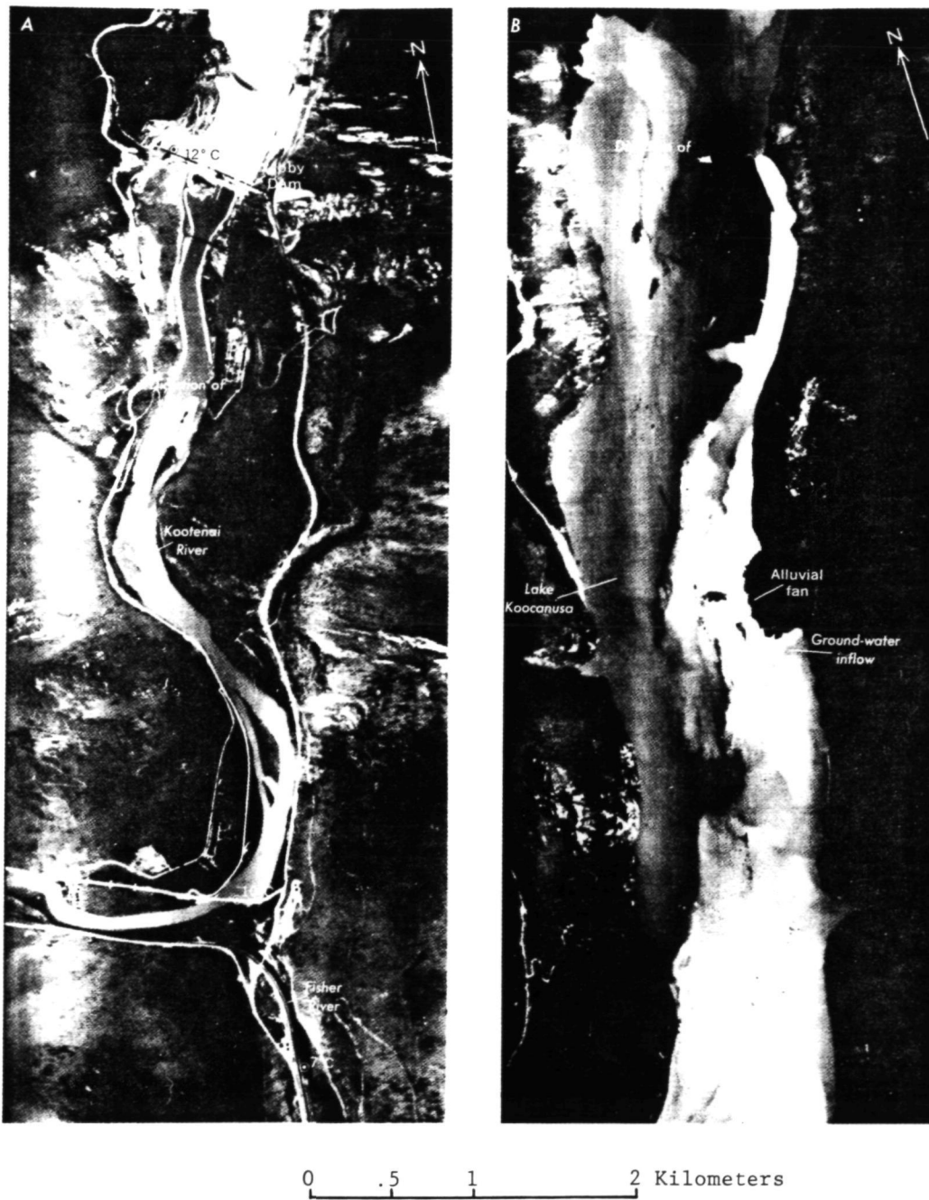
FIGURE 2. THERMAL-INFRARED IMAGERY AROUND LAKE KOOTENAI. A. Libby Dam and the confluence of the Fisher and Kootenai Rivers. B. Ground-water inflow to Lake Kootenai. Imagery by U.S. Forest Service
