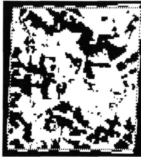
Fig. 2 : Rice fields (in black) recognized by level slicing on channel 7 May 10th, 1973
