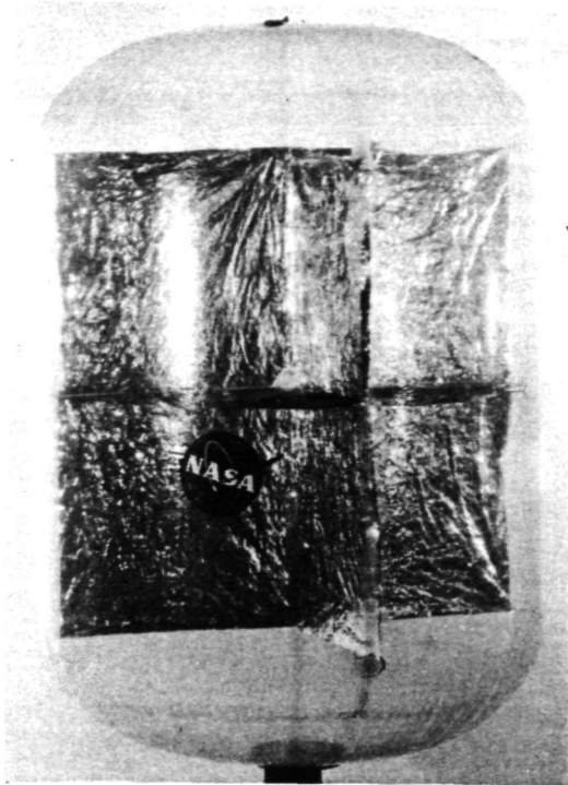
Fig. 5. Cylindrical balloon reflector (eight-corner reflector array) 91.4 cm diameter.
