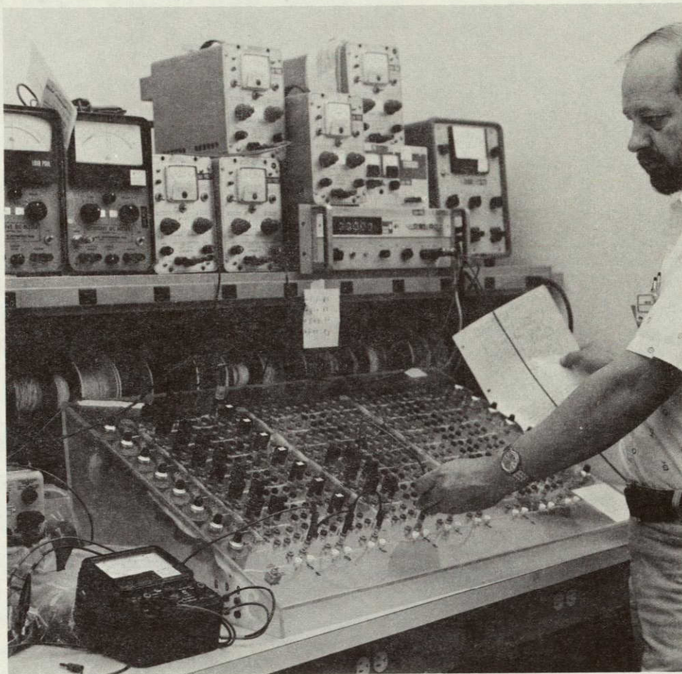
Fig. 5-2. Matrix Board Setup for Control of Bias During Irradiation and for Electrical Parameter Measurements in situ
