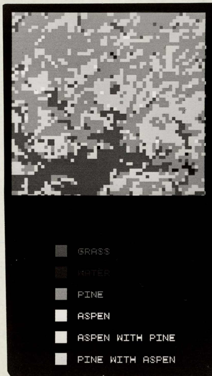
Figure 16. Sample black and white thematic map produced utilizing the Optronics film recorder system.
