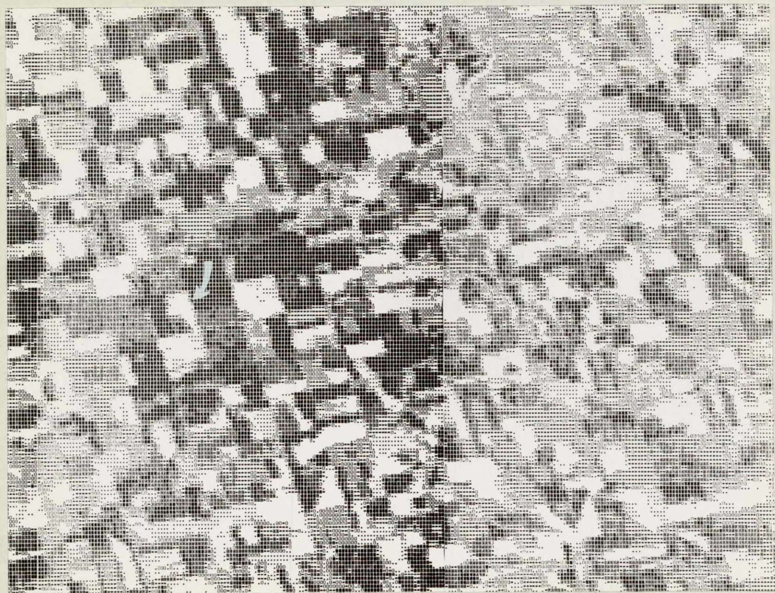
Fig. 12a. Computer overstrike printout from CCT encompassing intensive study area. Reduction is approximately one-third. (Arrow indicates common registration point with Fig. 12b). Variable overstrike darkness was caused by the printer ribbon.
