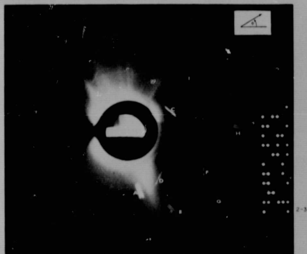
Fig. 5. A typical S052 photograph showing contamination tracks. The support boom obscures part of the field of view on the left side of the frame; the step wedge is inset in the center of the occulting disk. The matrix of white dots at the right are LEMs, which code the housekeeping data. The nine contamination tracks analyzed in this photograph are labeled A through I.
