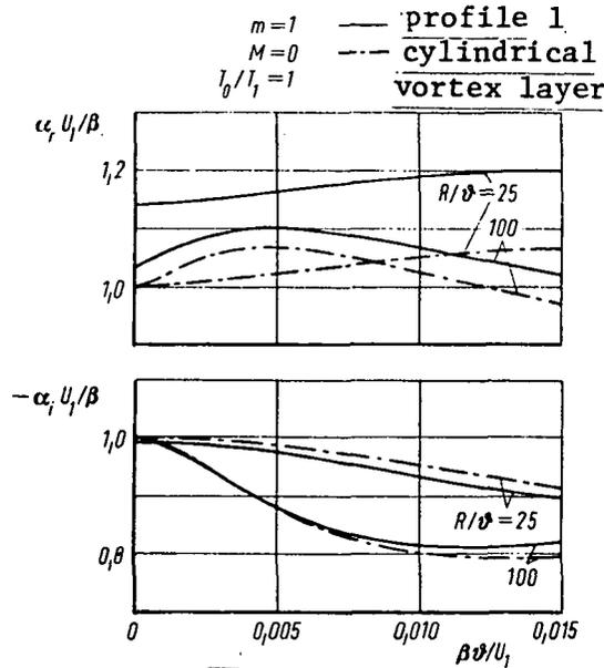
Figure 6: Comparison of eigenvalue  $\alpha_r$  and  $-\alpha_i$  of the first azimuthal perturbation for profile 1 with those of the cylindrical vortex layer  $R/\delta=100$  and 25 for small circular frequencies  $\beta(M = 0, T_0/T_1 = 1.)$
