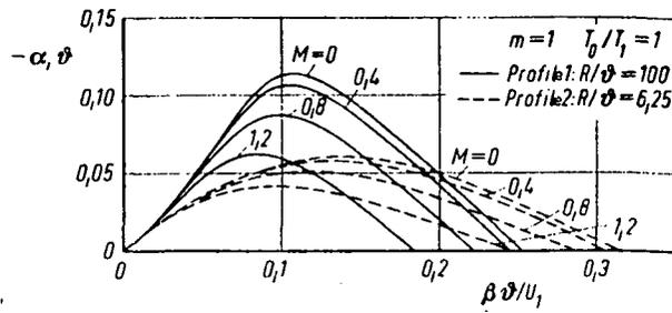
Figure 11: Buildup factor  $-\alpha_i$  of the first aximuthal perturbation as a function of circular frequency  $\beta$  for  $R/\phi = 100$  and  $6.25$  and various Mach numbers  $M$  ( $\gamma = 1.4$ ,  $T_o/T_i = 1$ )
