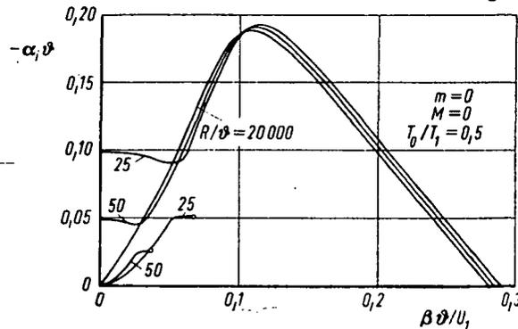
Figure 12: Buildup factor  $-\alpha_i$  of the axisymmetric perturbation as a function of circular frequency  $\beta$  for hot free jets ( $T_o/T_i = 0.5$ ) with various values of  $R/\phi$  ( $M=0$ ).
