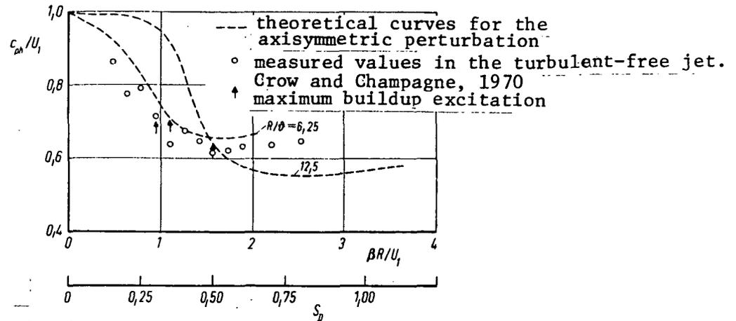
Figure 8: Measured phase velocity  $c_{ph}$  of the asymmetric perturbation in the turbulent free jet according to [44] as a function of the Strouhal number  $S_D$  compared with theoretical values for profile 2 and the free jet parameter values  $R/\delta = 12,5$  and  $6,25$  ( $M = 0$ ,  $T_0/T_1 = 1$ ).
