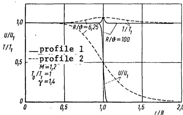
Figure 3: Velocity and temperature profiles in air ( $\gamma = 1.4$ ) for two values of the free jet parameter  $R/\theta$  for a Mach number  $M = 1.2$  and temperature ratio  $T_0/T_1 = 1$ .
