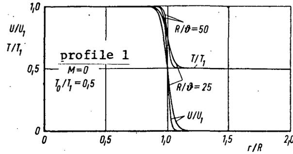
Figure 4: Velocity and temperature profiles for 2 values of the free jet parameter  $R/\theta$  for a Mach number  $M = 0$  and a temperature ratio of  $T_0/T_1 = 0.5$ .
