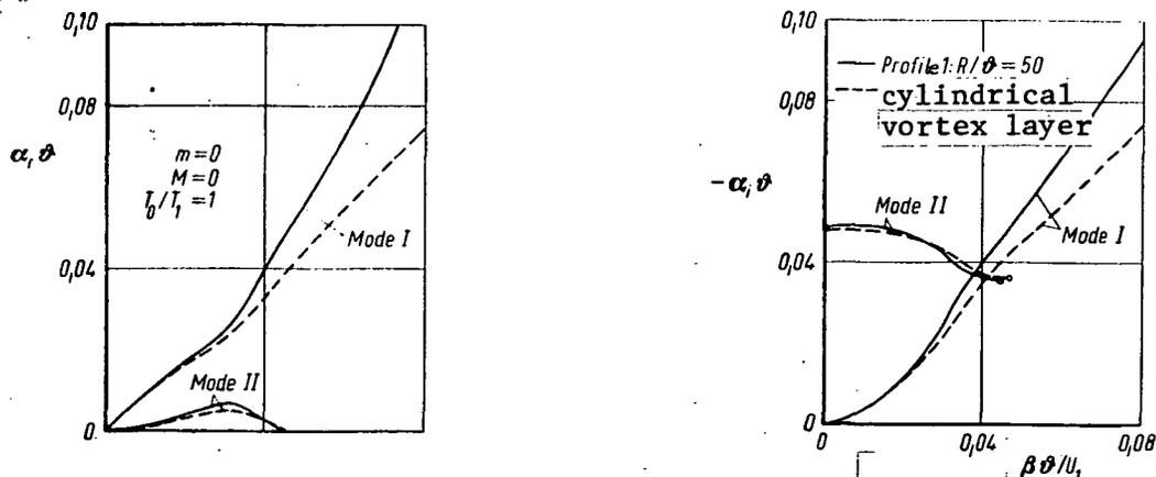
Figure 5: Comparison of eigenvalues  $\alpha_r$  and  $-\alpha_i$  of an axisymmetric perturbation for profile 1 with those of the cylindrical vortex layer at  $R/\delta = 50$  for small circular frequencies  $\beta$  ( $M = 0$ ,  $T_0/T_1 = 1$ )
