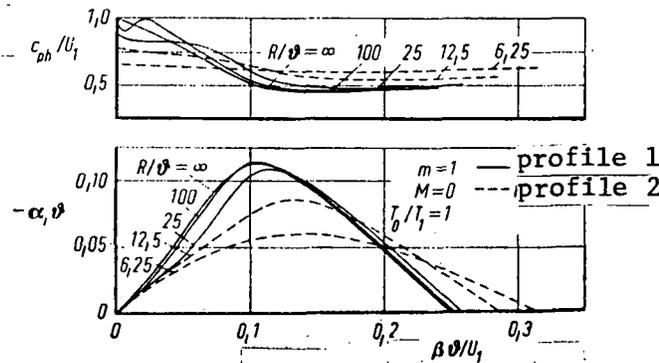
Figure 9: Phase velocity  $c_{ph}$  and buildup factor  $-\alpha_1$  of the first azimuthal perturbation as a function of circular frequency  $\beta$  for various free jet parameter values  $R/\delta$  ( $M = 0$ ,  $T_0/T_1 = 1$ )
