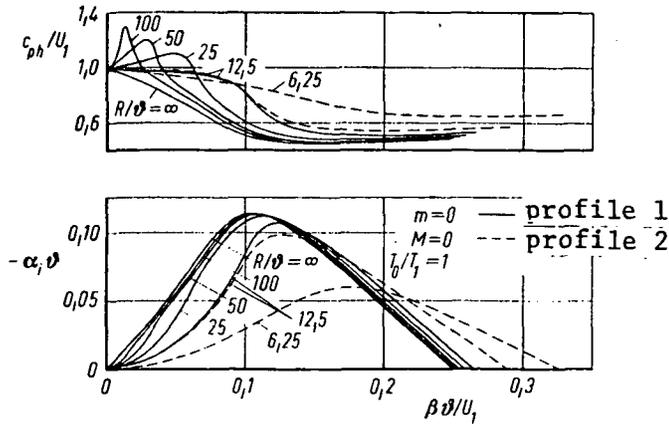
Figure 7: Phase velocity  $c_{ph}$  and buildup factor  $-\alpha_1$  of the asymmetric perturbation as a function of circular frequency  $\beta$  for various free jet parameter values  $R/\delta$  ( $M=0, T_0/T_1=1$ )
