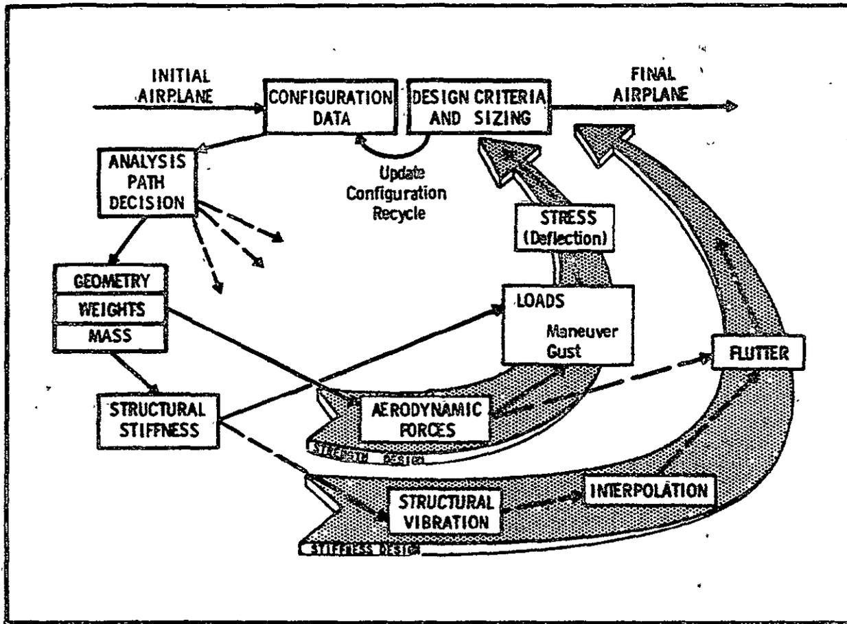
Figure 4.14 Boeing ATLAS System Aeroelastic Cycle
