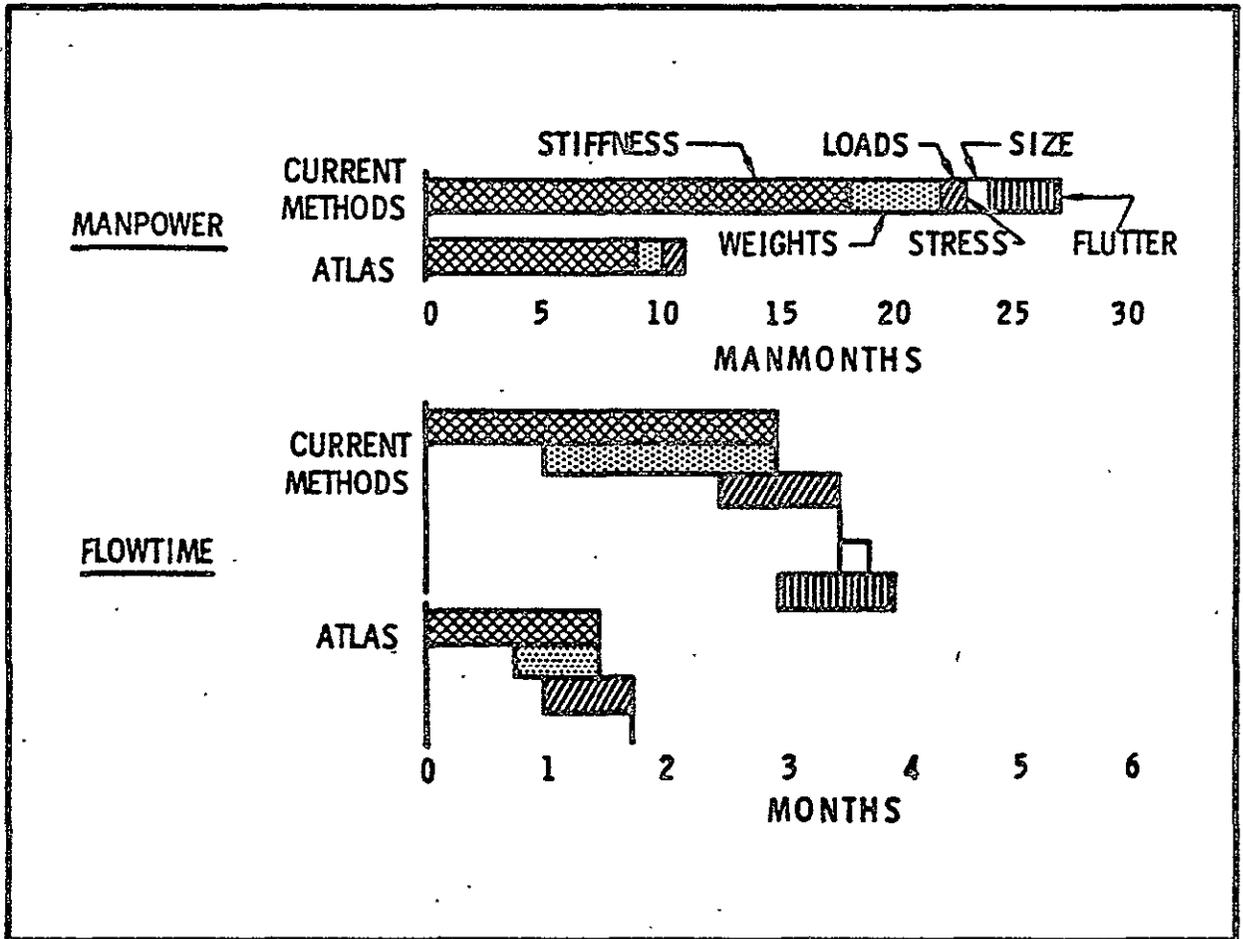
Figure 4.15 Boeing ATLAS System, Flowtime and Manpower Savings
