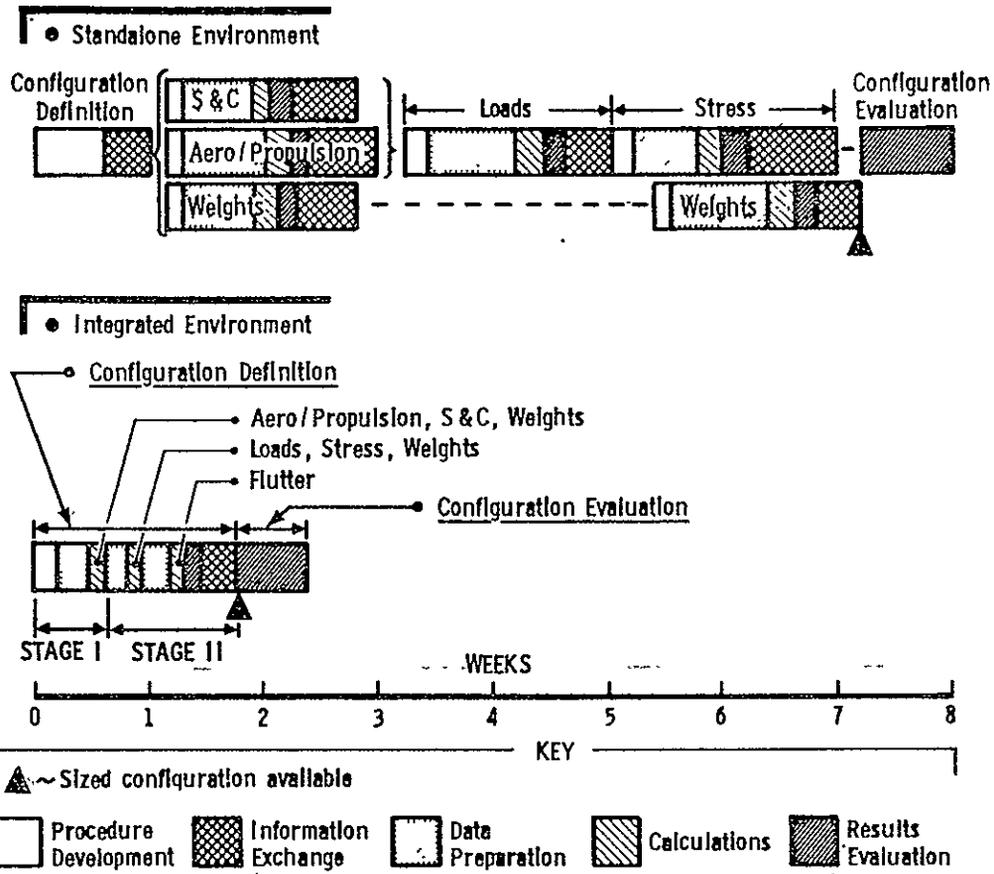
Figure 4.6 Level III, Subsonic Transport, Relative Flowtime, Standalone/Integrated Environment
