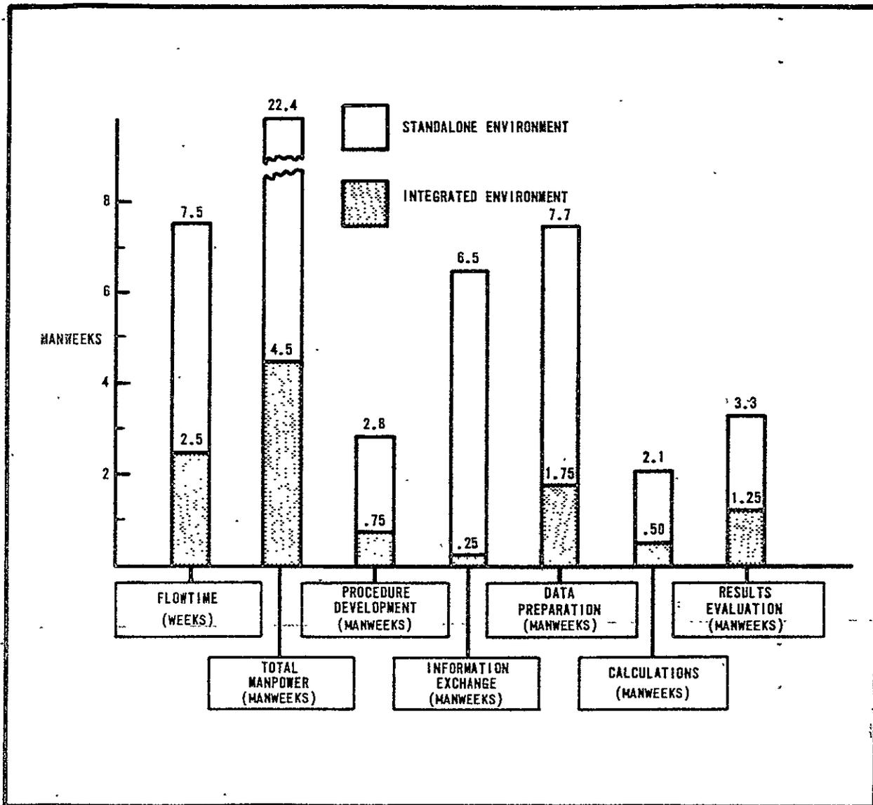
Figure 4.8 Level III, Subsonic Transport, Flowtime and Labor Comparison, Standalone/Integrated Environment
