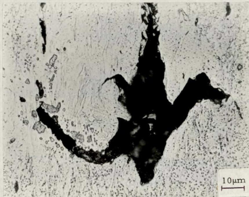
Figure 19 Optical micrograph of a sectioned tensile specimen of the 718 MN/m 2 (104 ksi) material strained to 1.550. The tensile axis is vertical.
