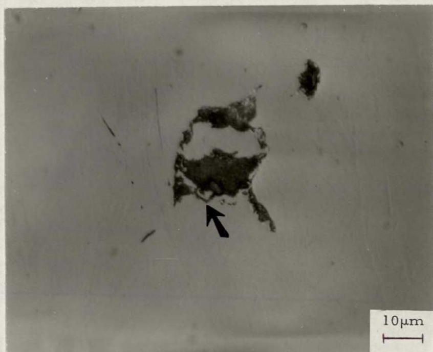
Figure 20 Optical micrograph of a sectioned tensile specimen of the 2070 MN/m 2 (300 ksi) material strained to 0.487. The Ti(C,N) inclusion nucleation site is marked by an arrow. The tensile axis is vertical.
