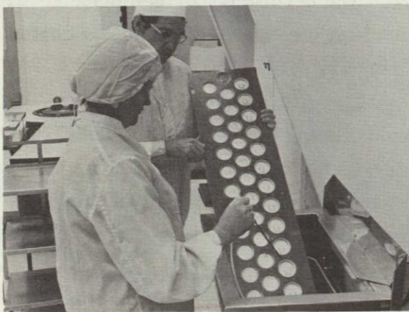
Figure 3.1.2-4 "P" Joint Cleaning
