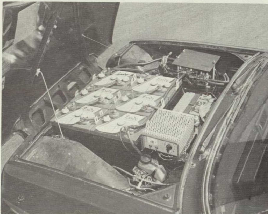
Figure 2. - View under hood of Waterman Renault, showing controller, charger, and front battery pack.
