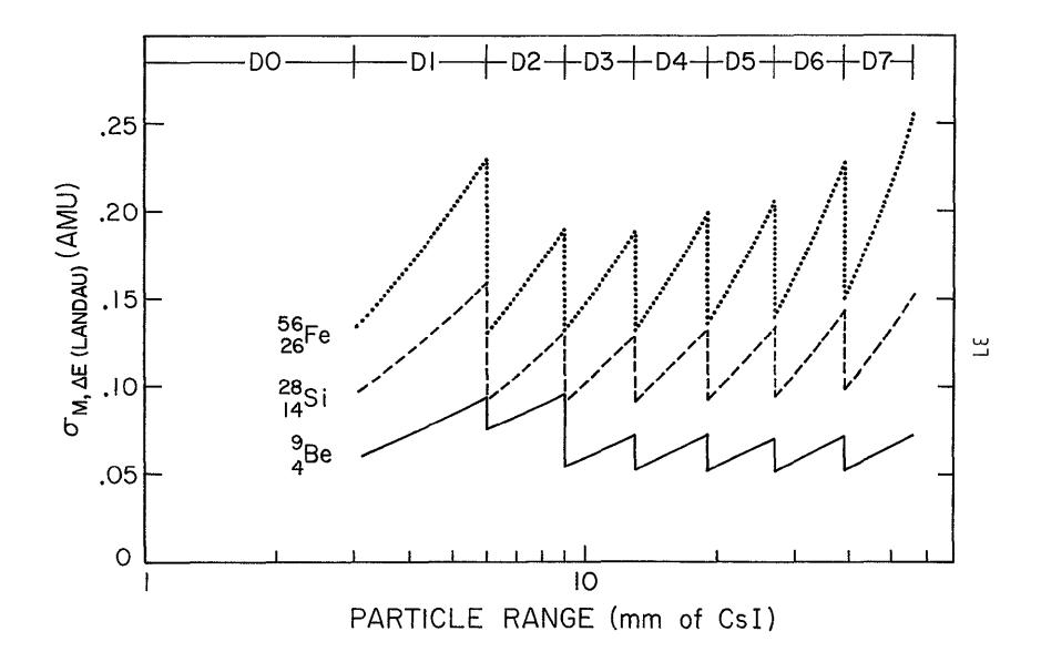
losses in D() through Dn-1 will be added to form the  $\Delta E$  measurement. The sawtooth pattern is primarily due to the variation of the L/R ratio as discussed above.
