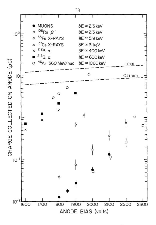
ORIGINAL PAGE IS OF POOR QUALITY avalanche is comparable to this static charge, a reduction in the gain of the chamber is expected since the charge in the electron cloud reduces the electric field seen by late arriving electrons.
