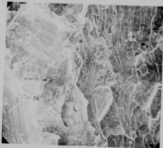
(b) Cleavage in Armco 18 SR (TRC) tested perpendicular to final rolling direction. Prior creep exposure 2.1MPa at 1273 K to 4.9 percent strain.
