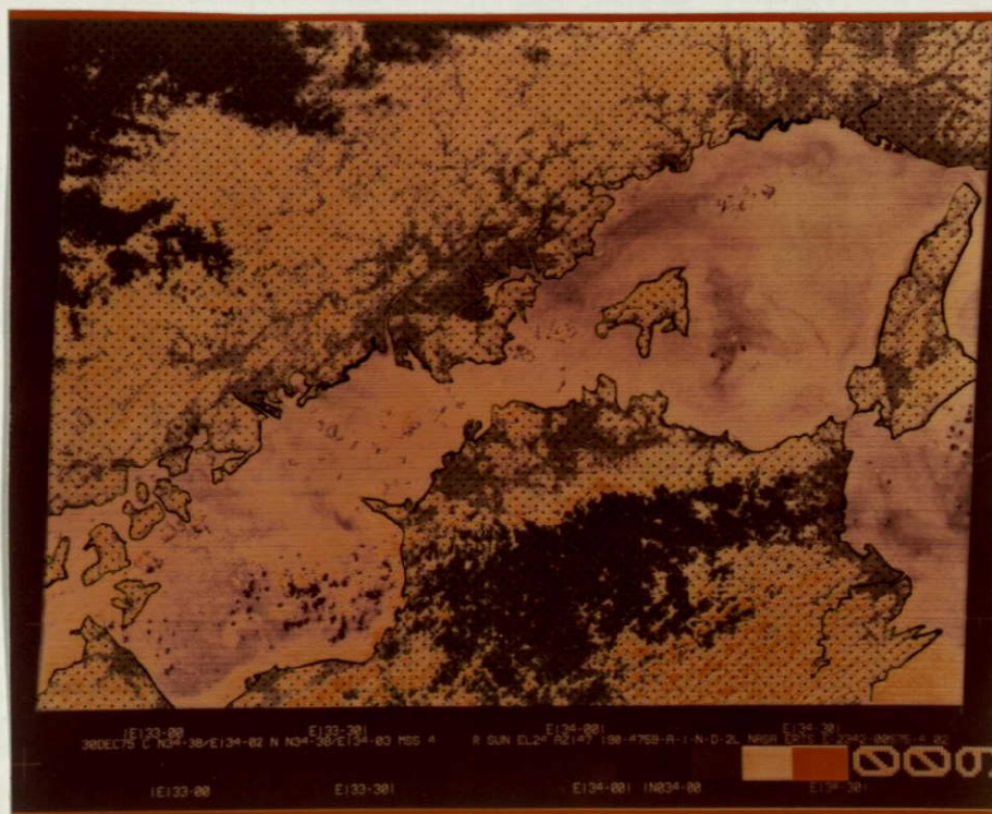
Fig.10 A color negative print made out of Band-4 of Landsat MSS image alone through manual photographic processing method. Dec. 30, 1975.
