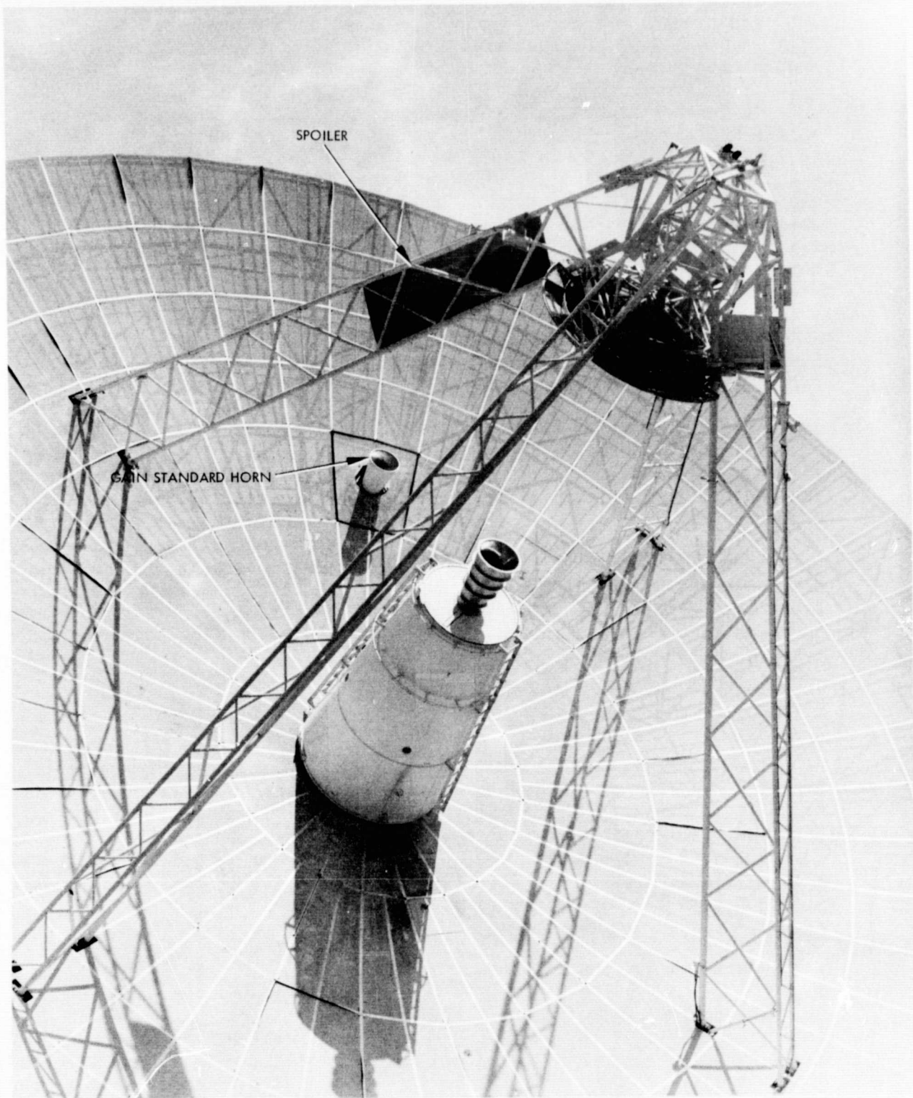
Fig. 3-6. Gain Standard Horn Mounted Within the 26-m Aperture (Oct. 1971)
