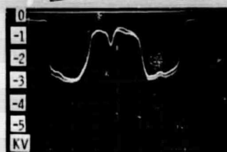
(a) Front surface potential profile, 5 KeV beam, minutes 20 and 27, 1 KV/division.
