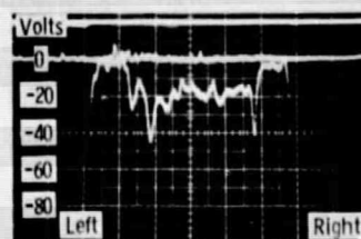
Figure 9. - Typical surface potential profiles of sample # 3.
