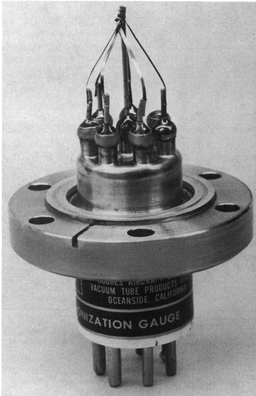
Figure 5.- Krypton desorption assembly.
