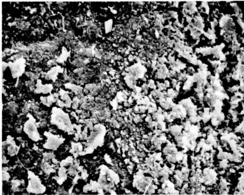
Figure 5 - Alumina impregnated RSSN surface after firing in A + SiO atmosphere for three hours at 1400°C, SEM, 2000X.
