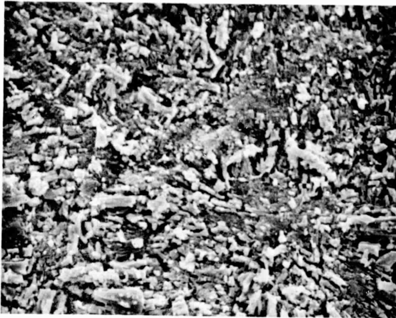
Figure 7 - Zirconia impregnated RSSN surface after firing in A + SiO atmosphere for three hours at 1400°C, SEM, 2000X.
