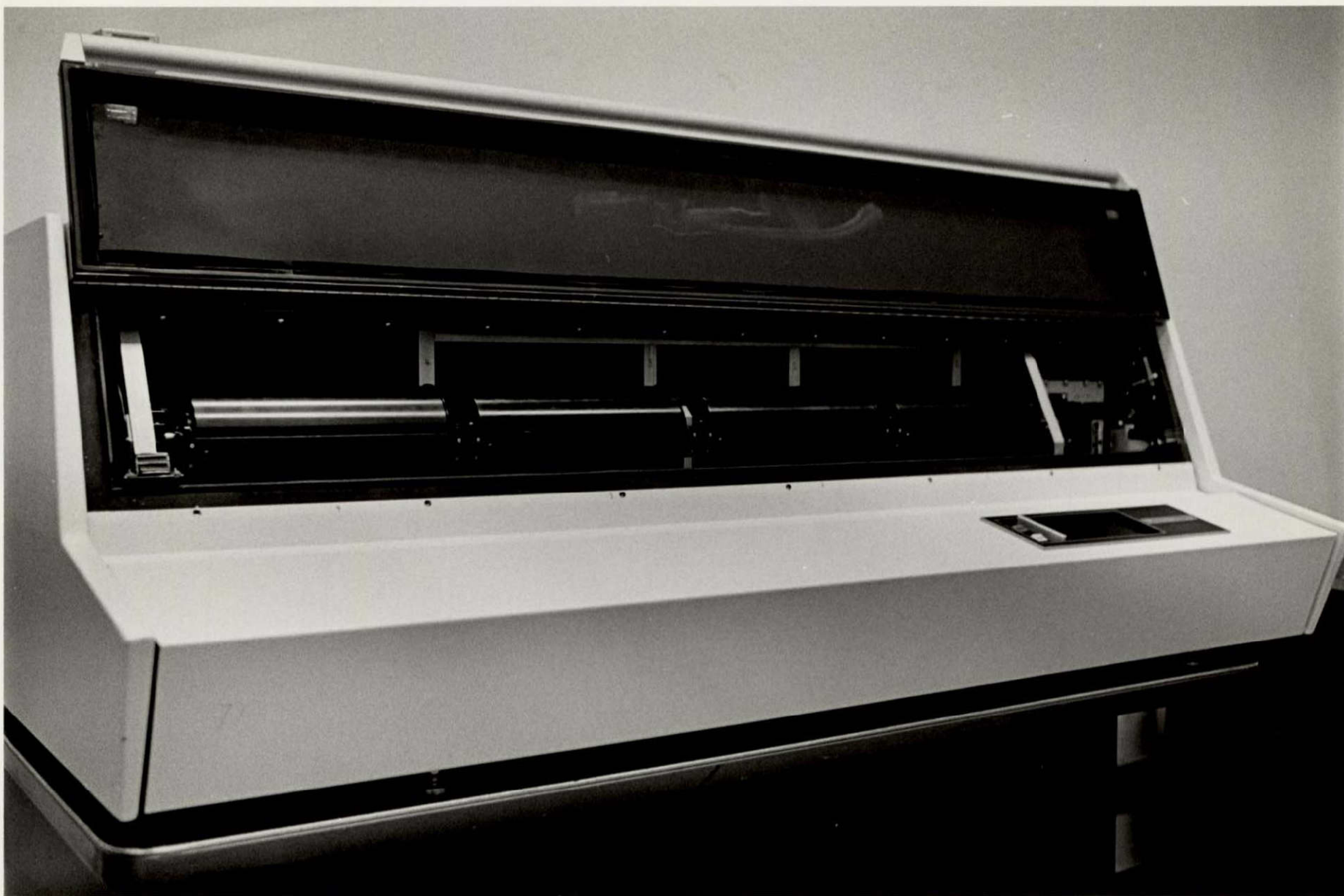
Figure 2 High resolution digital image recorder used at the Geophysical Institute to make film products from Landsat digital data.
