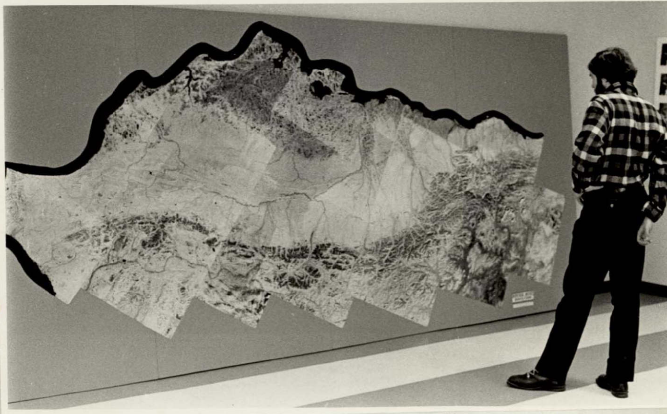
Figure 17 Alaska North Slope Mosaic Photographer Mal Lockwood (above) puts finishing touches on the 1:250,000 scale Landsat mosaic produced for the North Slope Borough. The completed mosaic, (below) measuring 16 feet across, now resides in Barrow, Alaska, and is used for planning by Borough officials.
