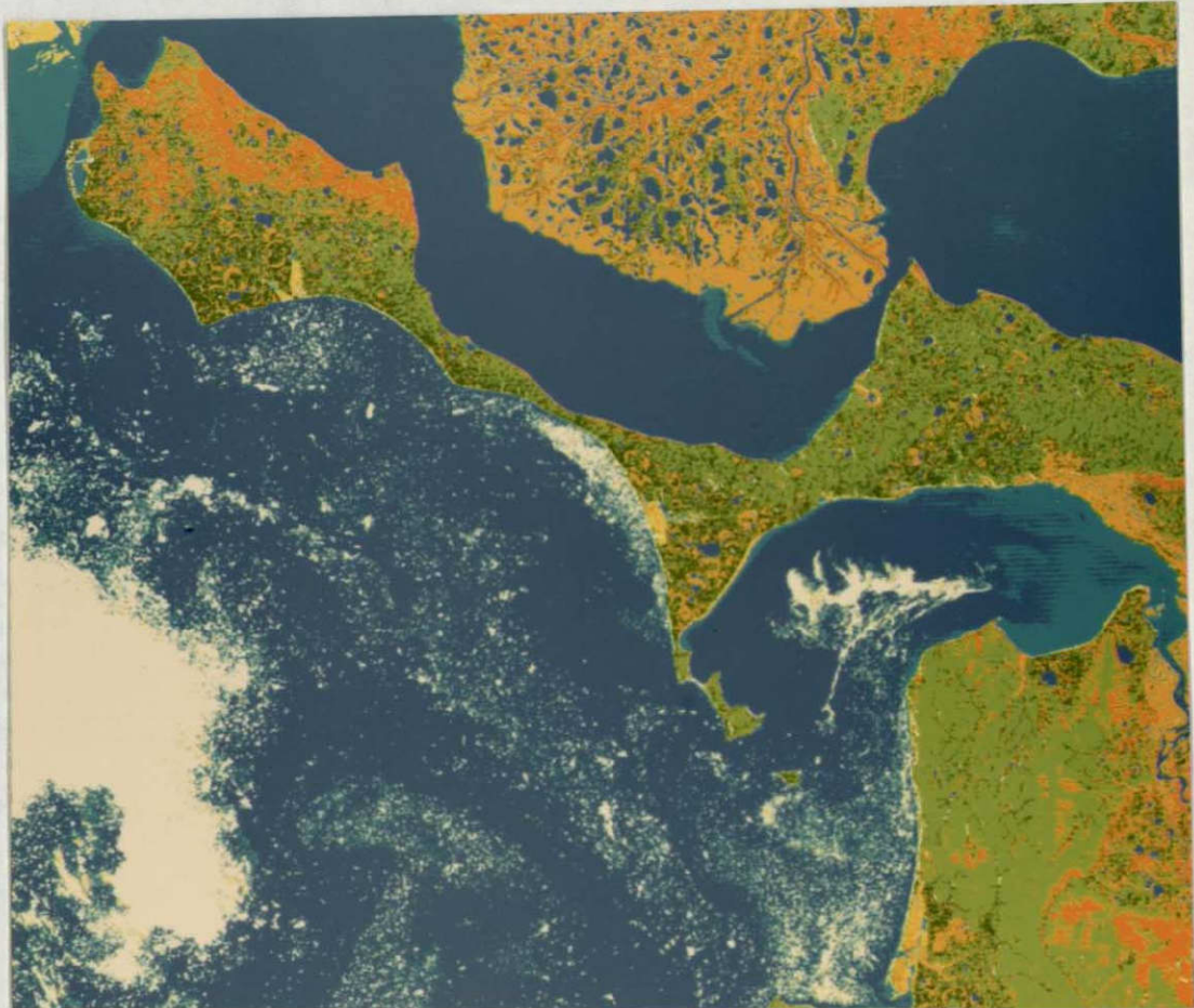
Figure 3 Color-coded thematic image of the Baldwin Peninsula, N.W. Alaska, produced from digital Landsat data on IGOR, a high resolution digital-image recorder.
