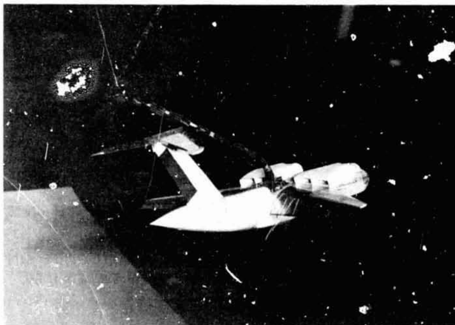
Figure 22.- Photograph of four-engine swept-wing free-flight USB model in the Langley full-scale tunnel.
