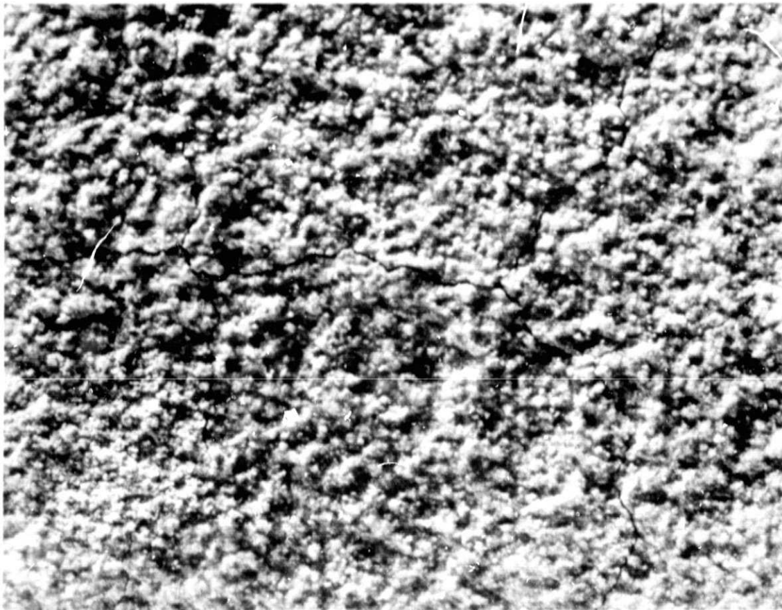
Figure 33 Radial (Mud Flat) Cracks – Thermal Fatigue Test No. 1 Baseline Seal System (77-441-0995-L)
