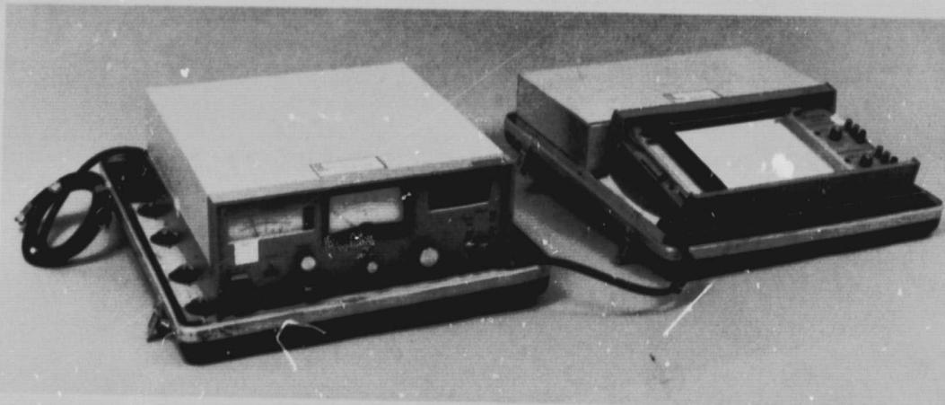
**Fig. 3. Scientific Atlanta Fault Locator Model 1691 and Recorder**
