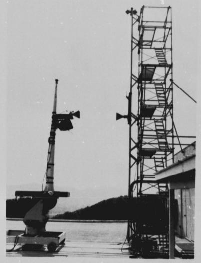
Fig. 2. Test Setup at JPL Antenna Range Facility. Horns are 152.4 cm (5 ft) apart
