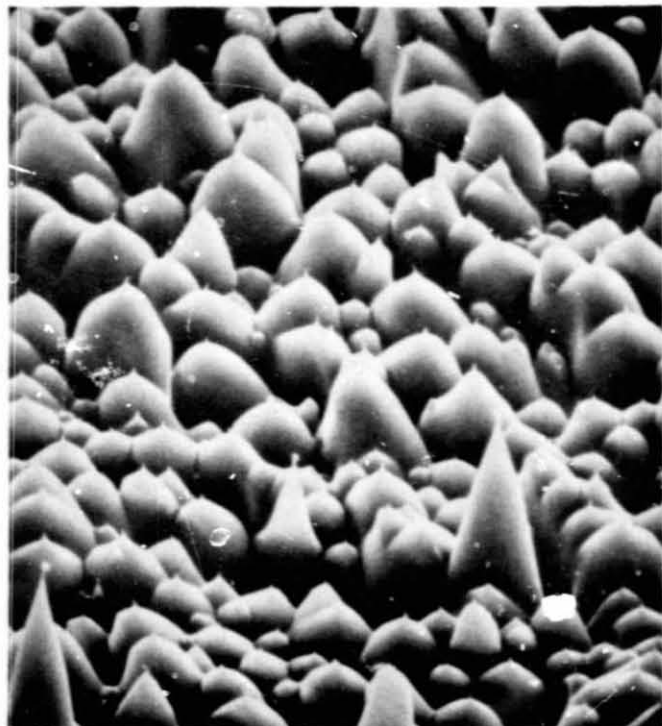
(b) FEP SPUTTER ETCHED 0.5 HOUR BY 750 eV ARGON IONS AT 0.6 mA/cm 2 .
