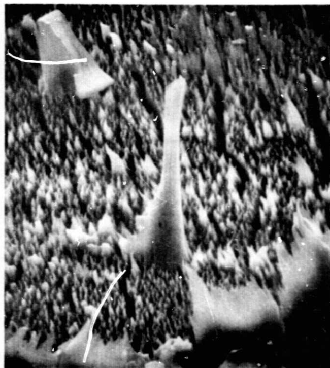
(d) PFA TEFLON R SPUTTER ETCHED 1.2 HOURS BY 750 eV ARGON IONS AT 0.3 mA/cm 2 .
